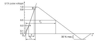
Front time:  $T_1 = 1.67 \text{ x T} = 1.2 \text{ } \mu\text{s} \pm 30 \text{ } \%$ Time to half-value:  $T_2 = 50 \text{ } \mu\text{s} \pm 20 \text{ } \%$
