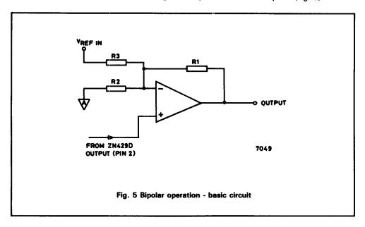
When the digital input of the ZN429 is zero the analogue output is zero and the amplifier output should be - full-scale. An input of all ones to the D-A will give a ZN429 output of  ${}_{\rm LN}$  and the amplifier output required is + full-scale. Also, to match the ladder resistance, the parallel combination of R1, R2 and R3 should be  $10 k\Omega$ .
