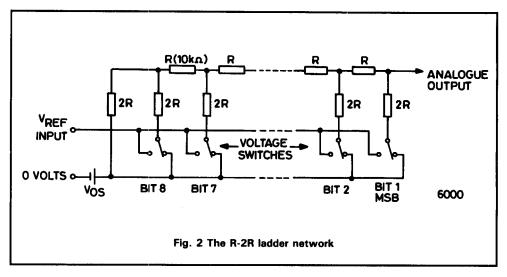
Each 2R element is connected either to 0V or  $V_{REF}$  by transistor switches specially designed for low offset voltage (typically 1mV).
