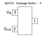
(Top View) Pin 1 floating or connected to pin 2
