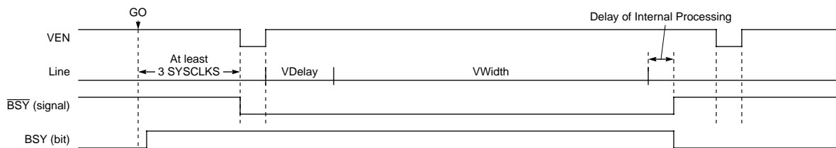
Figure 10. Relationship of BSY Terminal and BSY Flag and GO Bit
