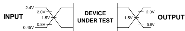
During AC testing, inputs are driven at 0.4V and 2.4V levels. Unless otherwise specified, switching times are measured from the 1.5V level of DCLK to the 0.8V or 2.0V levels at the input/output.
