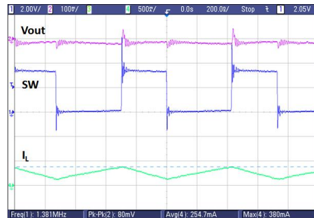
Dynamic loading operation ( I_L = 100 \sim 200mA )
