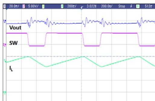
Heavy Loading Operation ( $I_L = 800\text{mA}$ )
