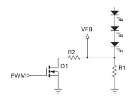
$$MOSFET 'off' \\ I_{LED(MIN)} = \frac{V_{FB}}{R_{LED}}$$
