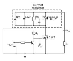
Gate charge test circuit
