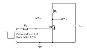
Switching time test circuit
