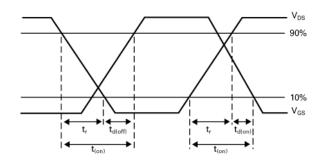
Switching time waveforms
