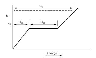
Basic gate charge waveform
