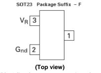
Pin 1 floating or connected to pin 2
