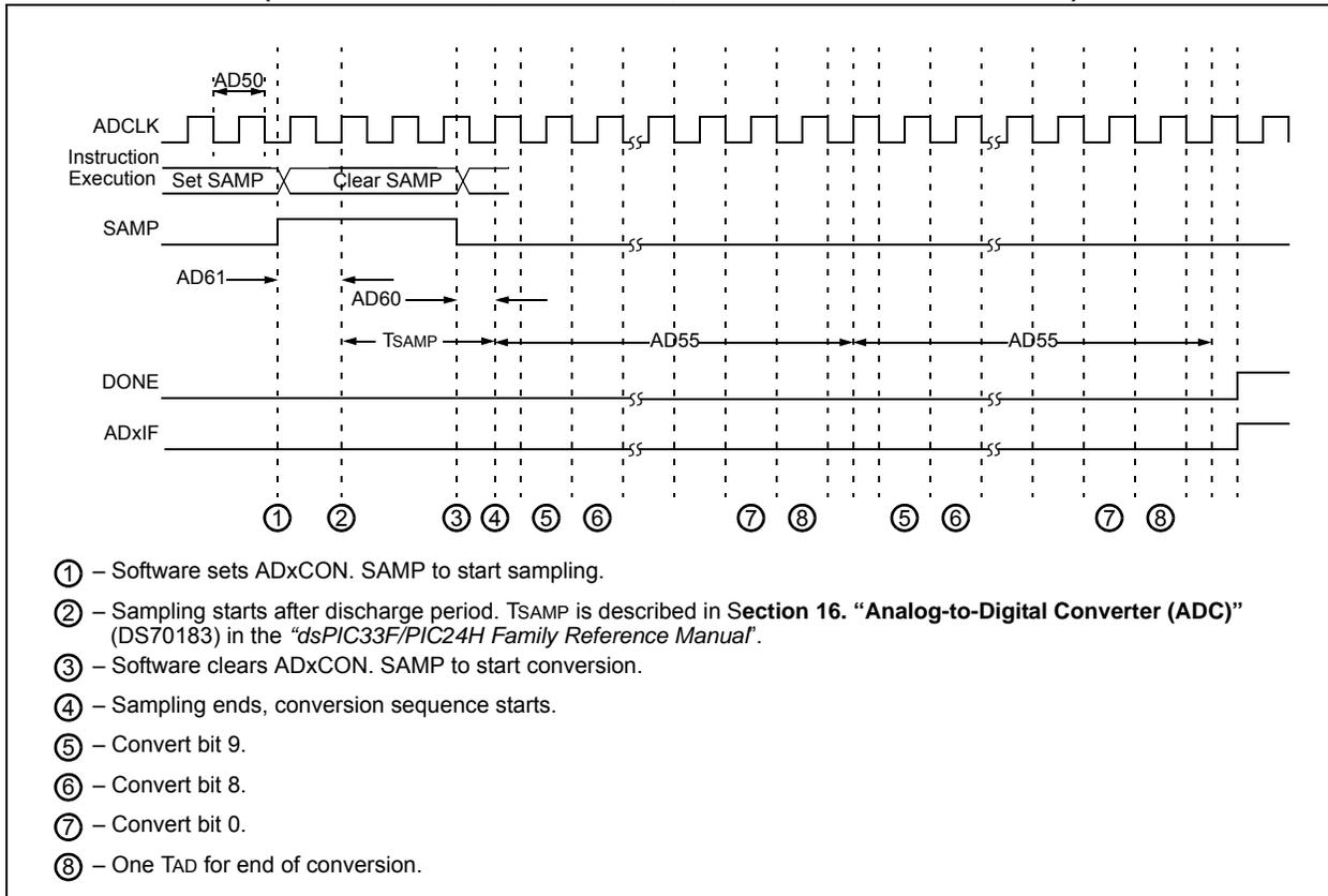
**FIGURE 24-28: ADC CONVERSION (10-BIT MODE) TIMING CHARACTERISTICS (CHPS<1:0> = 01, SIMSAM = 0, ASAM = 1, SSRC<2:0> = 111, SAMC<4:0> = 00001)**
