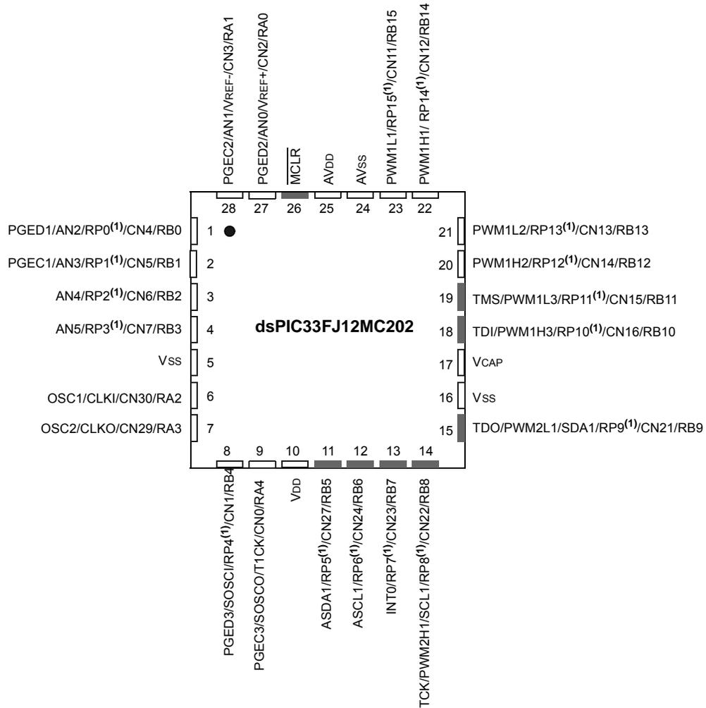
**Note 1:** The RPN pins can be used by any remappable peripheral. See [Table 1](#) for the list of available peripherals.
