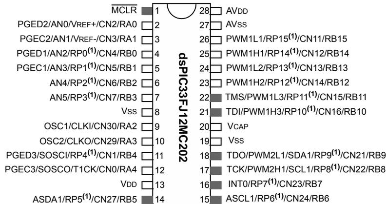
**Note 1:** The RPn pins can be used by any remappable peripheral. See [Table 1](#) for the list of available peripherals.
