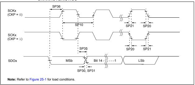
TABLE 25-29: SPIx MASTER MODE (HALF-DUPLEX, TRANSMIT ONLY) TIMING REQUIREMENTS
