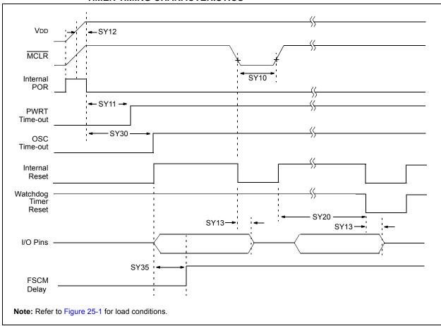
TABLE 25-21: RESET, WATCHDOG TIMER, OSCILLATOR START-UP TIMER, POWER-UP TIMER TIMING REQUIREMENTS
