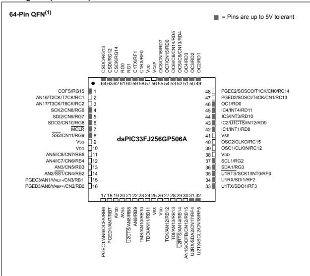
**Note 1:** The metal plane at the bottom of the device is not connected to any pins and should be connected to Vss externally.
