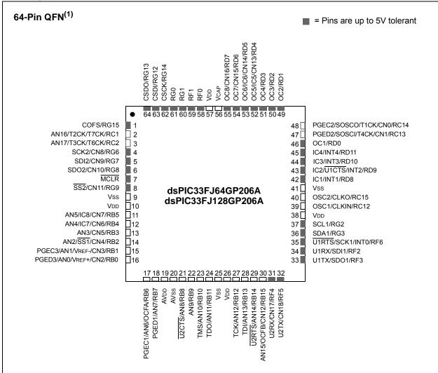
**Note 1:** The metal plane at the bottom of the device is not connected to any pins and should be connected to Vss externally.
