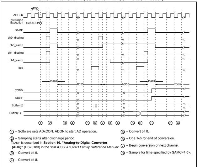
TABLE 25-45: ADC CONVERSION (10-BIT MODE) TIMING REQUIREMENTS
