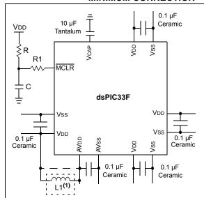
Note 1: As an option, instead of a hard-wired connection, an inductor (L1) can be substituted between VDD and AVDD to improve ADC noise rejection. The inductor impedance should be less than  $1\Omega$  and the inductor capacity greater than 10 mA.
