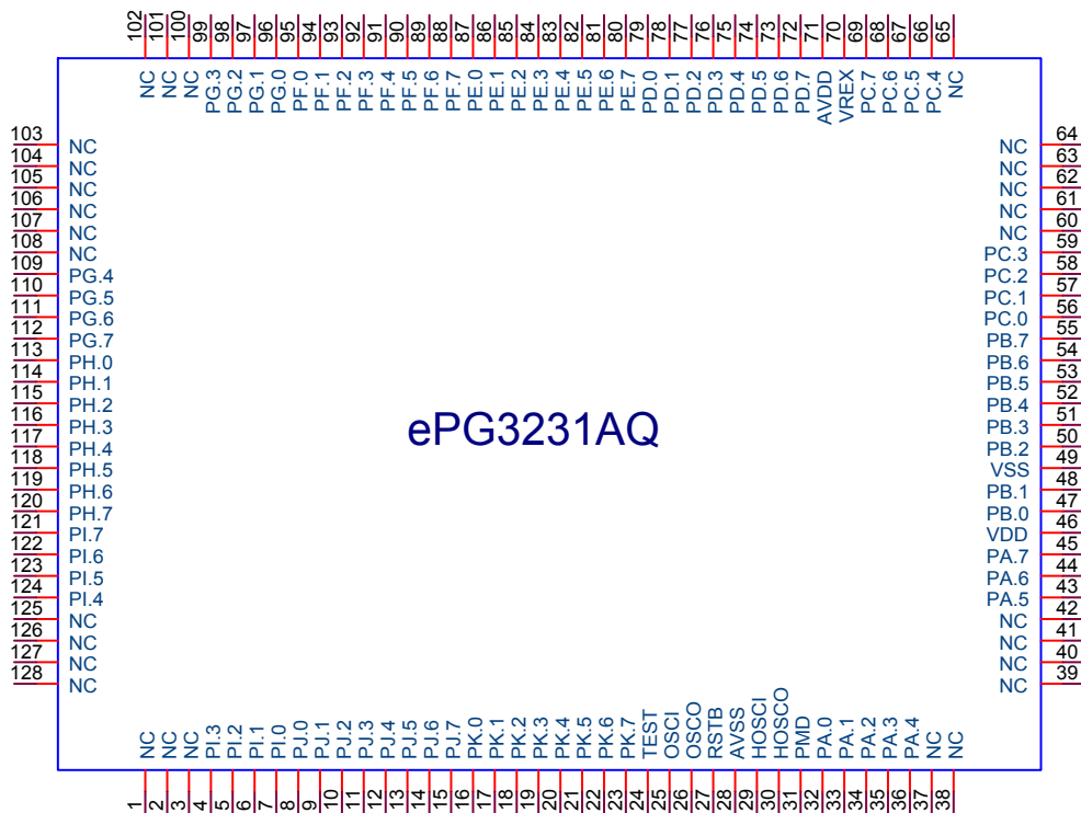
Fig. 4-1 ePG3231 Package: QFP 128 Pins
