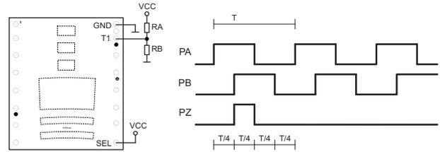
Figure 12: AB-gated index (T1 = open or VCC/2),
