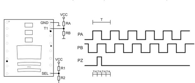
Figure 15: AB-gated index (T1 = open or VCC/2)
