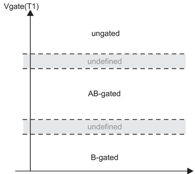
Figure 3: Index gating selection at pin T1.
