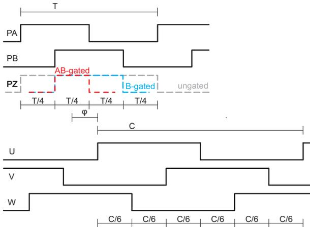
Figure 4: Encoder quadrature signals and motor commutation signals.
