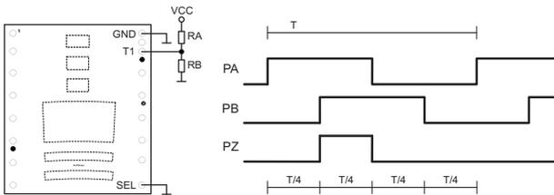
Figure 9: AB-gated index (T1 = open or VCC/2),
