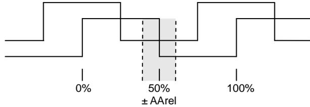
Figure 1: Definition of AB duty cycle variation.
