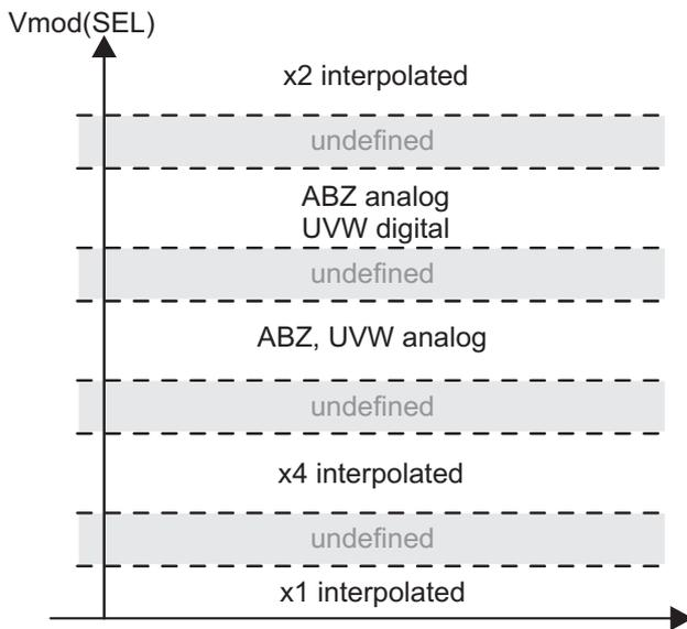
Figure 2: Operating mode selection at pin SEL.
