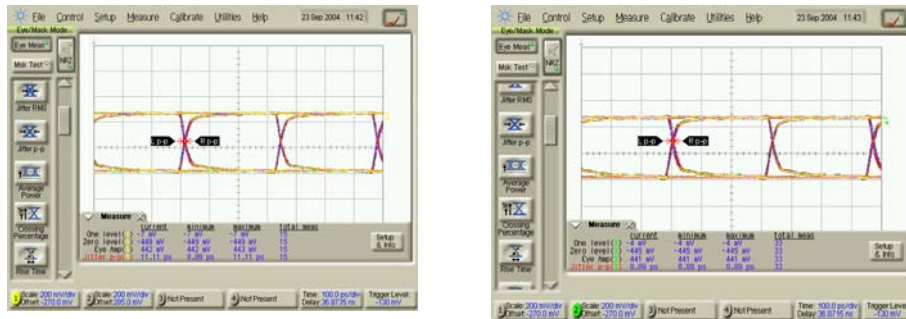
Die measurements (OUT and OUT/) VDD: +2.5 V, Vee: -3.3 V Input data rate: 3 Gb/s Differential data input (1.1 V/0.6 V) With two separated 50-ohms to ground termination, DC-coupled output
