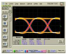
Input amplitude = 400 mV Output amplitude ≈ 5.0 V
