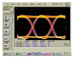
Input amplitude = 400 mV, Output amplitude ≈ 7.0 V
