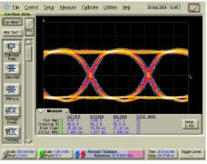
Input amplitude = 400 mV Output amplitude ≈ 3.5V
