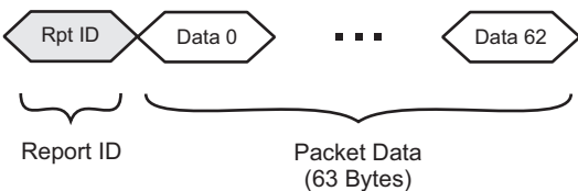
FIGURE 10-2: GENERIC HID – DATA PACKET FORMAT
