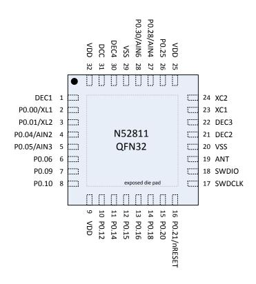
Figure 152: QFN32 pin assignments, top view
