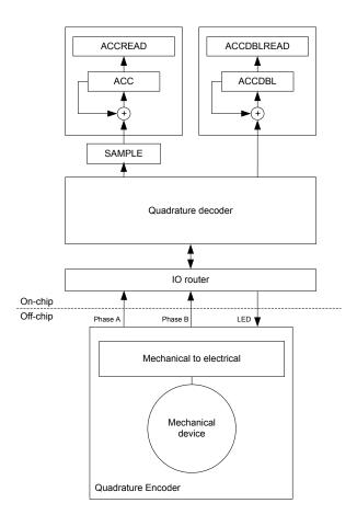
Figure 56: Quadrature decoder configuration
