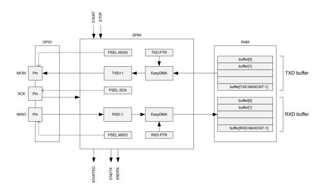
Figure 115: SPIM — SPI master with EasyDMA
