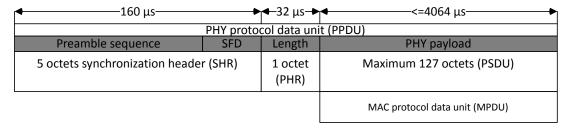
Figure 77: IEEE 802.15.4 frame format (PPDU)
