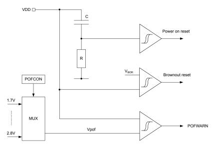
Figure 15: Power supply supervisor
