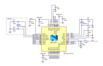
Figure 159: QCAA QFN32 with internal LDO regulator setup
