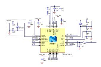
Figure 160: QCAA QFN32 with DC/DC regulator setup
