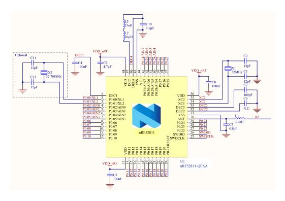
Figure 158: QFAA QFN48 with DC/DC regulator setup
