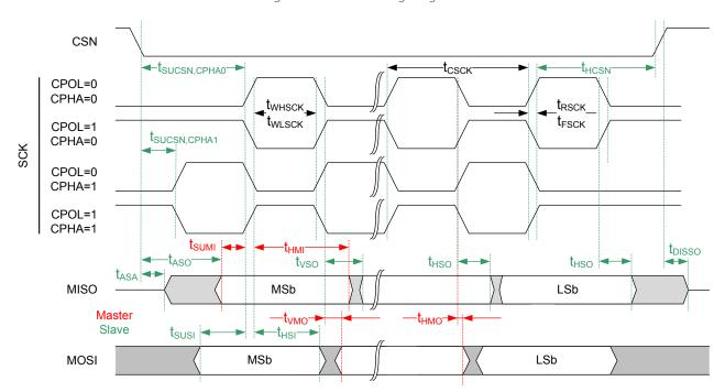
Figure 121: Common SPIM and SPIS timing diagram
