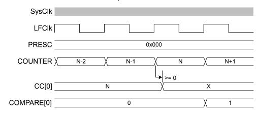
Figure 98: Timing diagram - COMPARE\_N-1
