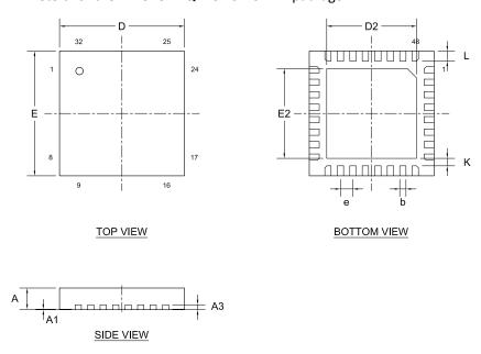
Figure 155: QFN32 5 x 5 mm package
