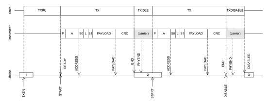
Figure 65: Transmission of multiple packets
