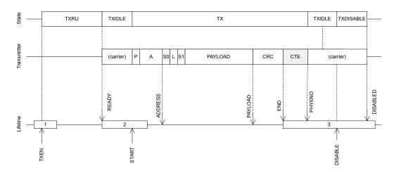
Figure 75: Transmit sequence with DFE
