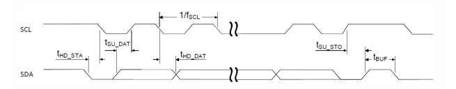
Figure 127: TWI timing diagram, 1 byte transaction
