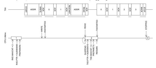
Figure 142: A repeated start sequence, where the TWI master writes two bytes followed by reading four bytes from the slave
