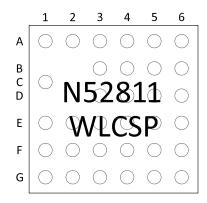
Figure 153: WLCSP ball assignments, top view
