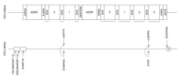
Figure 133: A repeated start sequence, where the TWI master writes two bytes followed by reading 4 bytes from the slave
