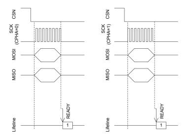
Figure 113: SPI master transaction
