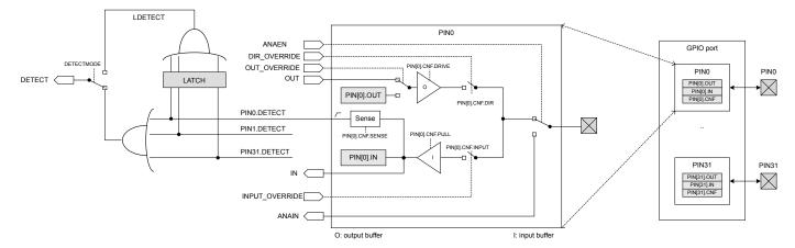
Figure 39: GPIO port and the GPIO pin details
