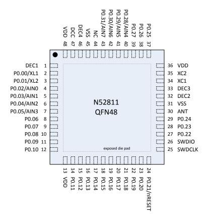
Figure 151: QFN48 pin assignments, top view
