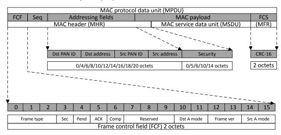
Figure 78: IEEE 802.15.4 frame format (MPDU)
