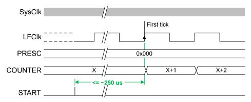
Figure 102: Timing diagram - JITTER START+
