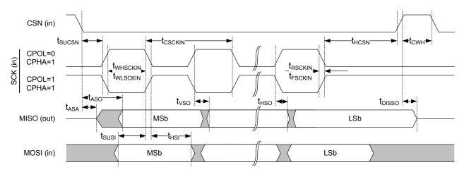
Figure 120: SPIS timing diagram
