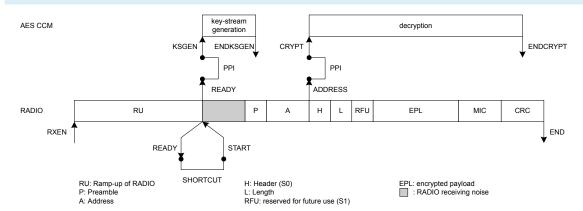
Figure 32: On-the-fly decryption of short packets (MODE.LENGTH = Default) using a PPI connection
