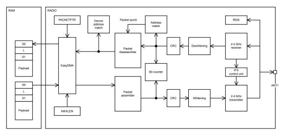
Figure 57: RADIO block diagram
