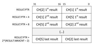
Figure 105: Example of RAM placement (even RESULT.MAXCNT), channels 1, 2 and 5 enabled
