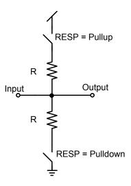
Figure 108: Resistor ladder for positive input (negative input is equivalent, using RESN instead of RESP)
