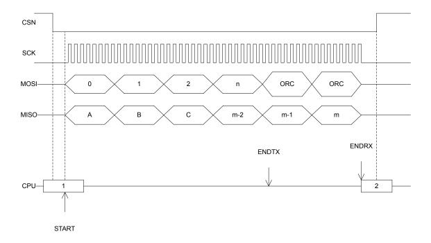
Figure 116: SPI master transaction
