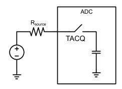
Figure 109: Simplified ADC sample network
