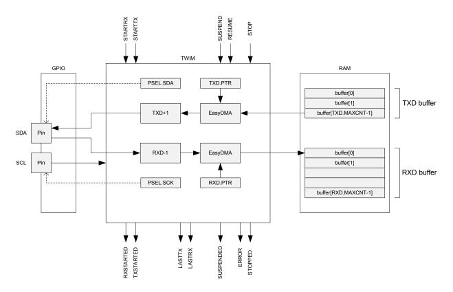
Figure 129: TWI master with EasyDMA
