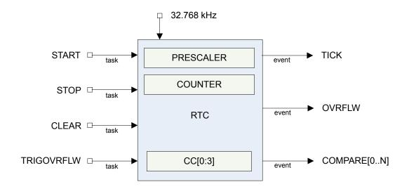
Figure 89: RTC block schematic
