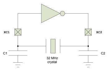
Figure 18: Circuit diagram of the 64 MHz crystal oscillator
