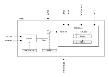
Figure 128: Block schematic for timer/counter
