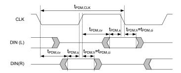
Figure 45: PDM timing diagram
