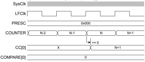
Figure 97: Timing diagram - COMPARE N+1
