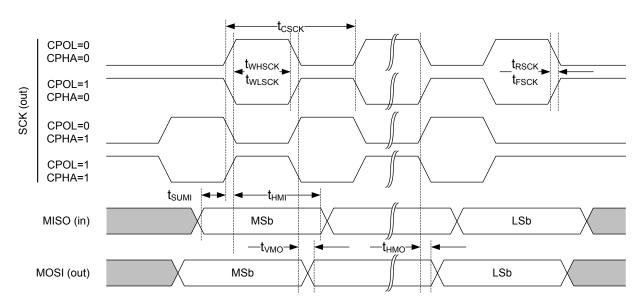
Figure 117: SPIM timing diagram
