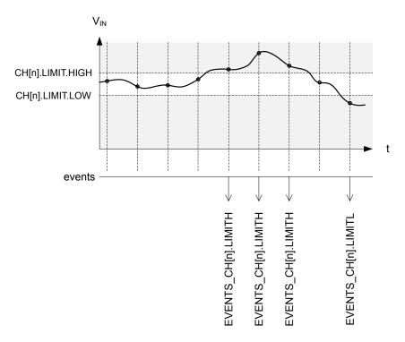
Figure 110: Example of limits monitoring on channel 'n'
