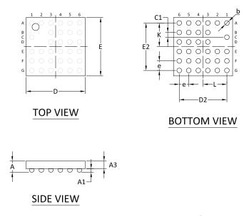
Figure 156: WLCSP 2.482 x 2.464 mm package
