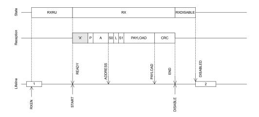
Figure 67: Receive sequence using shortcuts to avoid delays
