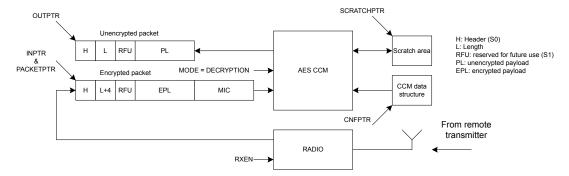
Figure 31: Configuration of on-the-fly decryption
