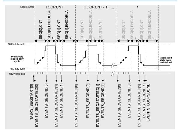
Figure 54: Complex sequence (LOOP.CNT>0) starting with SEQ[0]
