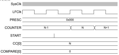
Figure 94: Timing diagram - COMPARE START
