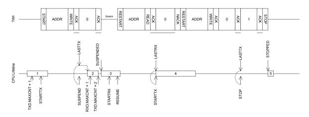
Figure 134: A double repeated start sequence using the SUSPEND task to secure safe operation in low priority interrupts
