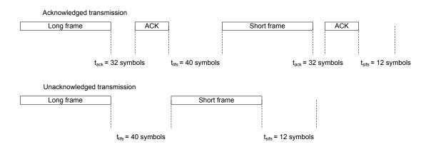
Figure 84: Interframe spacing examples
