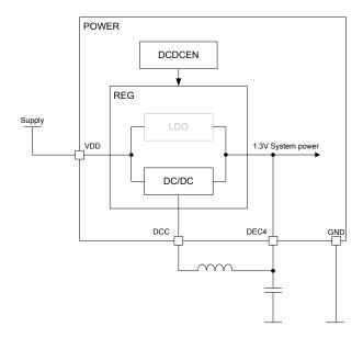
Figure 14: DC/DC regulator setup
