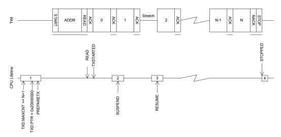
Figure 140: The TWI slave responding to a read command
