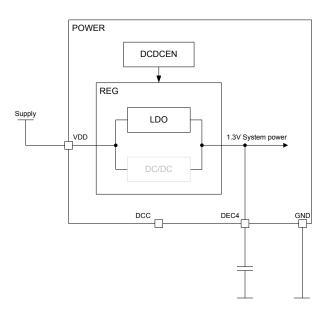
Figure 13: LDO regulator setup
