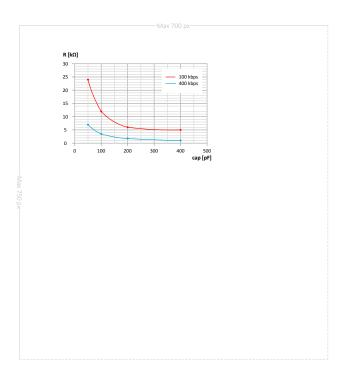
Figure 136: Recommended TWIM pullup value vs. line capacitance
