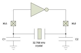
Figure 20: Circuit diagram of the 32.768 kHz crystal oscillator
