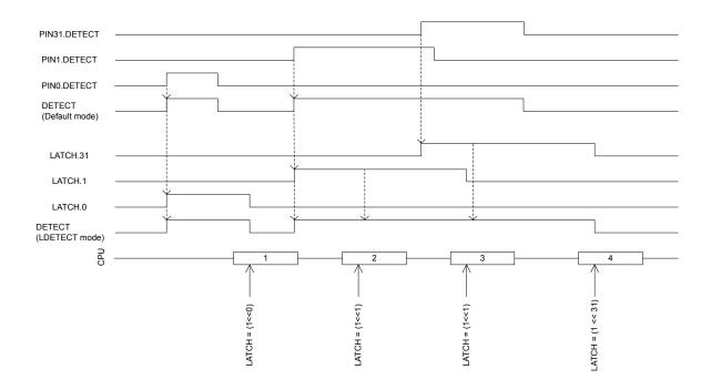
Figure 40: DETECT signal behavior
