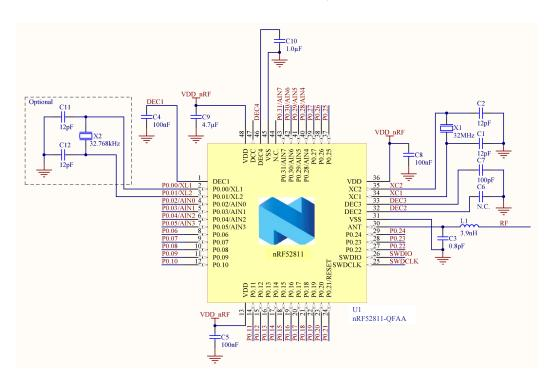
Figure 157: QFAA QFN48 with internal LDO regulator setup
