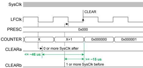
Figure 99: Timing diagram - DELAY\_CLEAR
