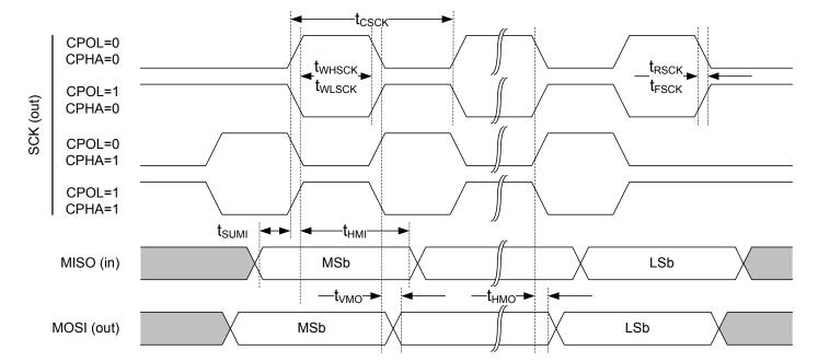
Figure 114: SPI master timing diagram
