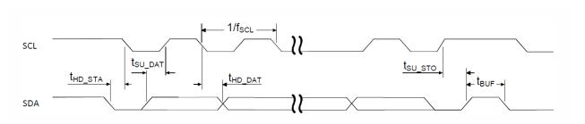
Figure 135: TWIM timing diagram, 1 byte transaction
