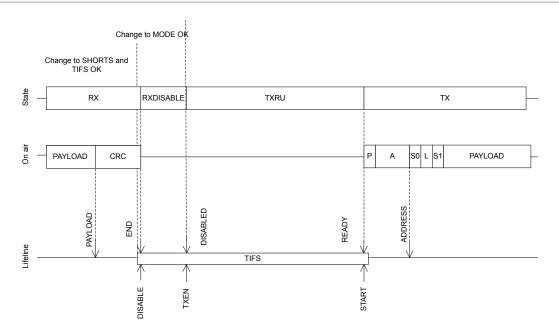
Figure 69: IFS timing detail
