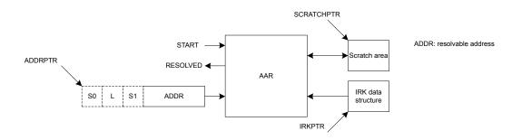
Figure 23: Address resolution with packet preloaded into RAM
