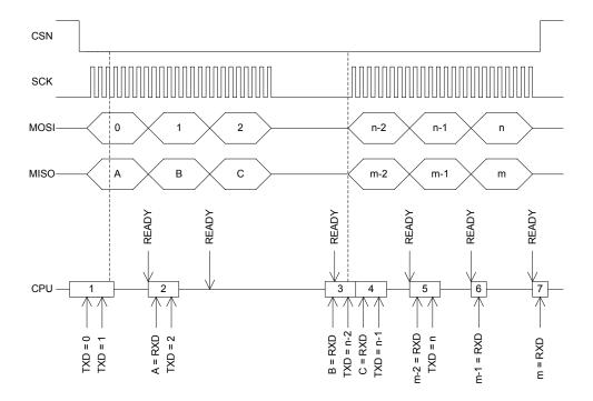
Figure 112: SPI master transaction
