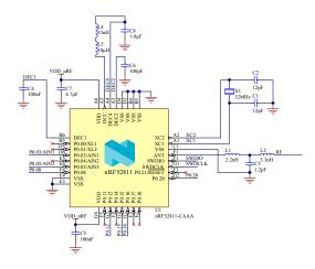
Figure 163: CAAA WLCSP 2-layer setup
