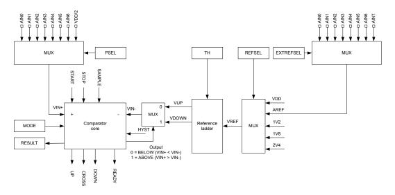
Figure 36: Comparator in single-ended mode
