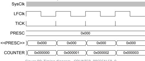
Figure 90: Timing diagram - COUNTER PRESCALER 0
