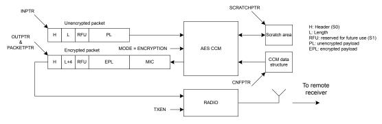
Figure 29: Configuration of on-the-fly encryption
