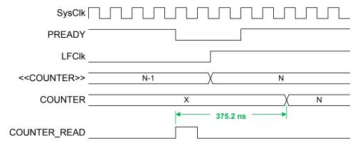
Figure 103: Timing diagram - COUNTER\_READ
