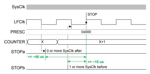
Figure 100: Timing diagram - DELAY\_STOP
