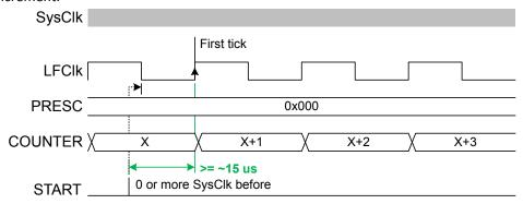
Figure 101: Timing diagram - JITTER START-
