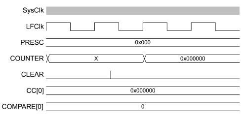
Figure 93: Timing diagram - COMPARE\_CLEAR
