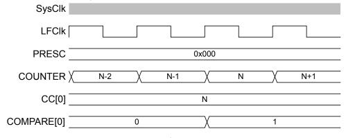
Figure 95: Timing diagram - COMPARE
