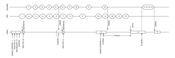
Figure 150: UARTE reception with forced stop via STOPRX
