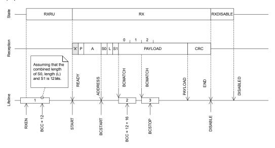
Figure 70: Bit counter example
