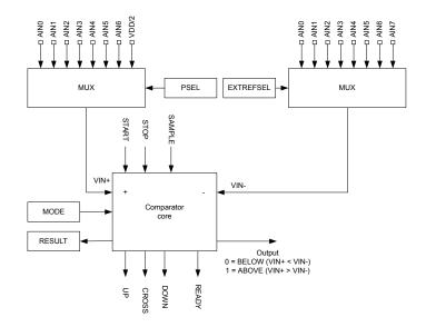
Figure 34: Comparator in differential mode
