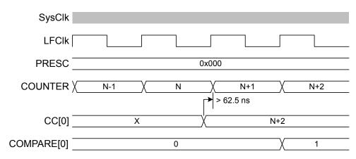
Figure 96: Timing diagram - COMPARE\_N+2
