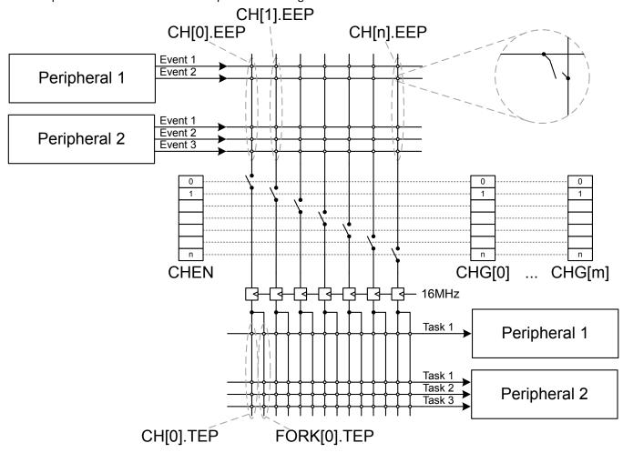
Figure 46: PPI block diagram
