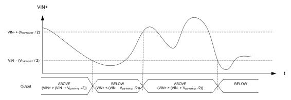
Figure 35: Hysteresis enabled in differential mode
