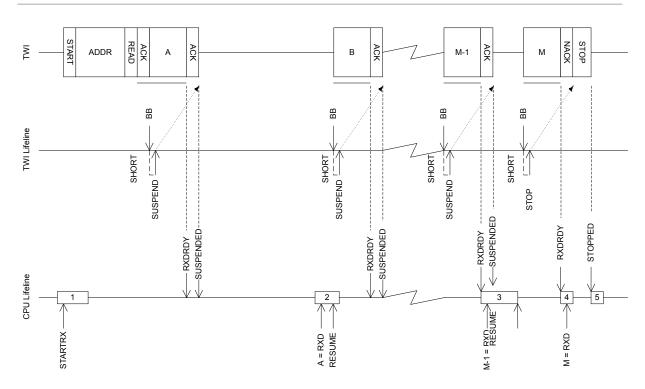
Figure 125: The TWI master reading data from a slave
