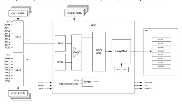
Figure 104: Simplified ADC block diagram
