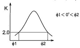
Contrast ratio K vs viewing angle  $\phi$
