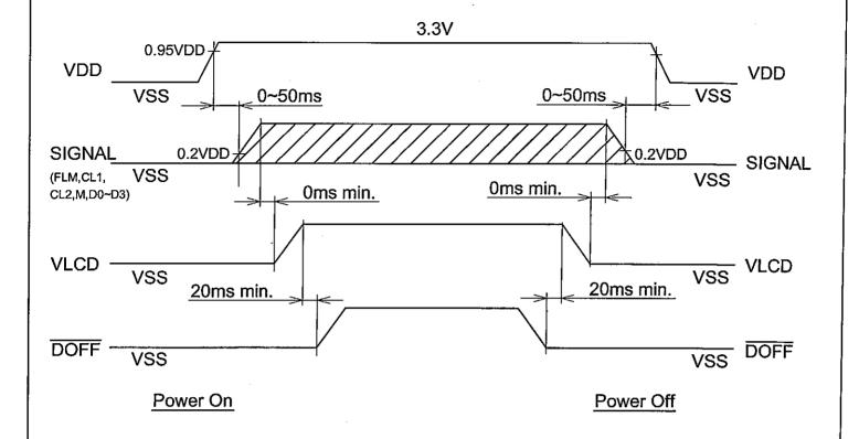
Note 1 DOFF function takes priority even if the input signal status becomes irregular immediately after VDD power-on. Note 2 Please keep the specified sequence because wrong sequence may cause permanent damage to the LCM.
