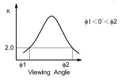
Contrast ratio K vs viewing angle  $\phi$
