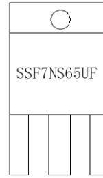
Marking and pin Assignment
