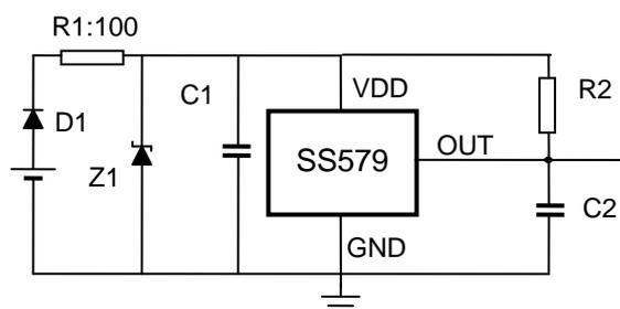
The SS579 have been optimized for commutation applications in 5V and 12V brushless DC motors. The following figure in the next page is the typical application circuit for 3 phase brushless DC motors.
