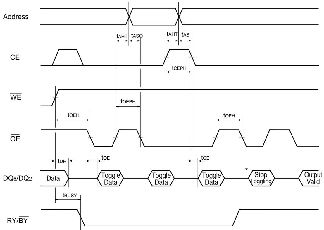
\* : DQ<sub>6</sub> stops toggling (The device has completed the Embedded operation).
