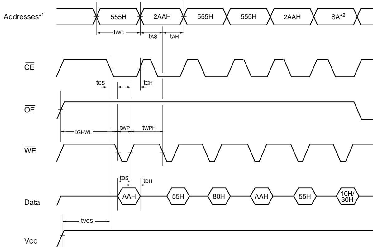
\*1: These waveforms are for the  $\times 16$  mode. (The addresses differ from  $\times 8$  mode.)
