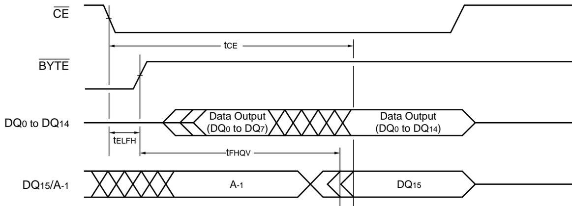
**Figure 15 Timing Diagram for Word Mode Configuration**
