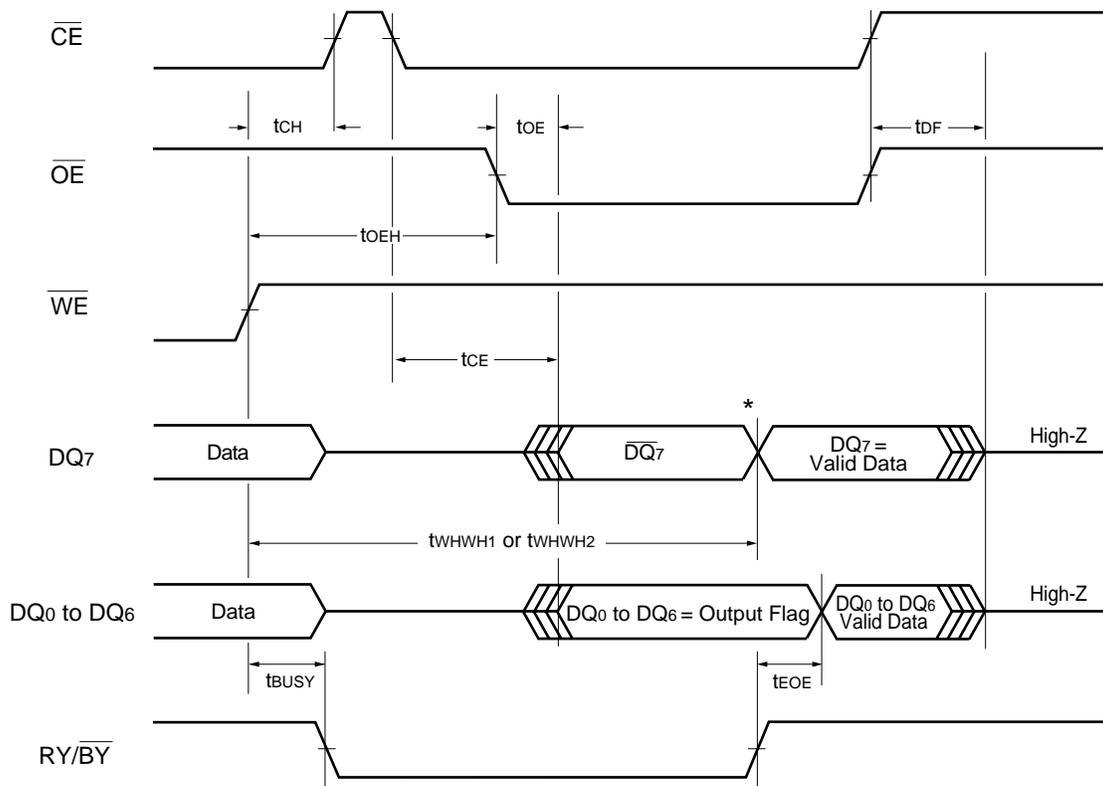
\* :  $DQ_7 = \text{Valid Data}$  (The device has completed the Embedded operation).
