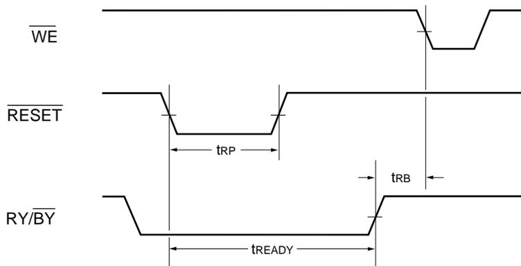
**Figure 14  $\overline{RESET}$ ,  $\overline{RY/BY}$  Timing Diagram**
