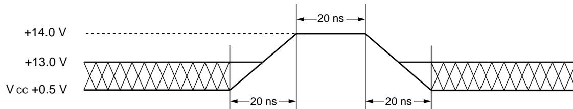
\*: This waveform is applied for  $A_9$ ,  $\overline{OE}$ , and  $\overline{RESET}$ .
