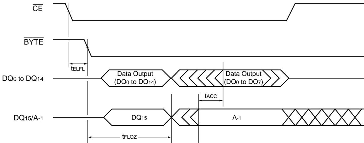
**Figure 16 Timing Diagram for Byte Mode Configuration**
