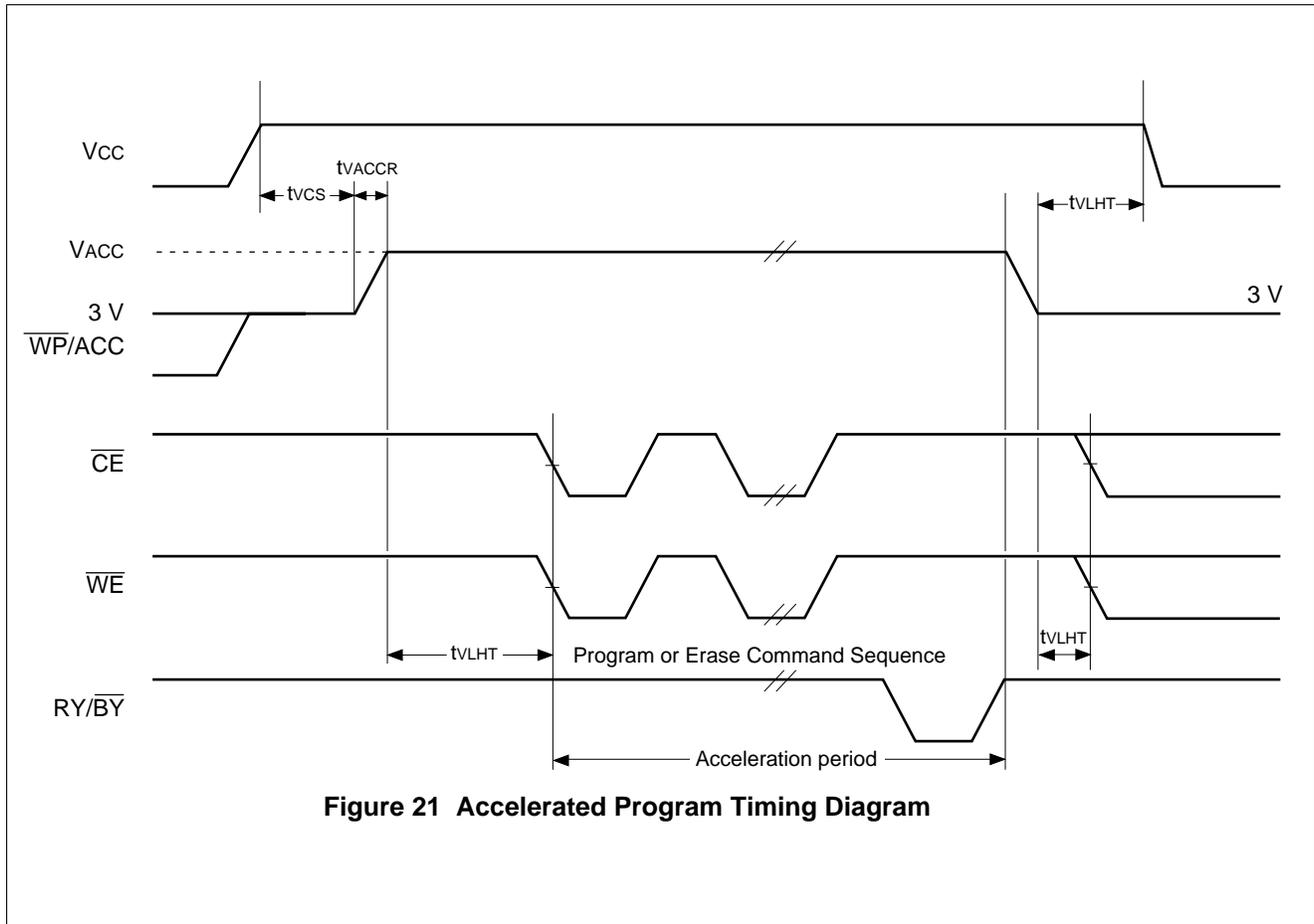
**Figure 21 Accelerated Program Timing Diagram**
