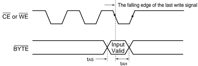
**Figure 17  $\overline{BYTE}$  Timing Diagram for Write Operations**
