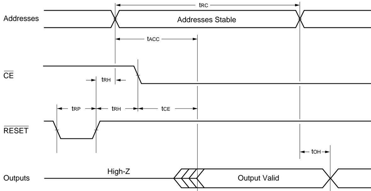
**Figure 5.2 AC Waveforms for Hardware Reset/Read Operations**
