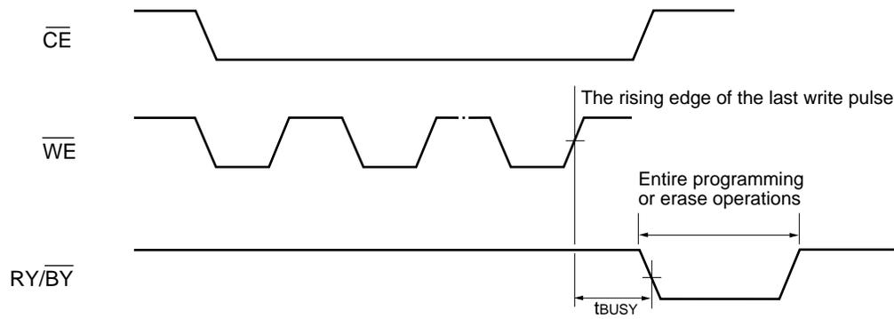
**Figure 13  $\overline{RY/BY}$  Timing Diagram during Program/Erase Operations**
