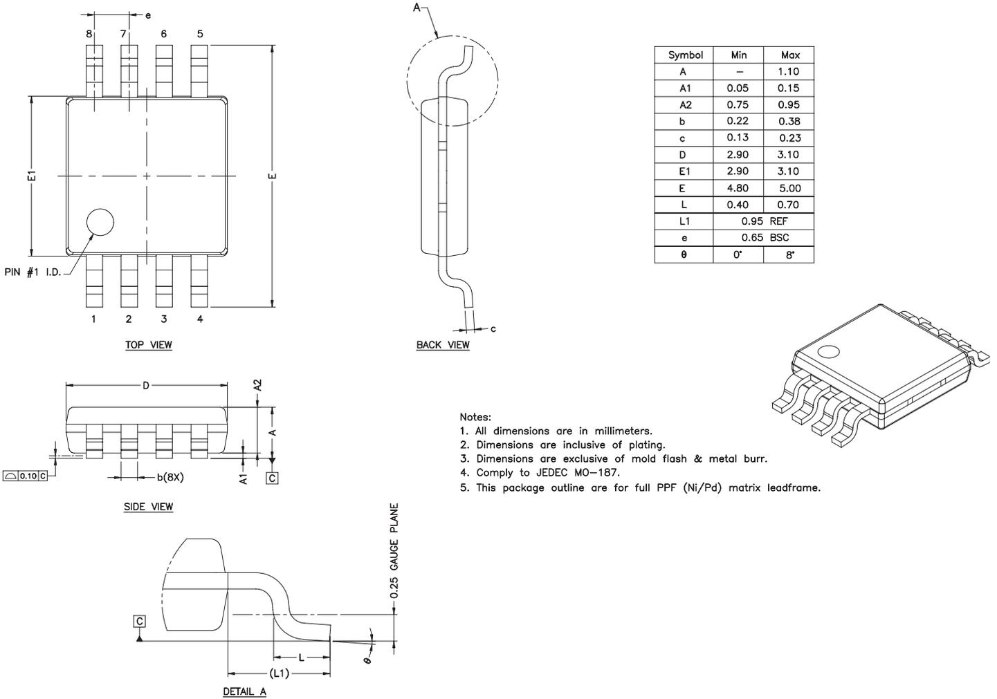
Figure 6.1 : Physical Dimensions of 8-pin MSOP Package
