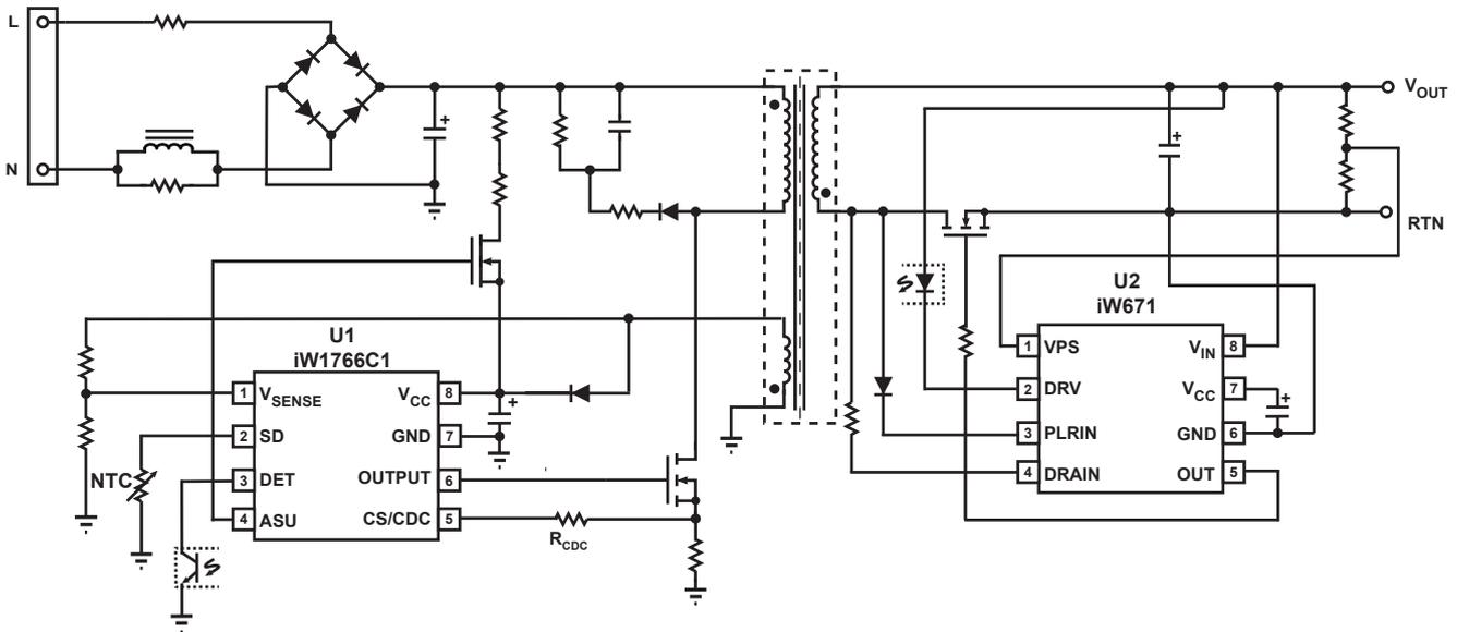
**Figure 3.2 : iW671 Typical Application Circuit (Using iW1766C1 as Primary-Side Controller)**
