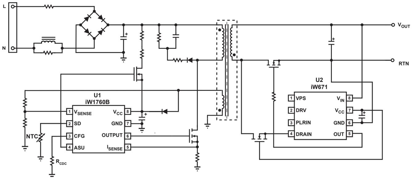
**Figure 3.3 : iW671 Typical Application Circuit for 12V-Output Application**
