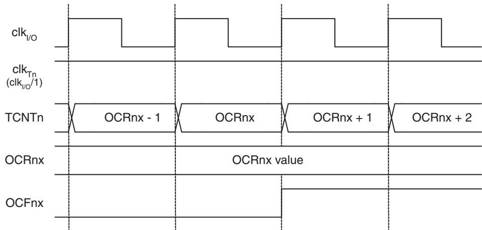
[Figure 15-11 on page 135](#) shows the same timing data, but with the prescaler enabled.
