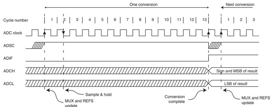
**Figure 26-6.** ADC timing diagram, auto triggered conversion.
