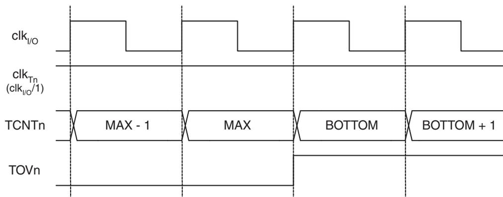
Figure 16-9 shows the same timing data, but with the prescaler enabled.
