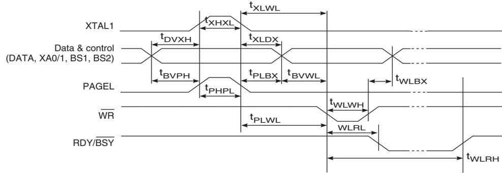
**Figure 30-8.** Parallel programming timing, loading sequence with timing requirements <sup>(1)</sup>.
