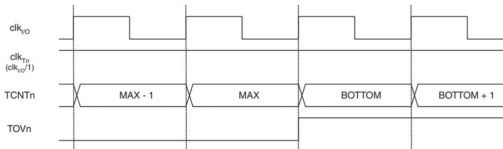
[Figure 14-9 on page 108](#) shows the same timing data, but with the prescaler enabled.
