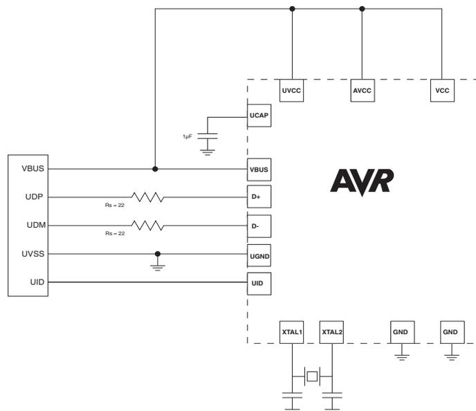
Figure 22-4. Typical bus powered application with 3V I/O.
