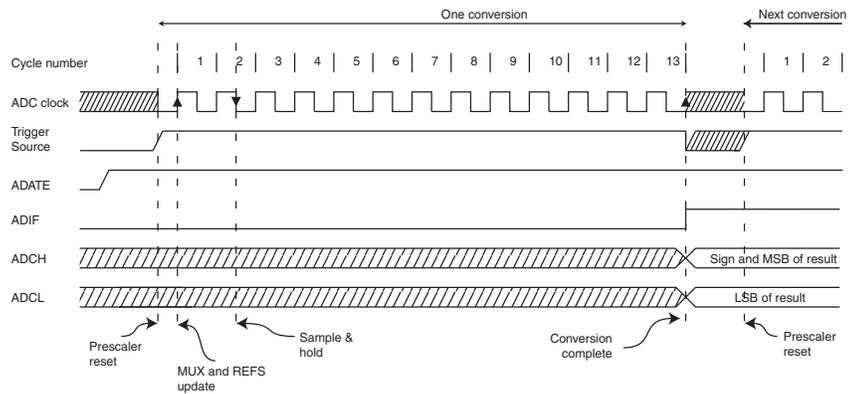
**Figure 26-7.** ADC timing diagram, free running conversion.
