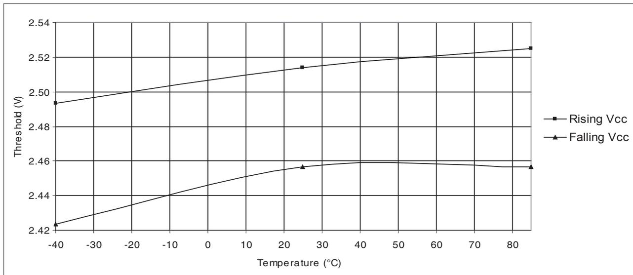
Figure 32-21. BOD voltage (3.4V level) vs. temperature.
