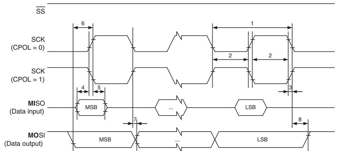
**Figure 31-5.** SPI interface timing requirements (slave mode).
