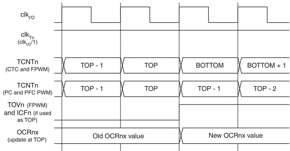
Figure 15-13 on page 136 shows the same timing data, but with the prescaler enabled.
