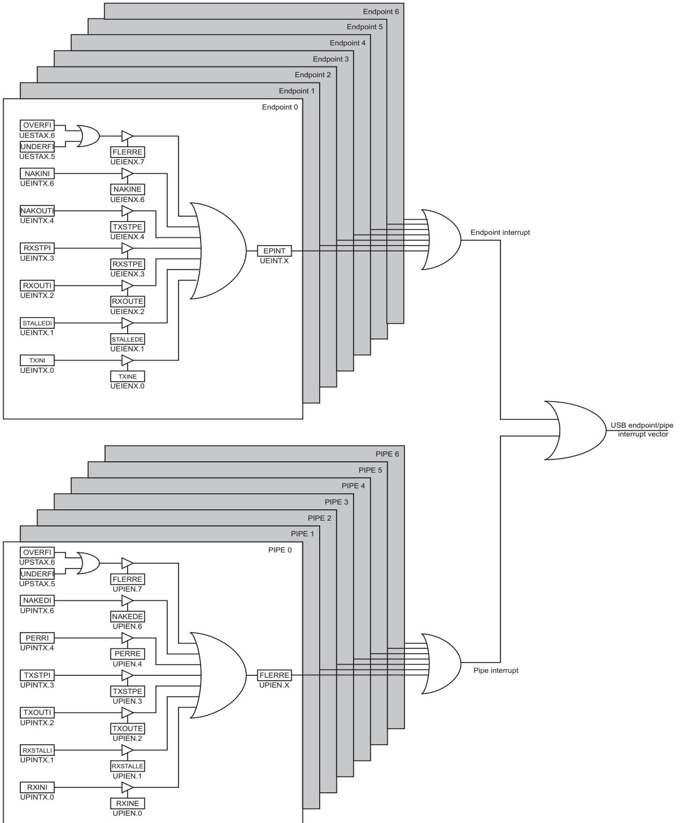
**Figure 22-13.** USB general and OTG controller interrupt system.
