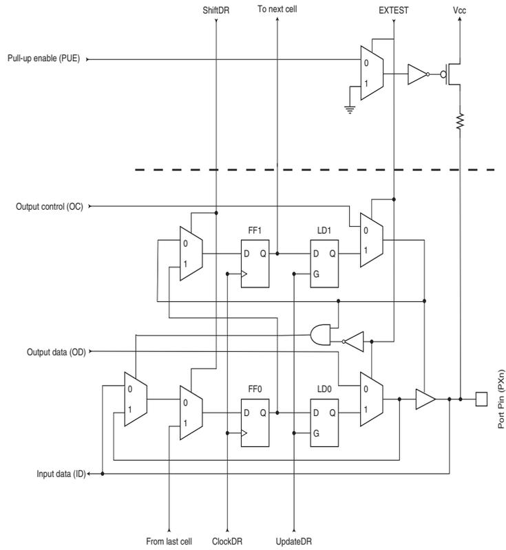
Figure 28-4. General port pin schematic diagram.
