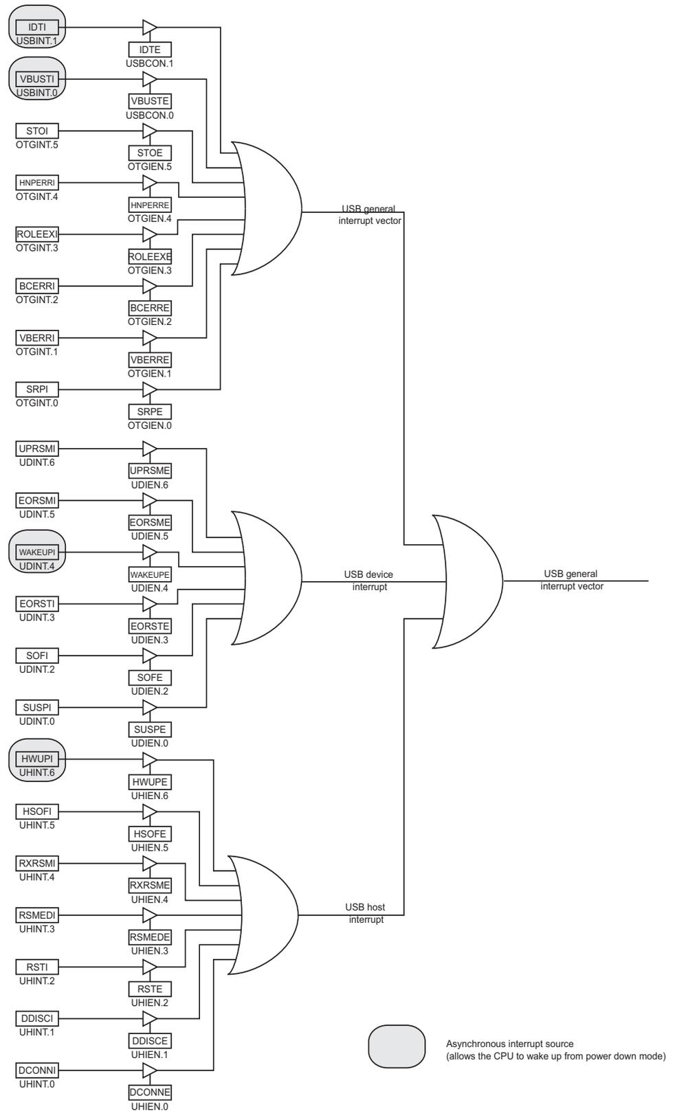
Figure 22-12. USB endpoint/pipe Interrupt vector sources.
