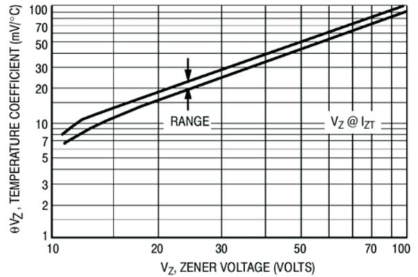
Figure 1. Temperature coefficients
