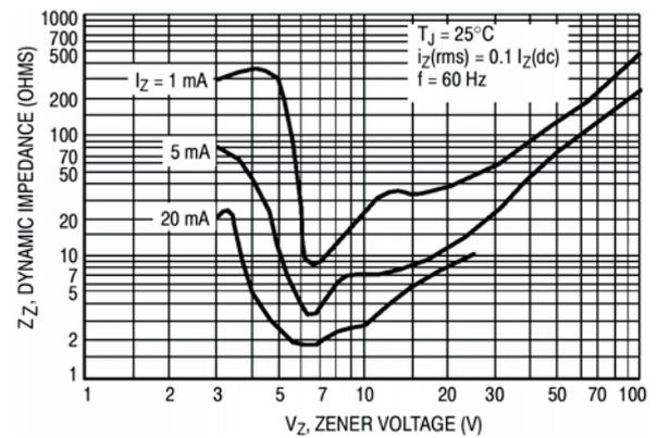
Figure 3. Effect of zener voltage on zener impedance
