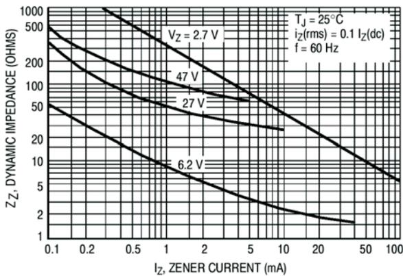
Figure 2. Effect of zener current on zener impedance
