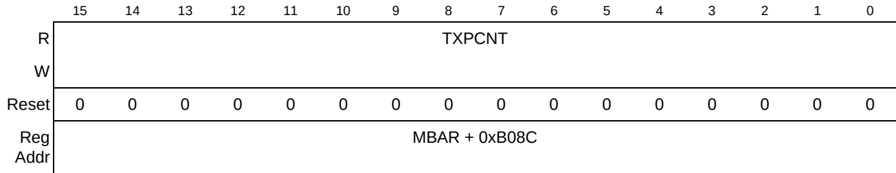
Figure 30-24. USB Transmitted Packet Counter Register (TXPCNT)
