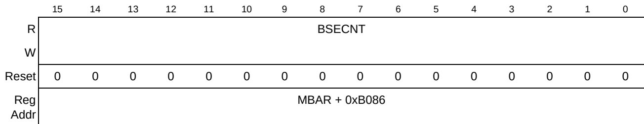
Figure 30-21. USB Bitstuffing Error Counter Register (BSECNT)
