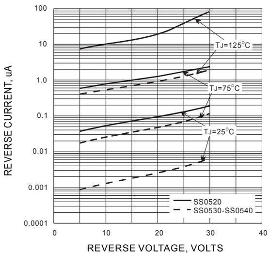
Fig.3 Typical Reverse Current
