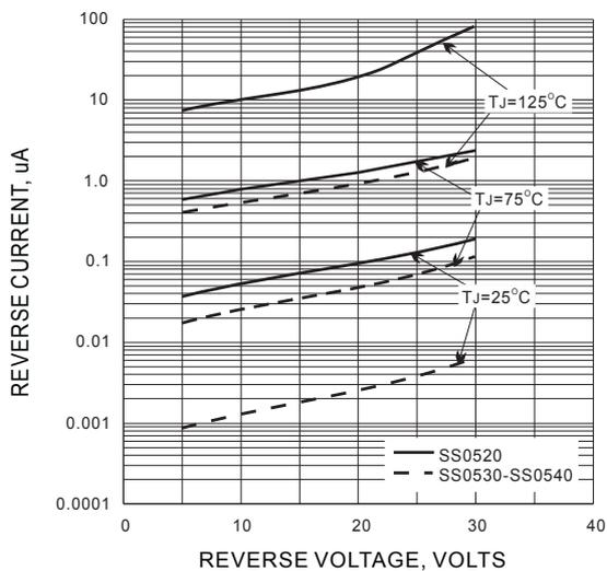
Fig.3 Typical Reverse Current
