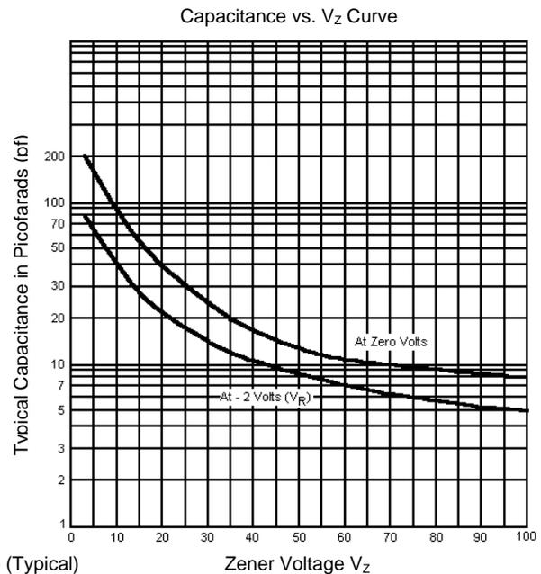
**FIGURE 3** Capacitance vs. Zener Voltage (Typical)
