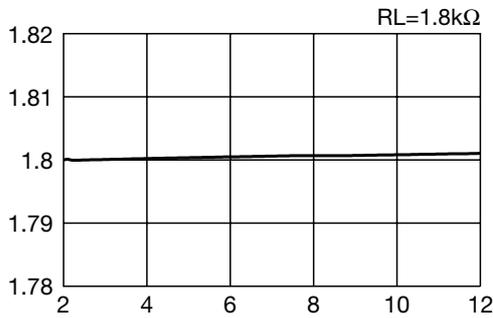
**Output Voltage- Ambient Temperature**
