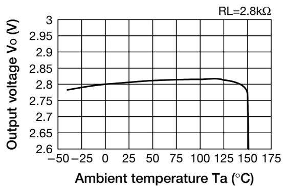
**Characteristics** ( $V_o=2.8V$  Except where noted otherwise,  $T_a=25^\circ C$ ,  $V_{in1}=V_o+1V$ ,  $V_{cont}=2V$ ,  $C_{in}=1\mu F$ ,  $C_o=1\mu F$ ,  $C_n=0.01\mu F$ )
