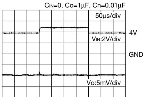
**Line Transient Responses ( $V_{IN}=3.8 \rightarrow 4.8V$ ,  $I_o=30mA$ )**
