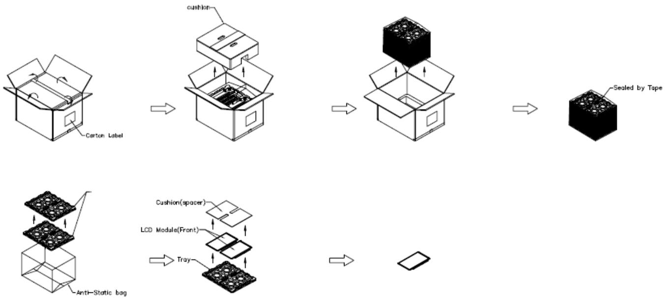
**Figure. 7-3 Un-Packing method**
