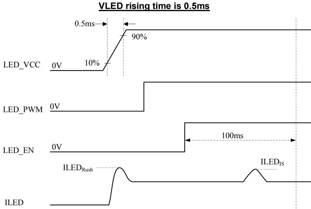
Note (2) If PWM control frequency is applied in the range less than 1KHz, the “waterfall” phenomenon on the screen may be found. To avoid the issue, it’s a suggestion that PWM control frequency should follow the criterion as below.
