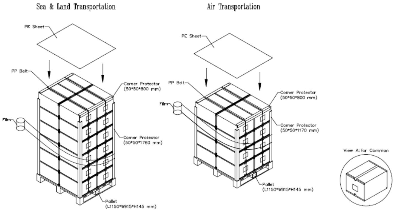
Figure. 7-2 Packing method
