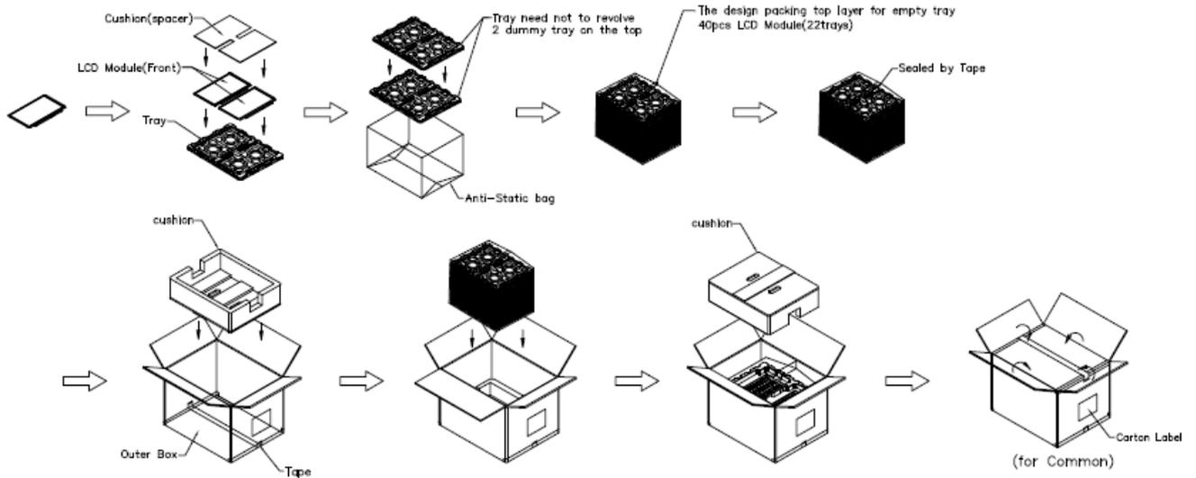
**Figure. 7-1 Packing method**
