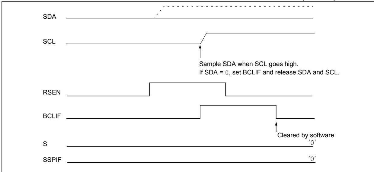
**FIGURE 22-37: BUS COLLISION DURING REPEATED START CONDITION (CASE 2)**
