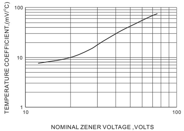
Fig.2 TEMPERATURE COEFFICIENTS
