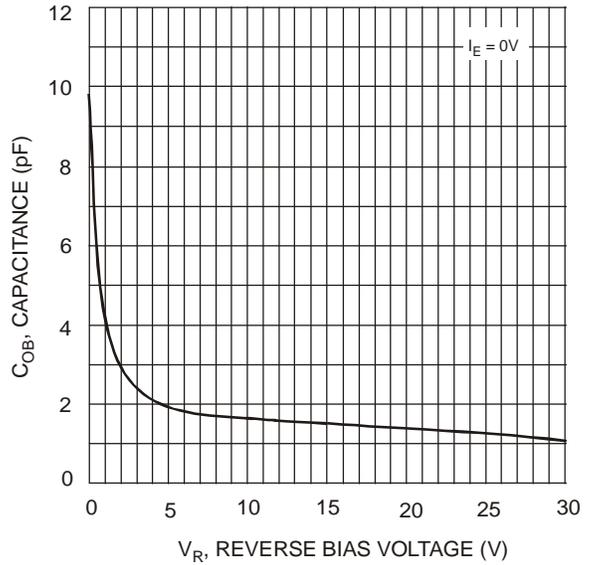
Fig. 4 Output Capacitance
