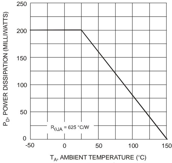
Fig. 1 Derating Curve
