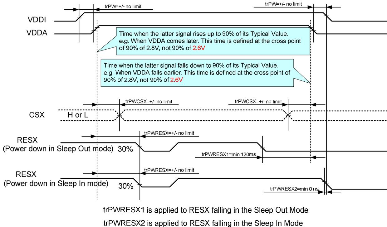
**Figure 174: Case 1 – RESX Line is Held High or Unstable by Host at Power ON**
