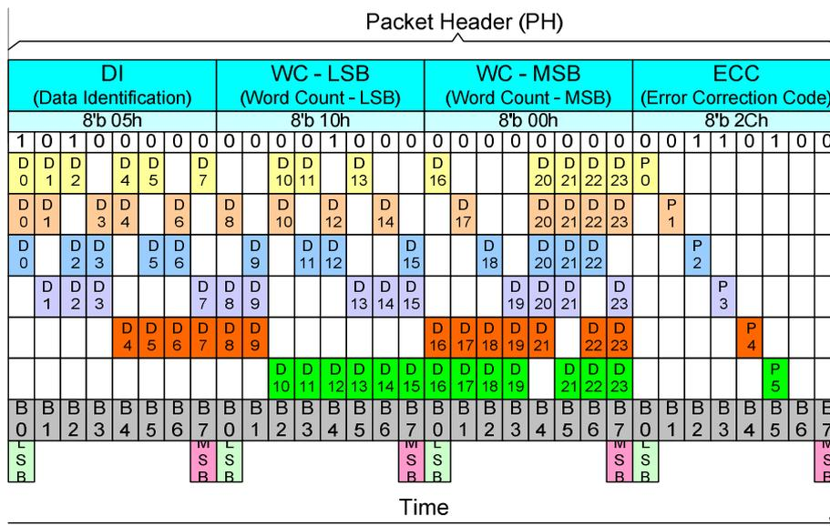
Figure 72: XOR Functionality in a Short Packet (SPa)
