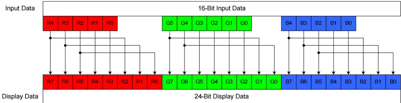
**Figure 155: EPF [1:0] = 10, 16-bit data mapping to 24-bit**
