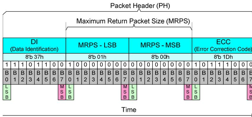
**Figure 86 Set Maximum Return Packet Size (SMRPS-S) - Example**
