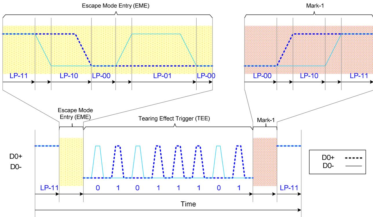
**Figure 40: Tearing Effect (TEE)**
