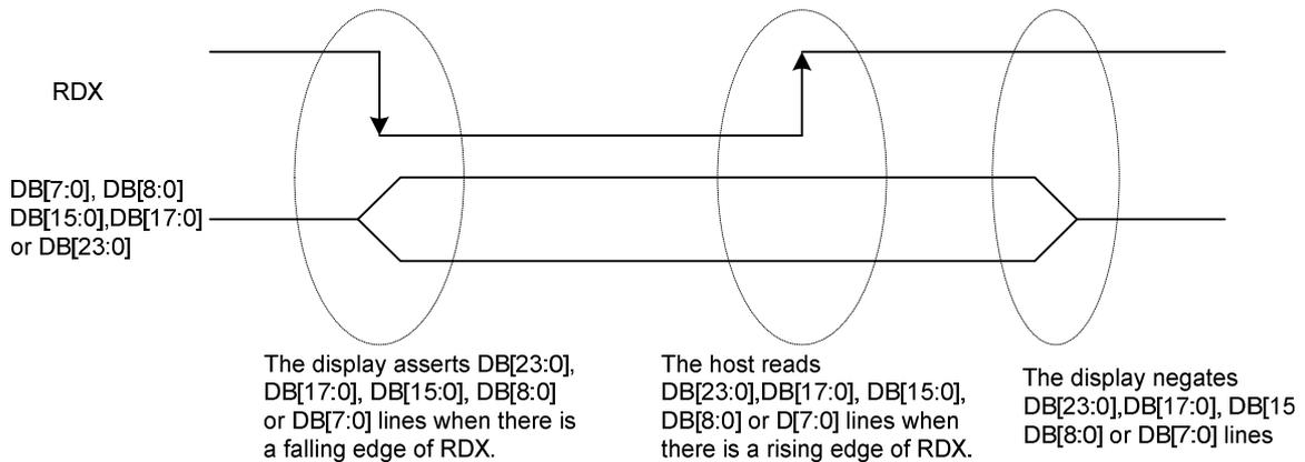
**Figure 4: DBI Type B Read Cycle** <sup>Note 1</sup>
