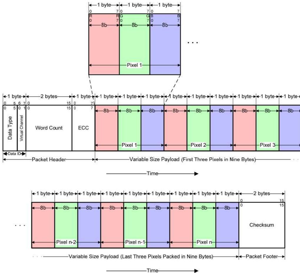
**Figure 160: 24-bit per Pixel, Data Type = 11 1110 (3Eh)**
