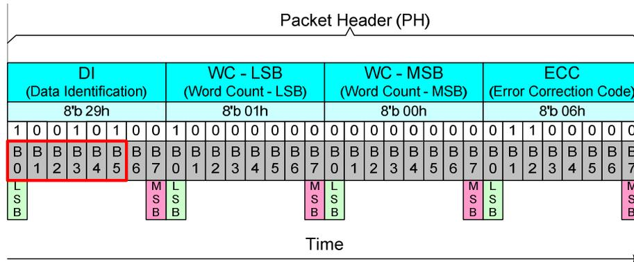
**Figure 65: Data Type (DT) in the Packet Header (PH)**
