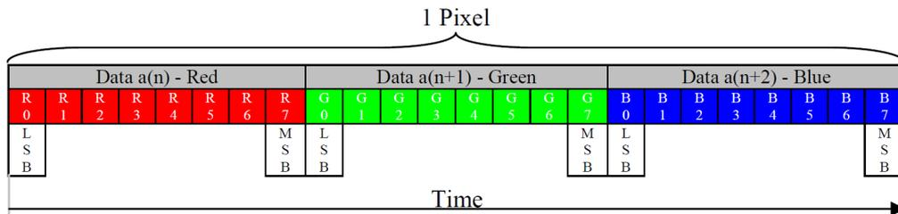
Figure 104: One Pixel Bit and Color Write Orders
