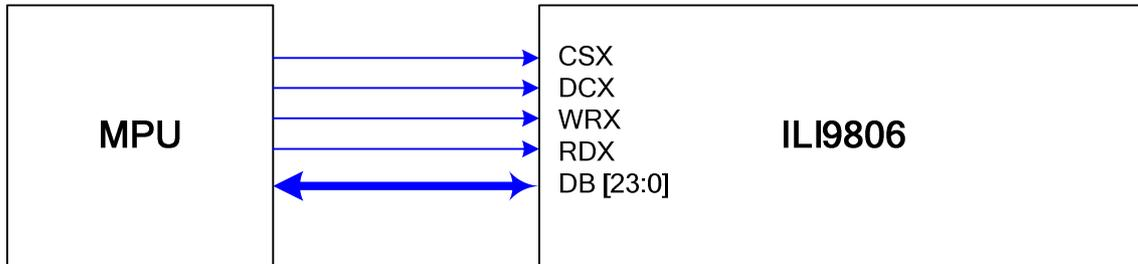
**Figure 150: 24-bit Parallel MPU Interface**
