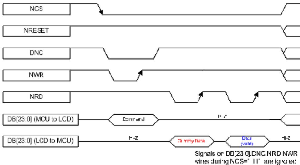
**Figure 5: DBI Type B Read Cycle Sequence** <sup>Note 2</sup>
