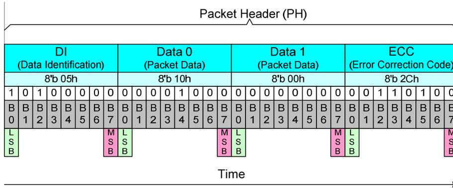
Figure 81: Display Command Set (DCS) Write, No Parameter (DCSWN-S) - Example
