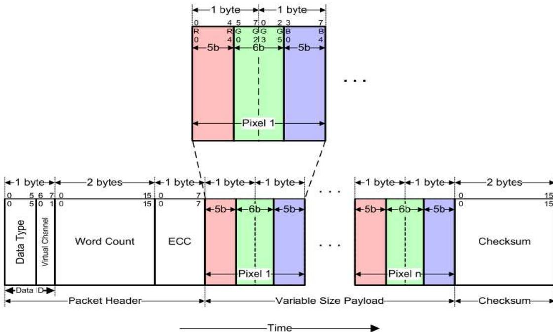
**Figure 157: 16-bit per Pixel, Data Type 00 1110 (0Eh)**
