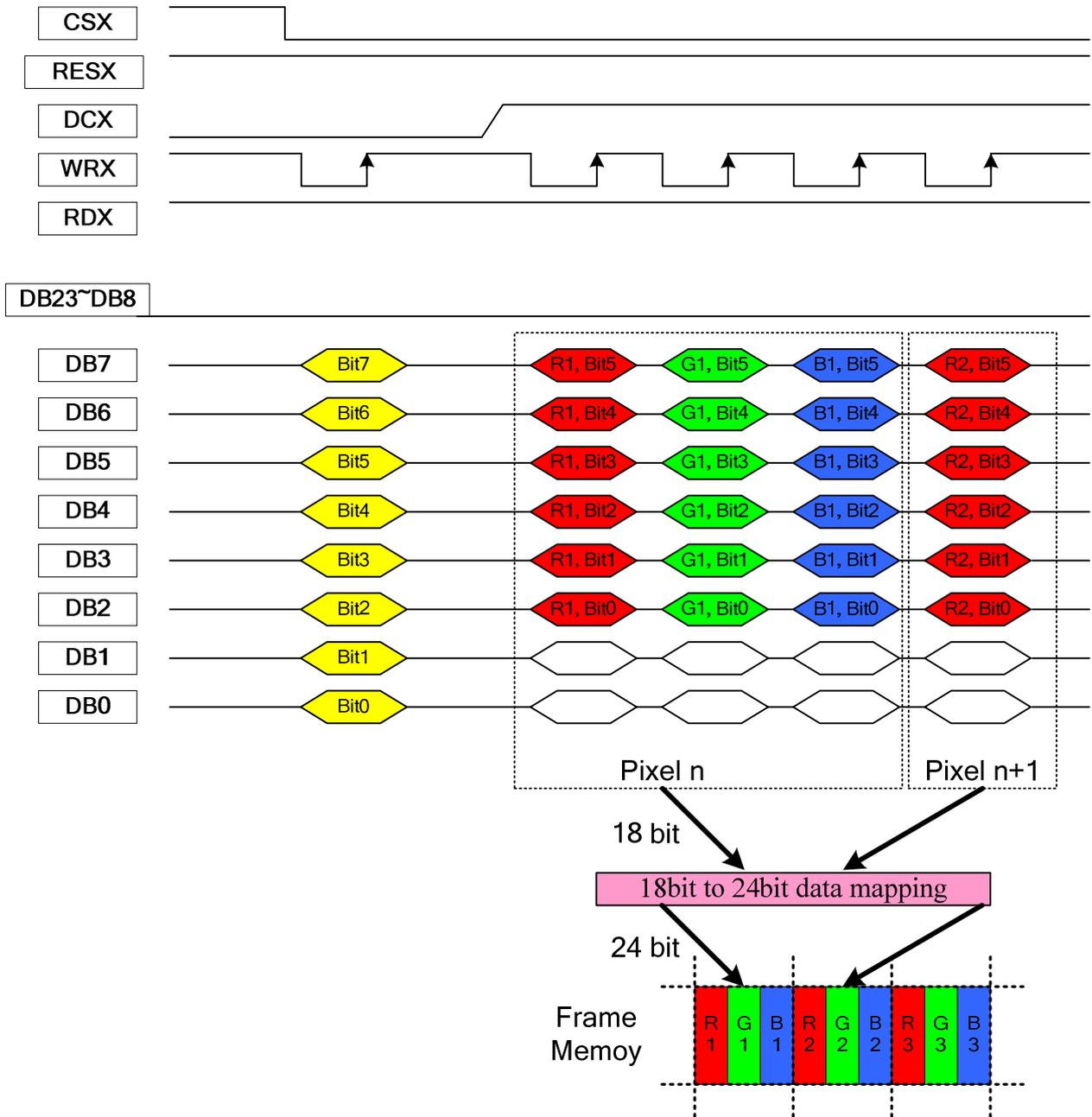
**Figure 136: 8-bit Data Bus for 18-bit/pixel (RGB 6-6-6 bits input), 262K-color**
