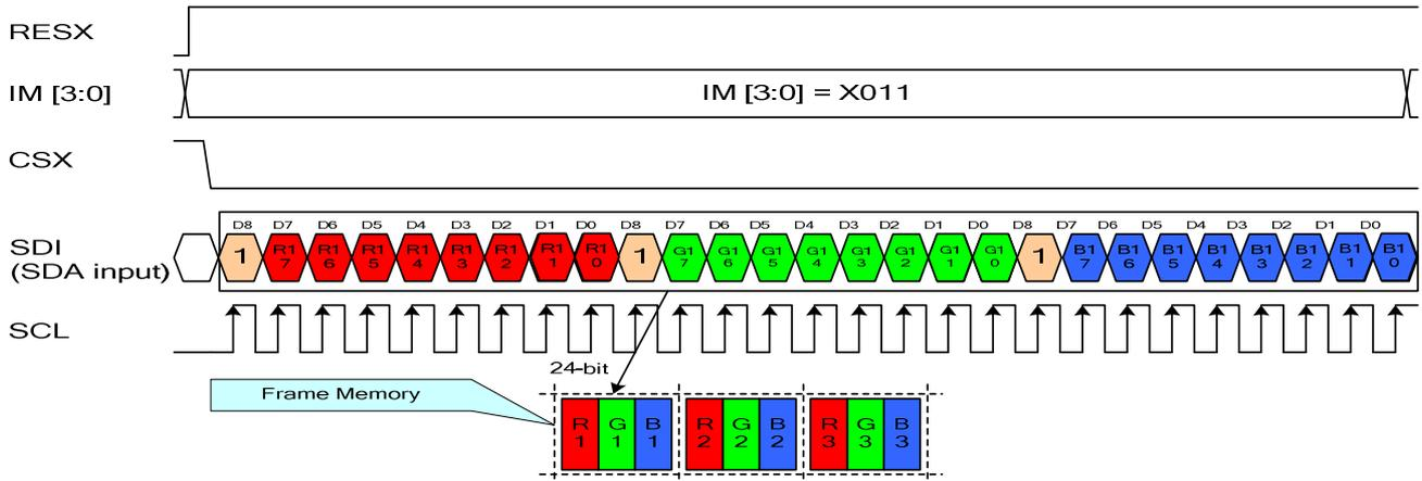
**Figure 132: SPI Data for 24-bit/pixel (RGB 8-8-8 bits input), 16.7M-color**
