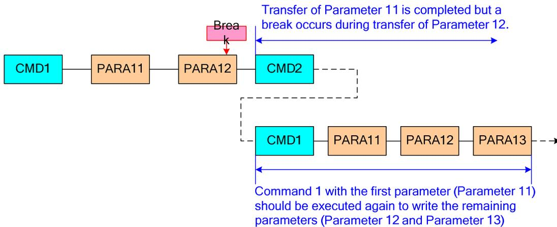
**Figure 15: Data Transfer Break - Case 1**
