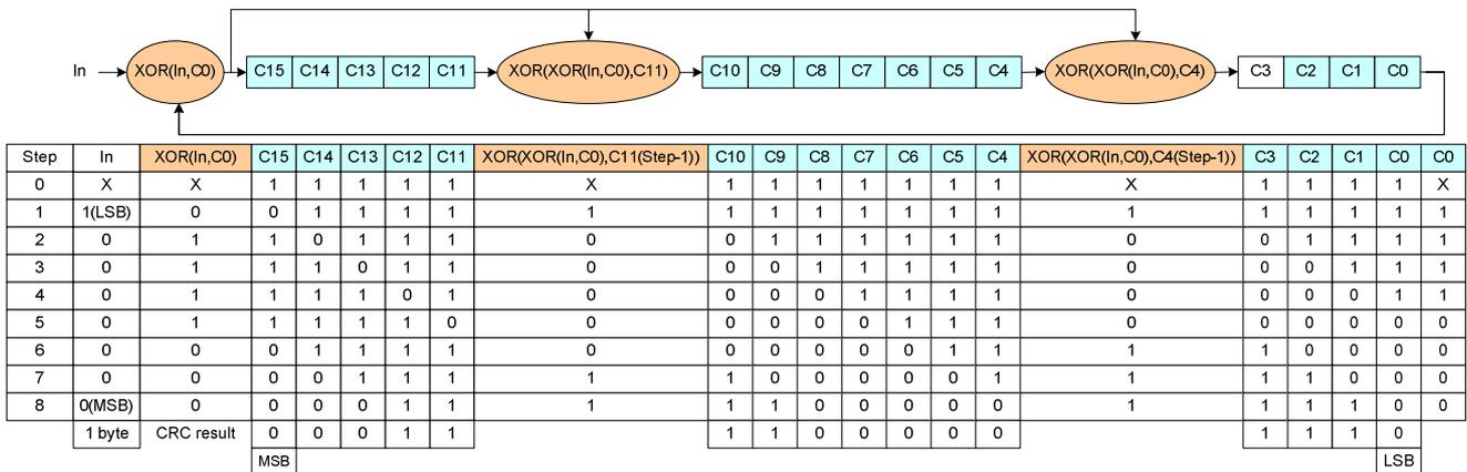
**Figure 78: CRC Calculation – Packet Data (PD) is 01h**
