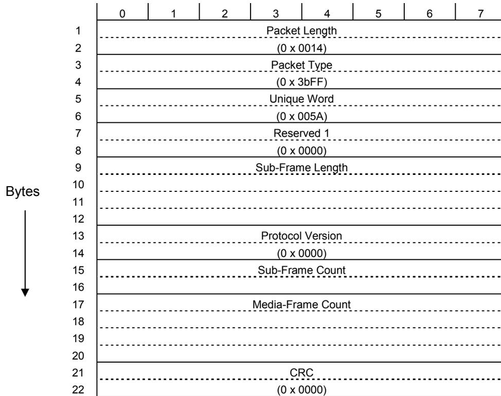
**Figure 119: Sub-Frame Header Packet**
