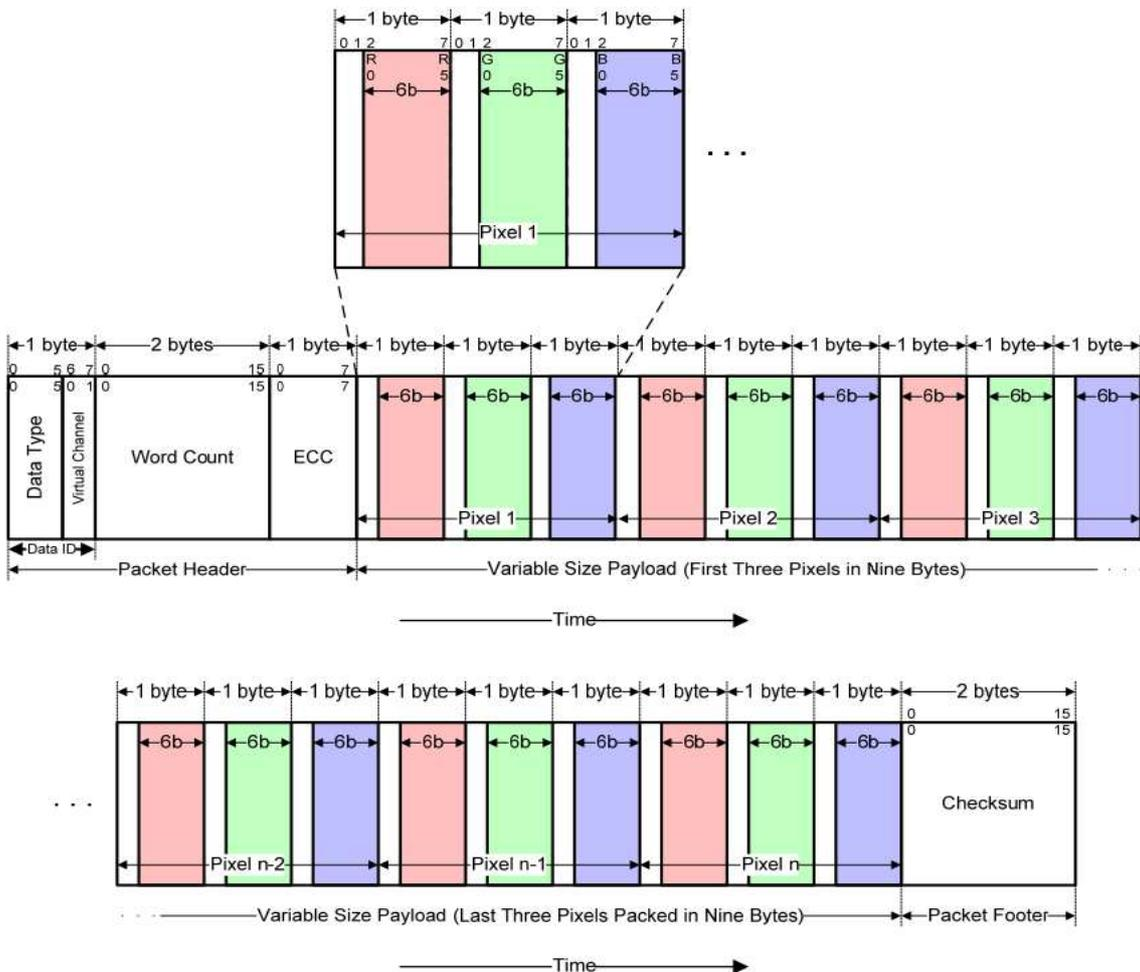
**Figure 159: 18-bit per Pixel, Data Type = 10 1110 (2Eh)**
