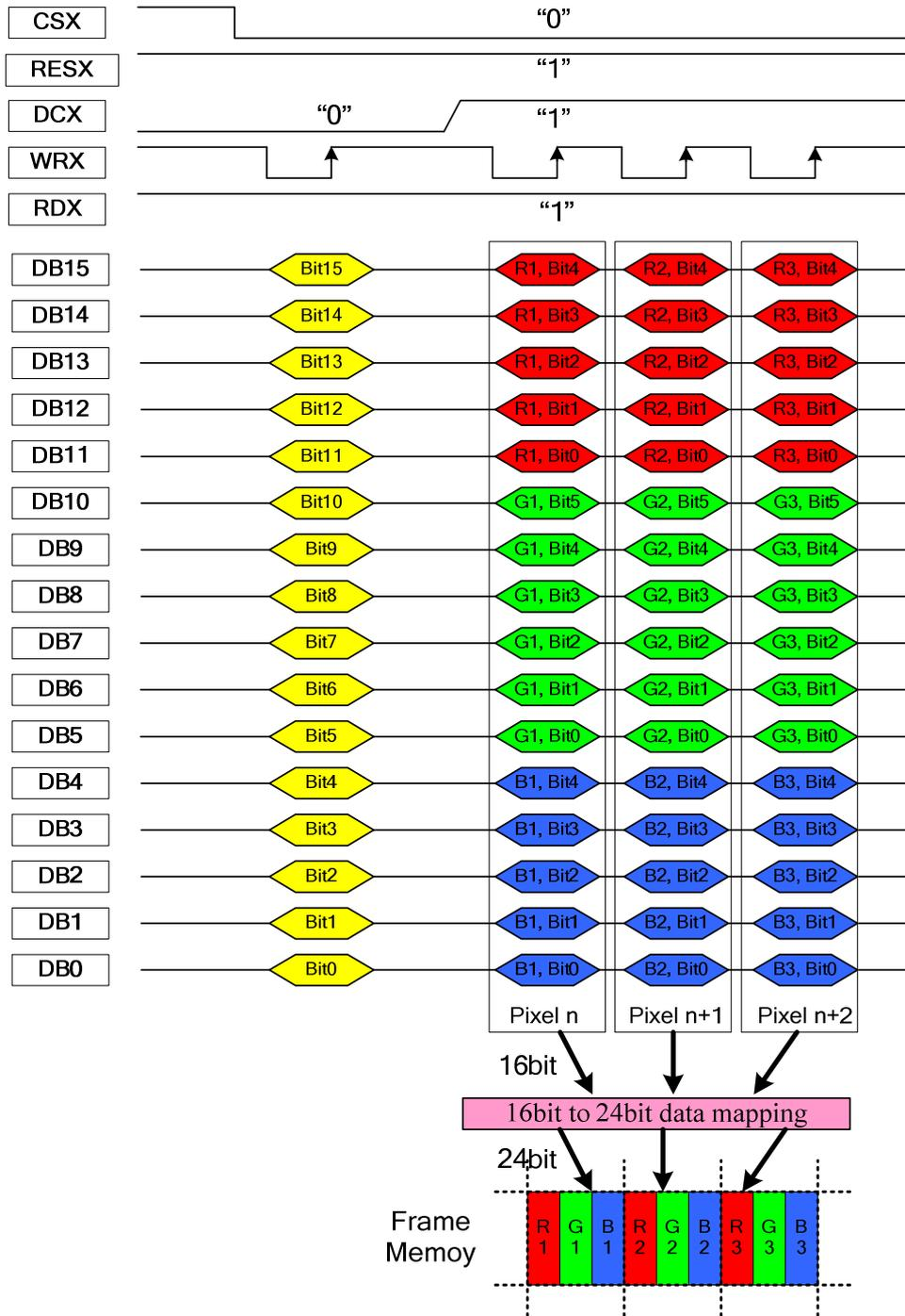
**Figure 143: 16-bit Data Bus for 16-bit/pixel (RGB 5-6-5 bits input), 65K-color**
