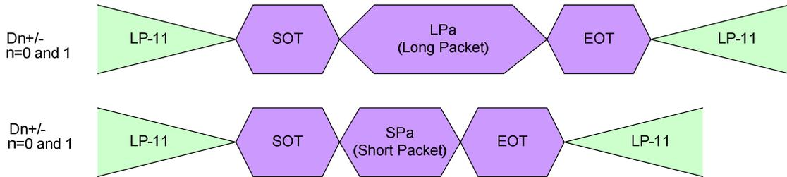
**Figure 44: Single Packet in High-Speed Data Transmissions**
