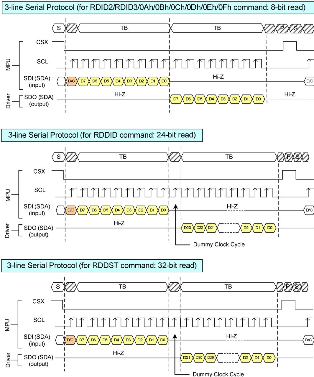
**Figure 13: DBI Type C Read Cycle Sequence**
