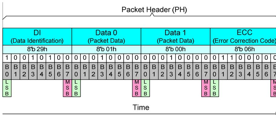
**Figure 60: Packet Header (PH) on Long Packet (LPa)**
