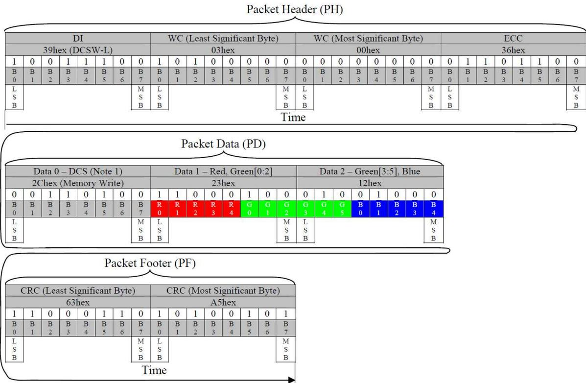
**Figure 101: One Pixel Write (DCSW-L) – Example 1<sup>Note</sup>**
