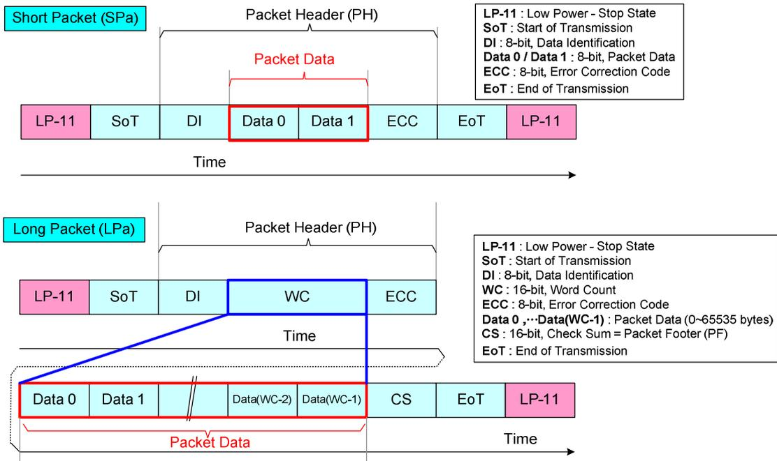
**Figure 69: Packet Data in Short and Long Packets**
