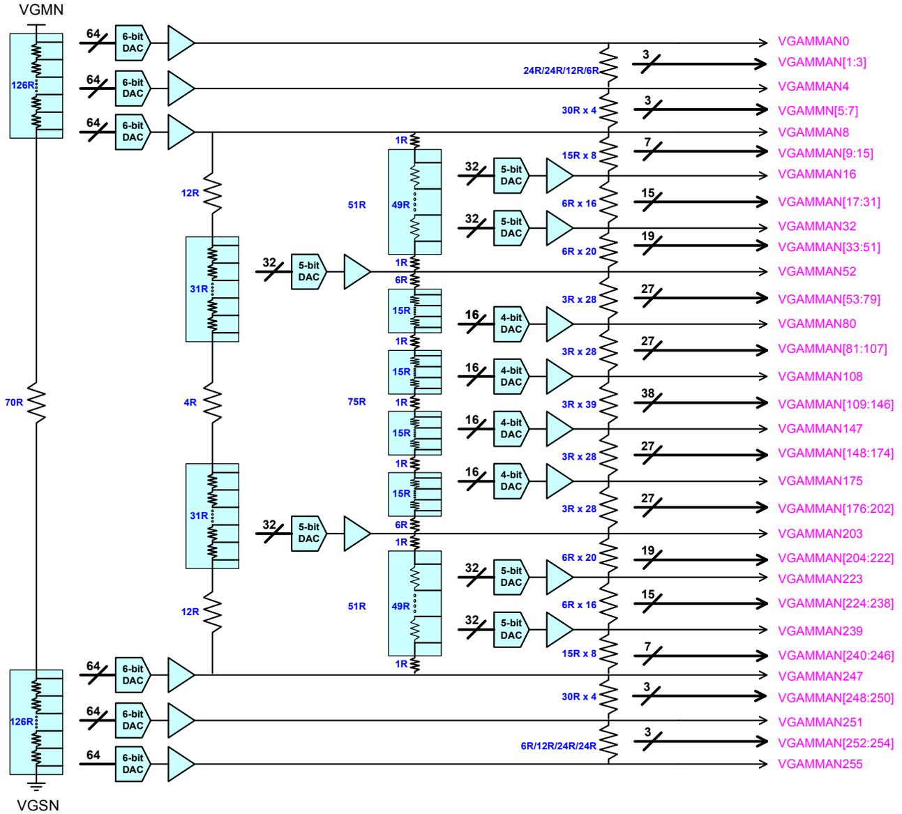
**Figure 186: Negative Gamma Control (E1h)**
