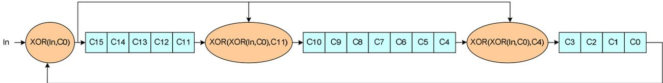
**Figure 77: 16-bit Cyclic Redundancy Check (CRC) Calculation**
