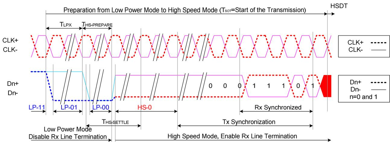
**Figure 42: Entering High-Speed Data Transmission (T<sub>SOT</sub> of HSDT)**
