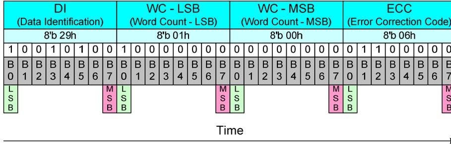
Figure 57: Bit Transmission Order of Bytes in Packets
