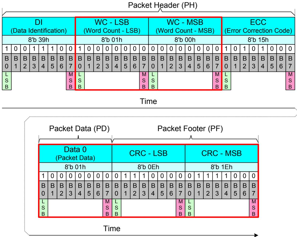
**Figure 79: Packet Footer (PF) Example**
