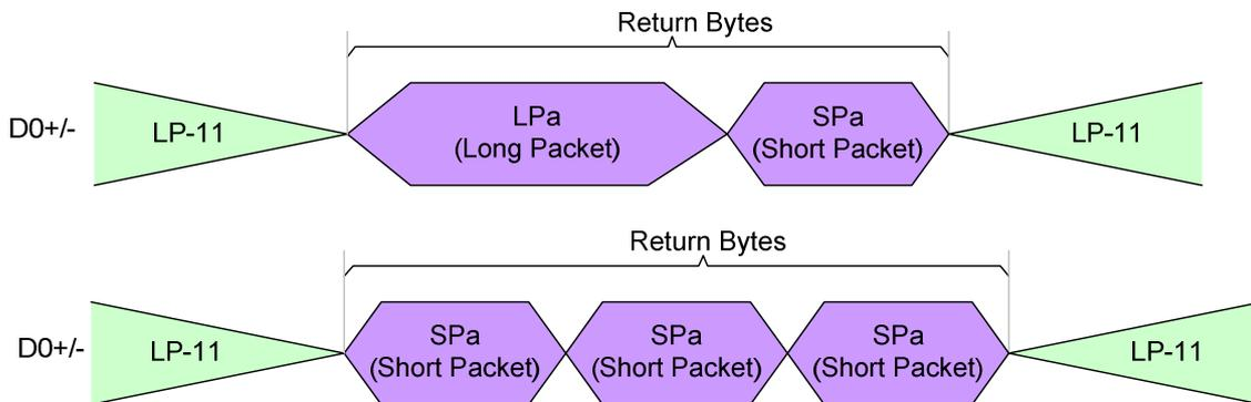
**Figure 92: Return Bytes in Several Packets – Not Allowed**
