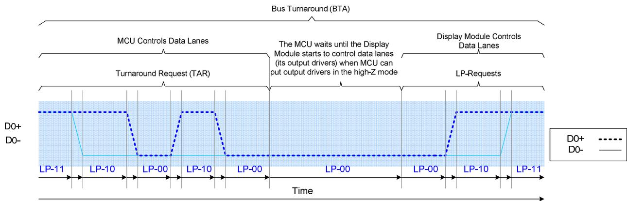
**Figure 54: Bus Turnaround Procedure**
