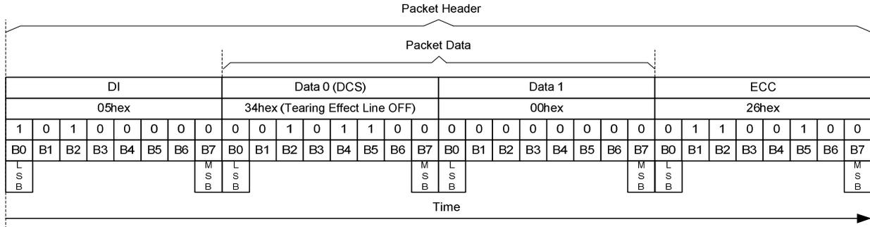
**Tearing Effect Bus Trigger Disable - Long Packet**
