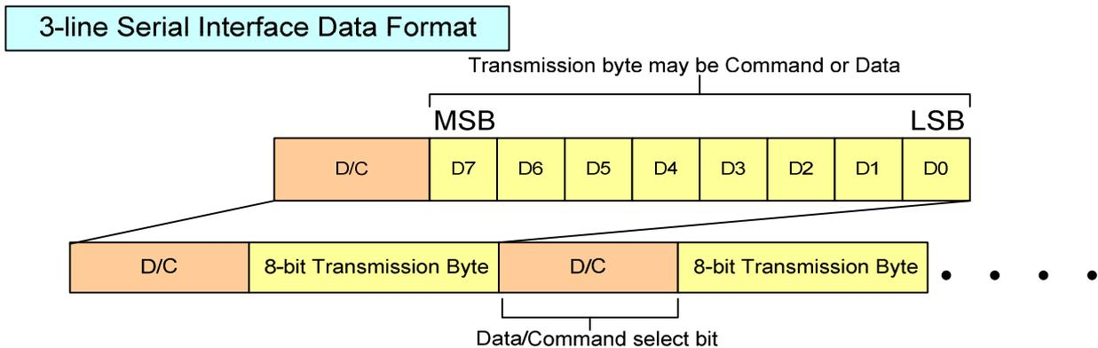
**Figure 11: DBI Type C Data Format**
