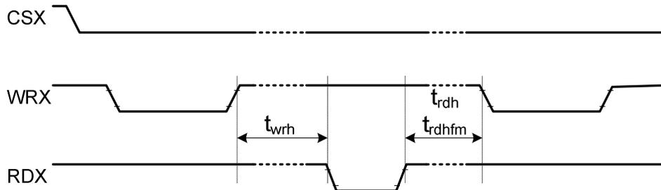
**18.4.2. Display Serial Interface Timing Characteristics (3-line SPI system)**
