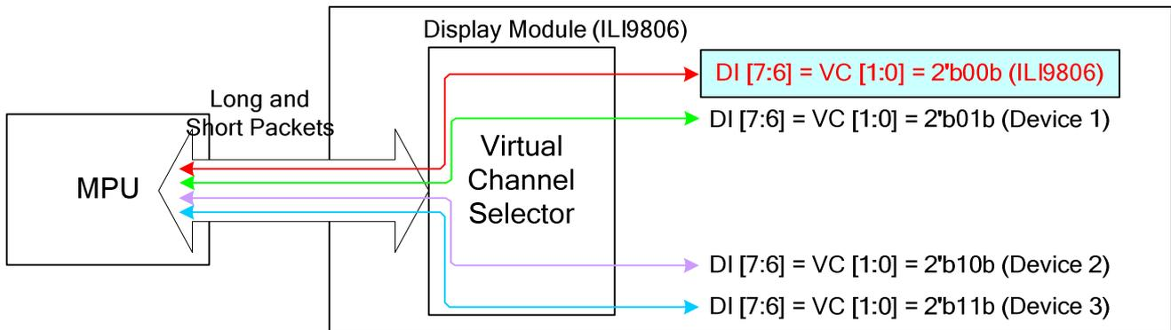
**Figure 64: Virtual Channel (VC) Configuration**
