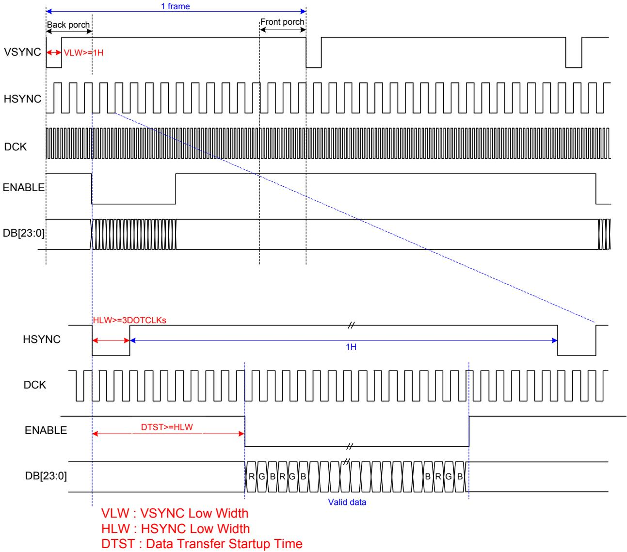
Figure 24: DPI Interface Timing diagram<sup>Note</sup>
