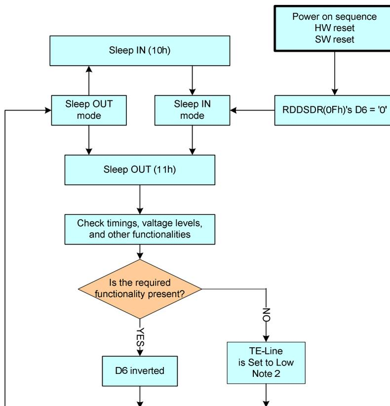
**Figure 173: Functionality Detection**
