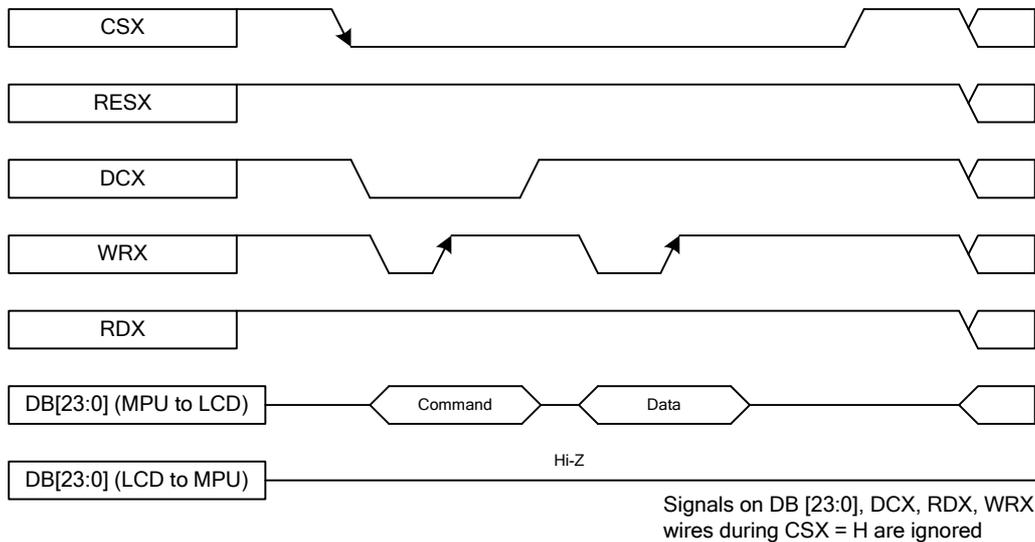
**Figure 3: DBI Type B Write Cycle Sequence**
