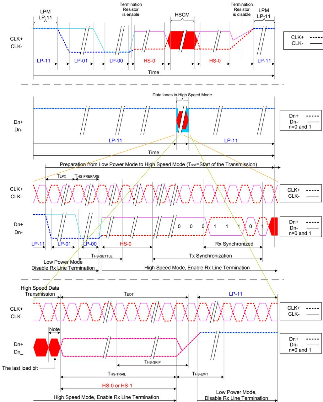
**Figure 34: High Speed Clock Burst**<sup>Note</sup>
