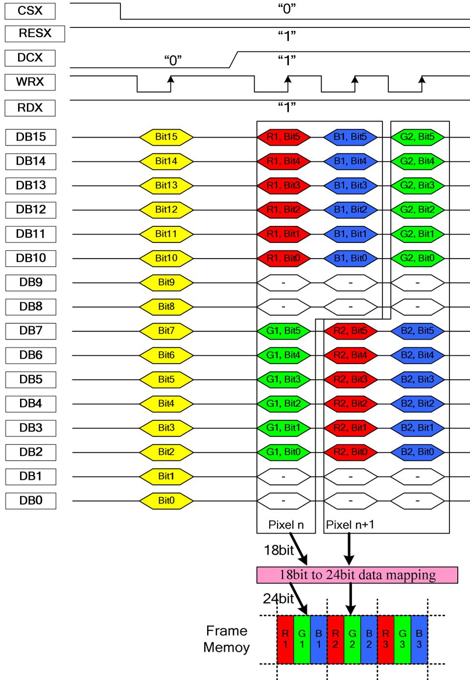
**Figure 144: 16-bit Data Bus for 18-bit/pixel (RGB 6-6-6 bits input), 262K-color**
