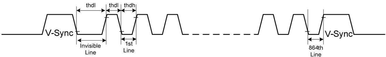
**Figure 168: Tearing Effect Line Mode 2**
