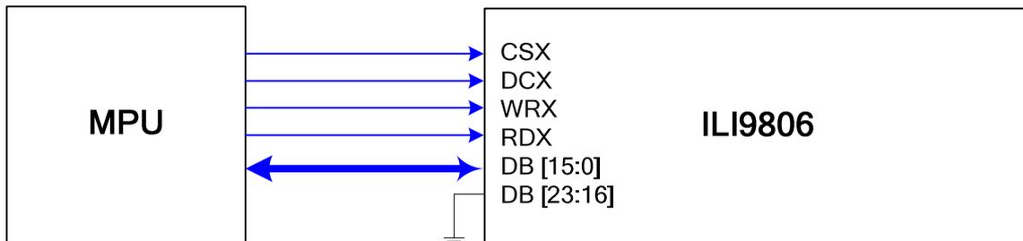
**Figure 142: 16-bit Parallel MPU Interface**
