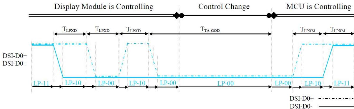
**Figure 197: BTA from the Display Module to the MPU**
