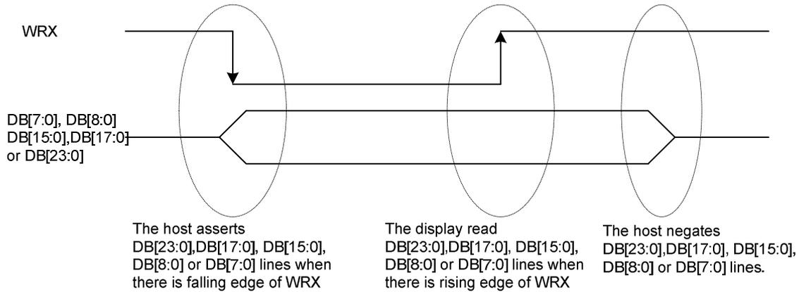
**Figure 2: DBI Type B Write Cycle**<sup>Note</sup>
