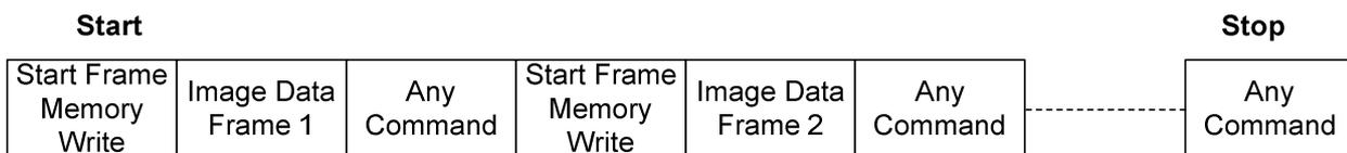
**Figure 21: Data Transfer Mode - Method 2**
