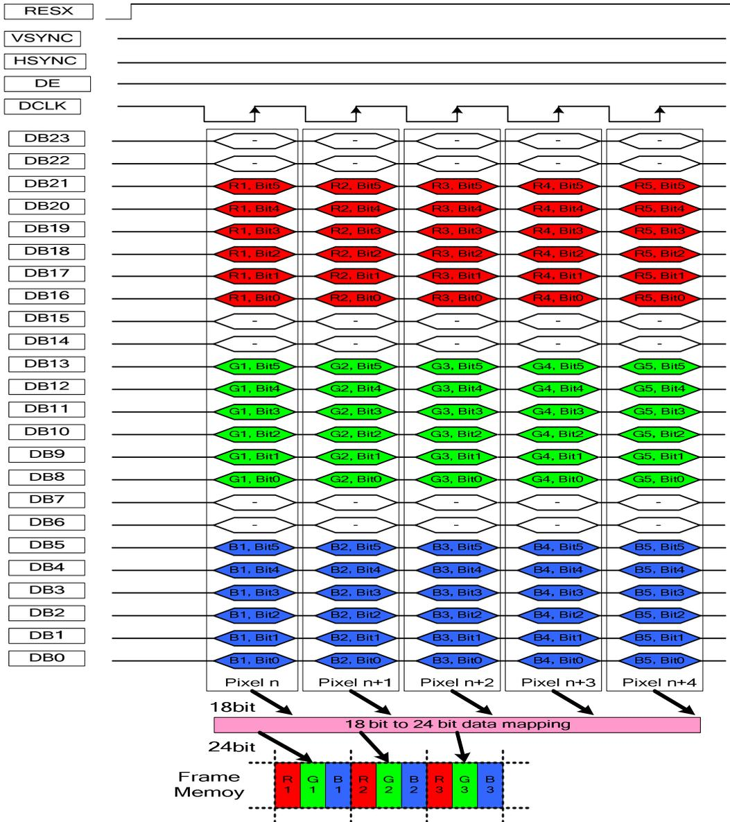
**Figure 153: 18-bit/pixel 262K colors order on the DPI Interface**
