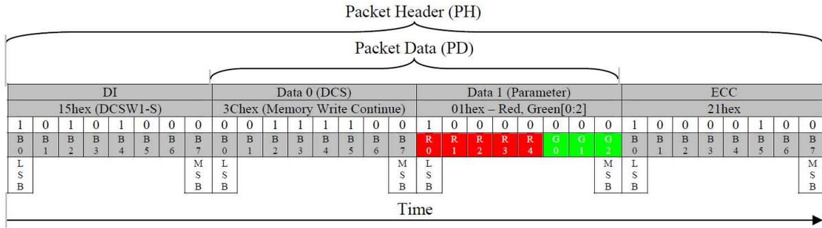
Figure 102: Red/Green [0:2] Subpixel Write (DCSW1-S) – Example 2<sup>Note 1</sup>
