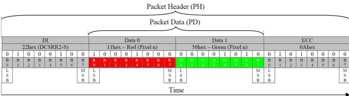
**Figure 114: Red and Green Subpixels Response (DCSRR2-S) – Example 5**
