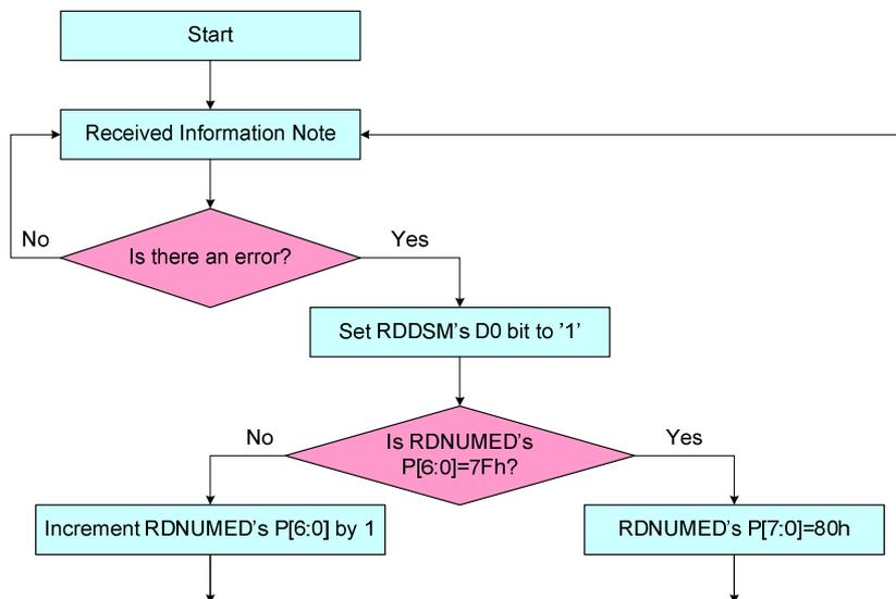
**Figure 96: Flow Chart for Errors on DSI<sup>Note</sup>**
