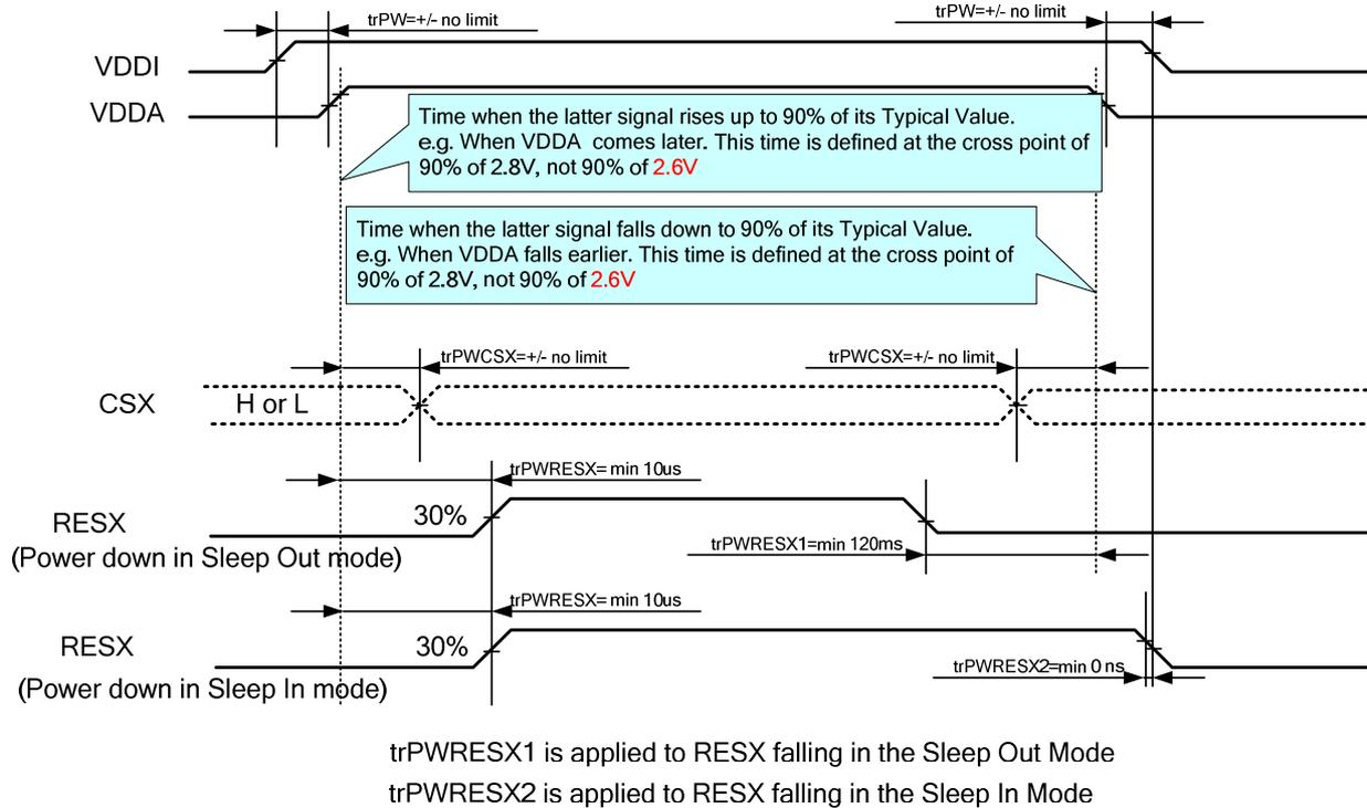
**Figure 175: Case 2 – RESX Line is Held Low by Host at Power ON**
