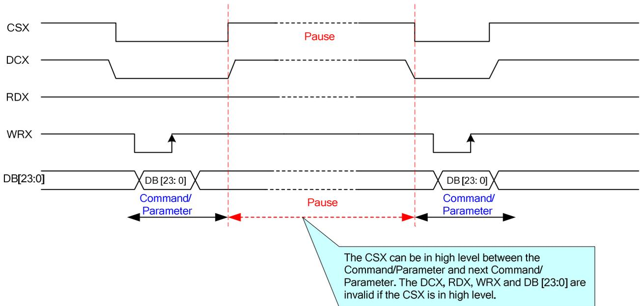
**Figure 19: DBI Type B Data Transfer Pause**
