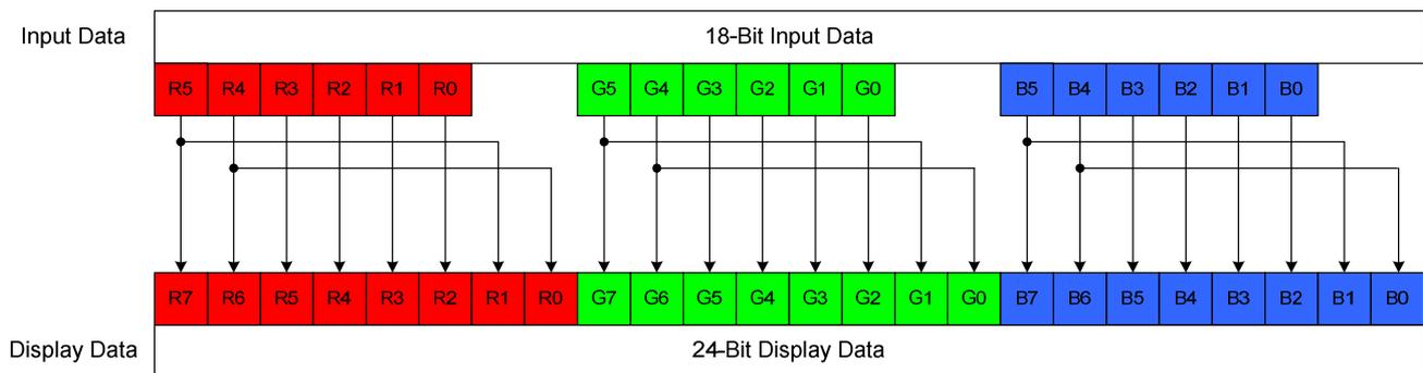
**Figure 156: EPF [1:0] = 10, 18-bit data mapping to 24-bit**
