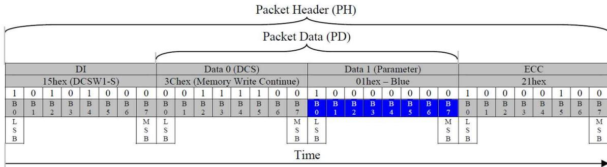
**Figure 106: Blue Subpixel Write (DCSW1-S) – Example 2**
