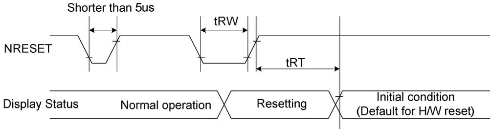
**Figure 182: Reset Timing**
