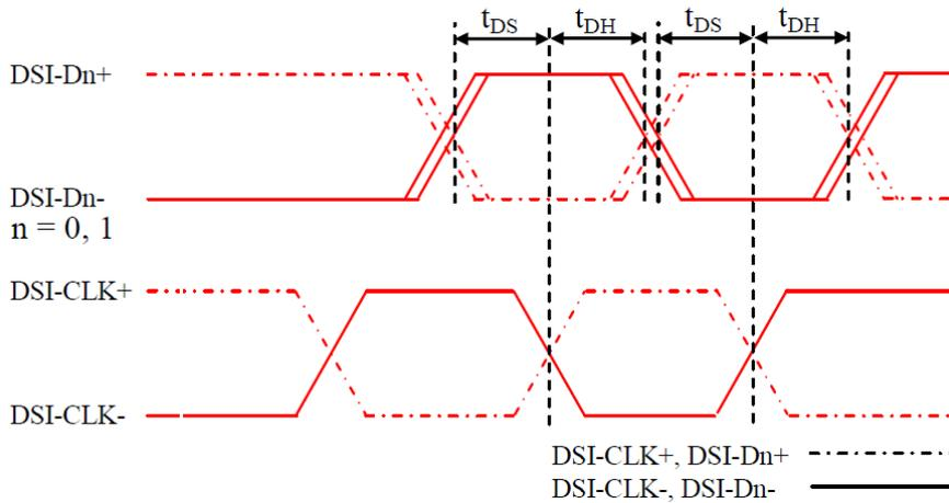
**Figure 194: DSI Data to Clock Channel Timings**
