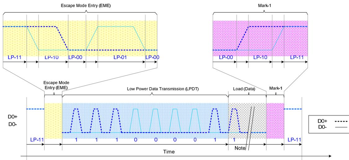
**Figure 36: Low-Power Data Transmission (LPDT)**<sup>Note</sup>
