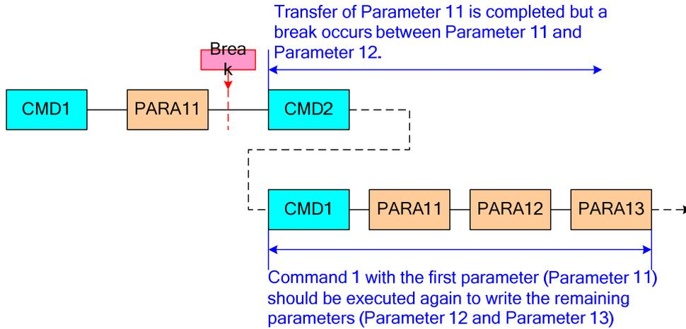
**Figure 16: Data Transfer Break - Case 2**
