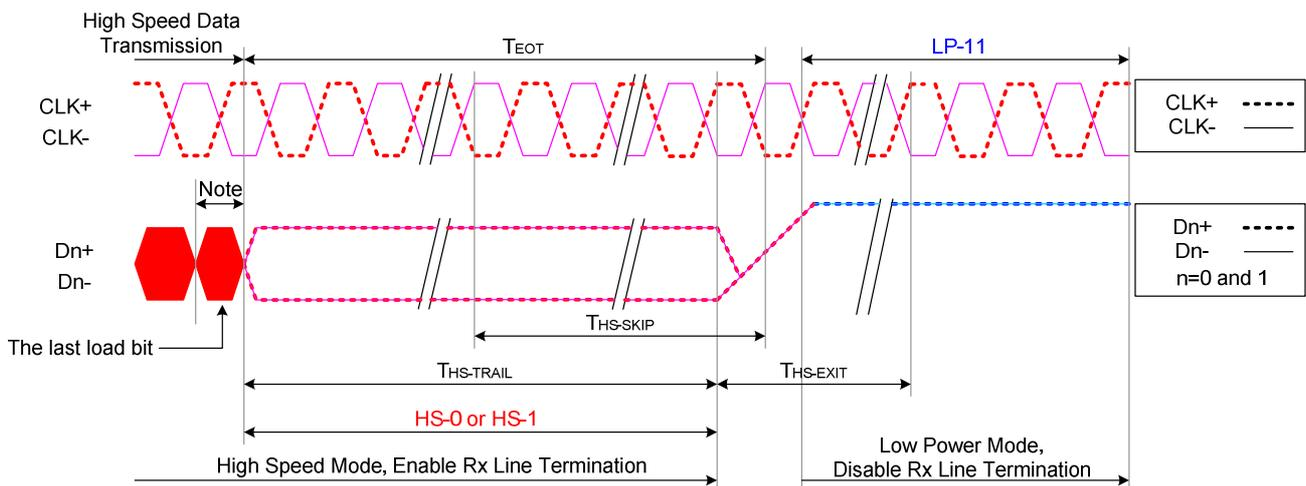
**Figure 43: Leaving High-Speed Data Transmission (T<sub>EOT</sub> of HSDT)<sup>Note</sup>**
