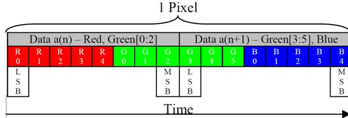
**Figure 100: One Pixel Bit and Write Color Orders**
