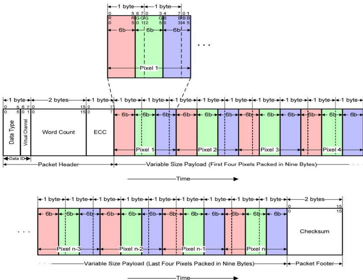
**Figure 158: 18-bit per Pixel, Data Type = 01 1110 (1Eh)**
