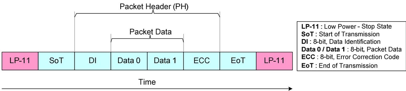
**Figure 55: Short Packet (SPa) Structure**
