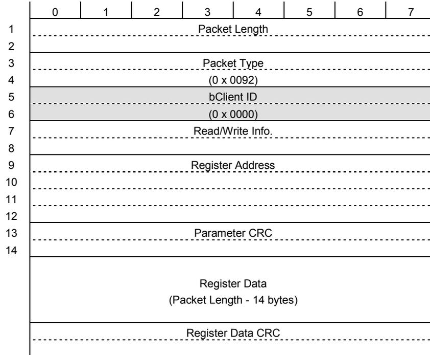
**Figure 122: Register Access Packet**<sup>Note</sup>
