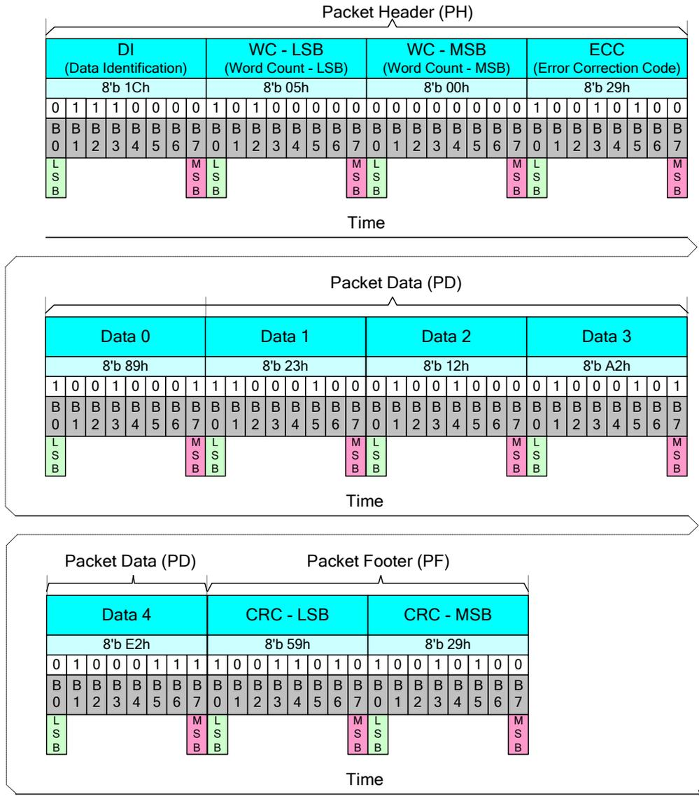
**Figure 97: DCS Read Long Response (DCSRR-L) - Example**
