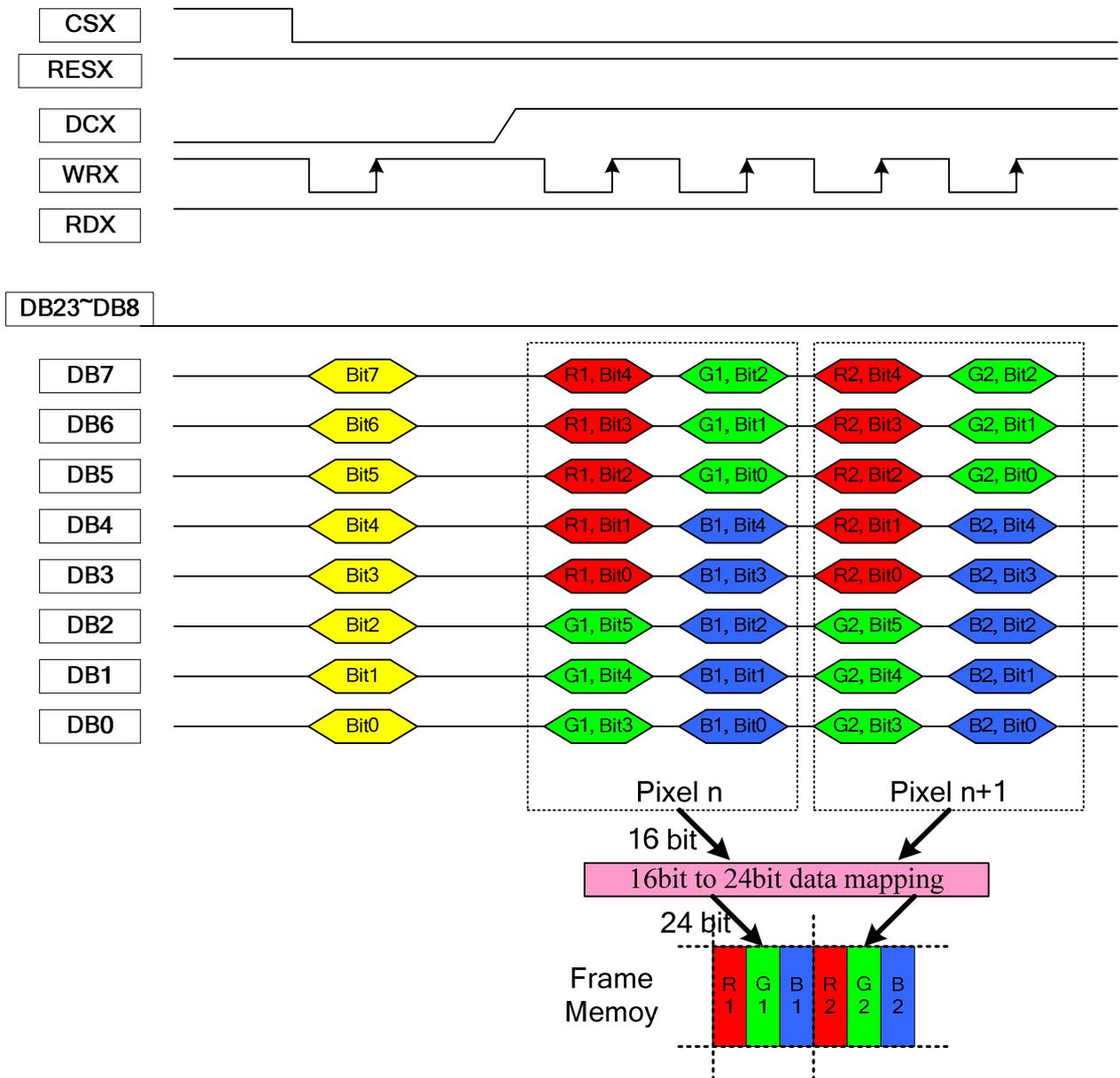
**Figure 135: 8-bit Data Bus for 16-bit/pixel (RGB 5-6-5 bits input), 65K-color**
