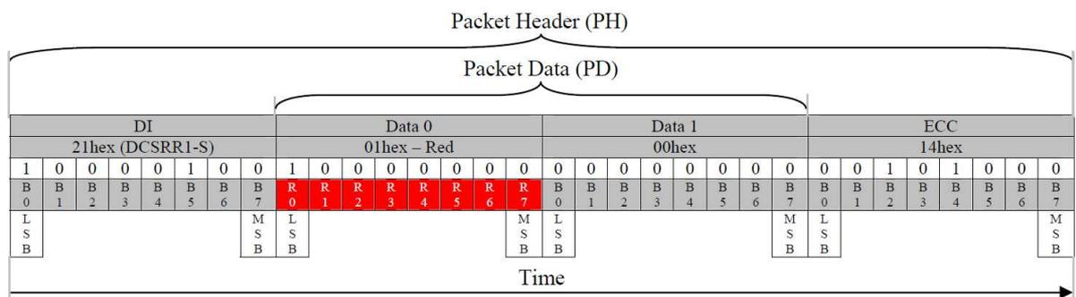
**Figure 111: Red Subpixel Response (DCSRR1-S) – Example 2**
