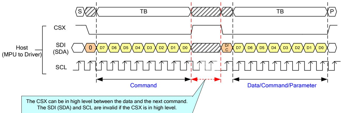
**Figure 18: DBI Type C Data Transfer Pause**
