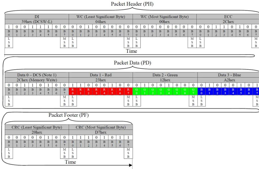
**Figure 105: One Pixel Write (DCSW-L) – Example <sup>Note</sup>**
