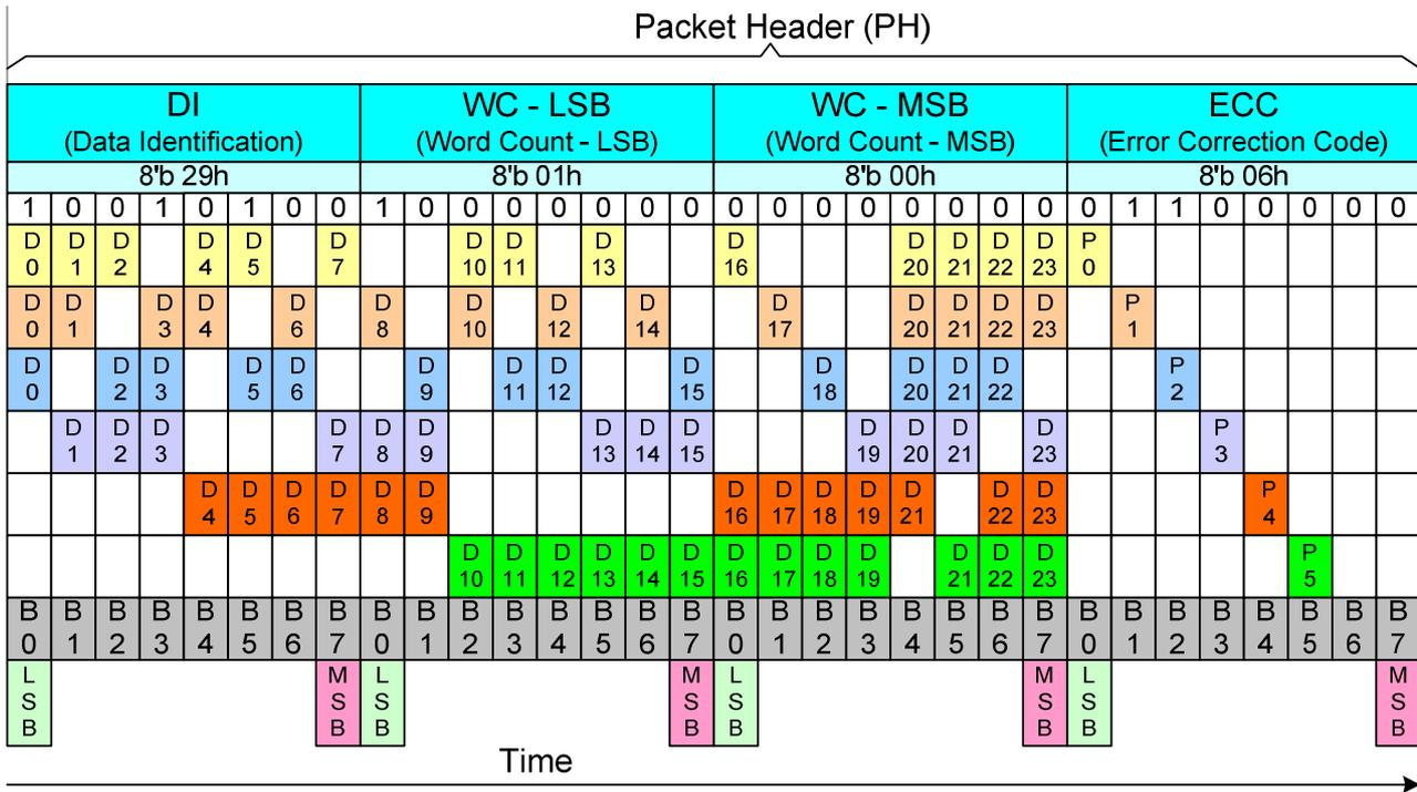
**Figure 73: XOR Functionality in a Long Packet (LPa)**
