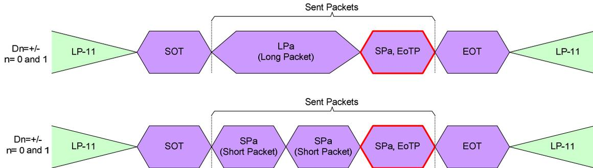
**Figure 90: End of Transmission Packet (EoTP) - Examples**
