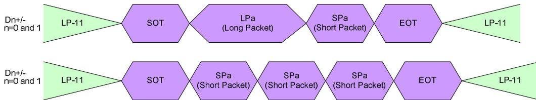
**Figure 45: Multiple Packets in High-Speed Data Transmission – Examples**
