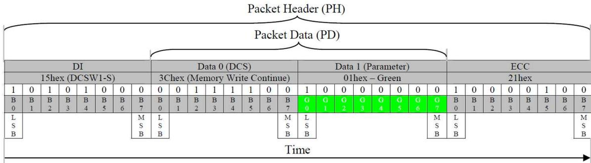
**Figure 107: Green Subpixel Write (DCSW1-S) – Example 3**
