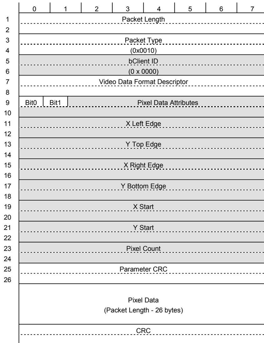
**Figure 120: Example of Video Stream Packet Fields**<sup>Note</sup>
