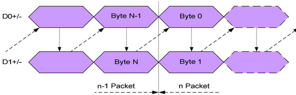
**Figure 50: Continuous Multiple Packets in HSDT when Number of Bytes is Equal on Both Data Lanes at the End of the Packet**
