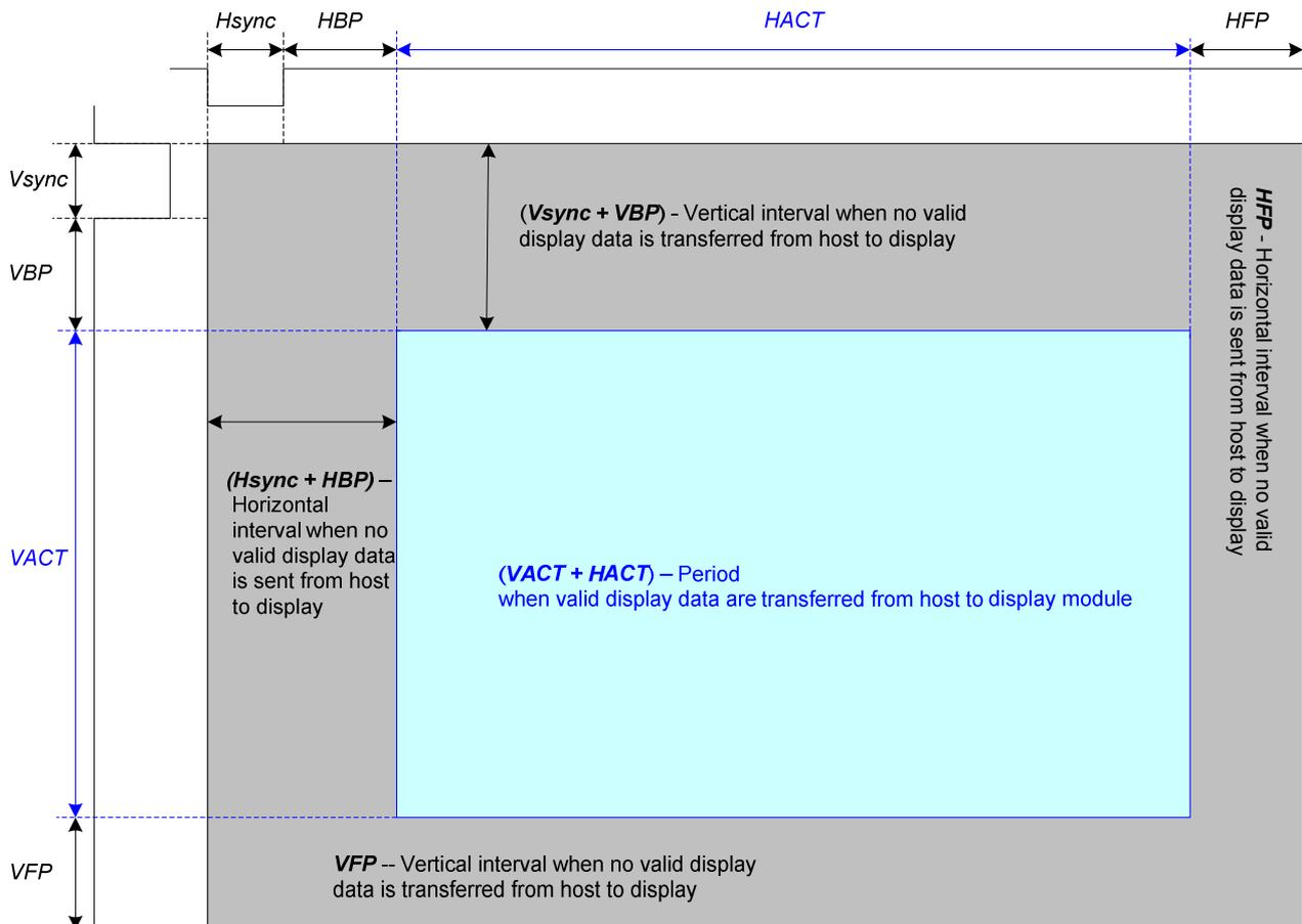
**Figure 23: General DPI Timing Diagram**
