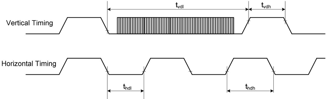
AC characteristics of the Tearing Effect Signal is: (Resolution 480(RGB)x800, Frame Rate = 60.5 Hz)
