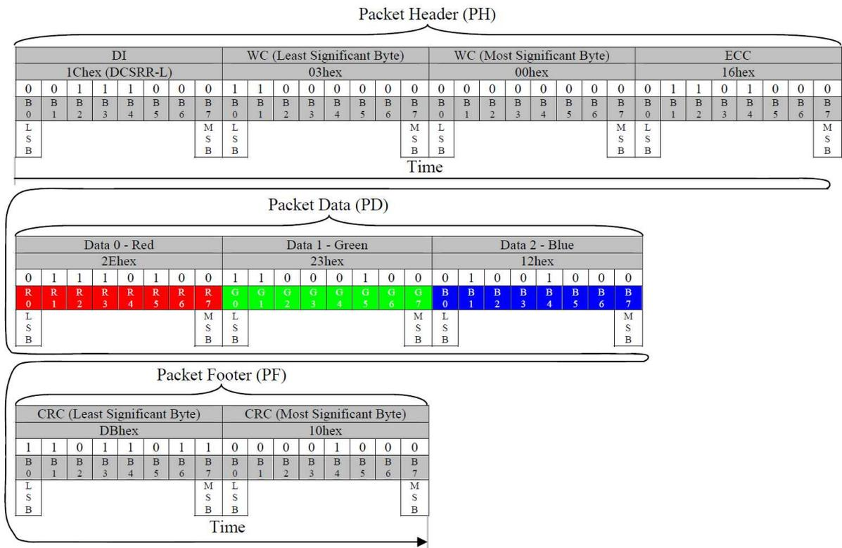
**Figure 110: One Pixel Read Response (DCSRR-L) – Example 1**
