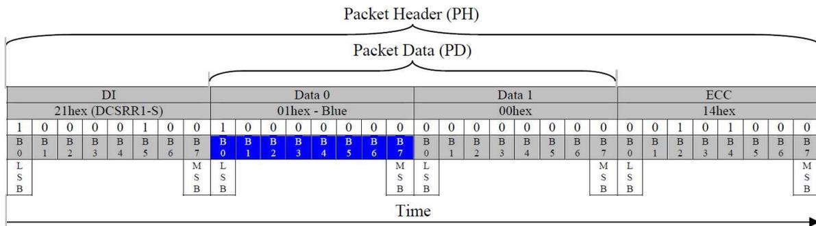
**Figure 113: Blue Subpixel Response (DCSRR1-S) – Example 4**
