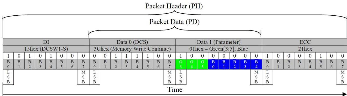
Figure 103: Green [3:5]/Blue Subpixel Write (DCSW1-S) – Example 3<sup>Note 2</sup>
