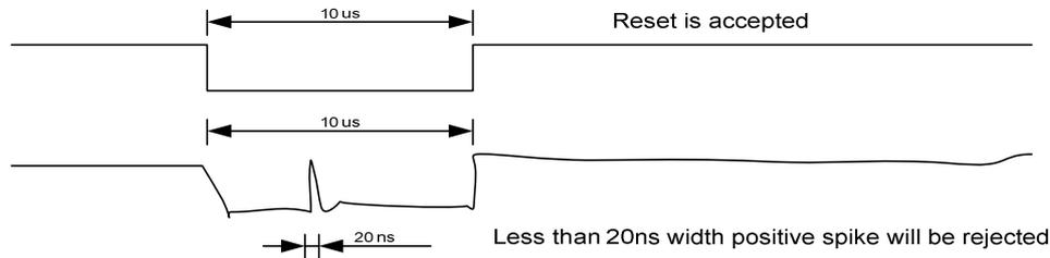
**Figure 183: Positive Noise Pulse during Reset Low**
