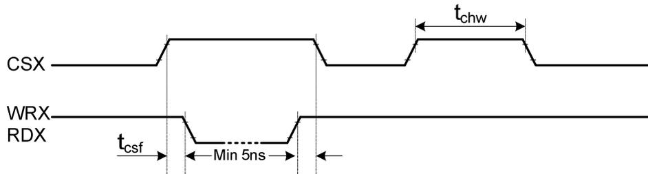
5. The Write-to-Read or the Read-to-Write timing:
