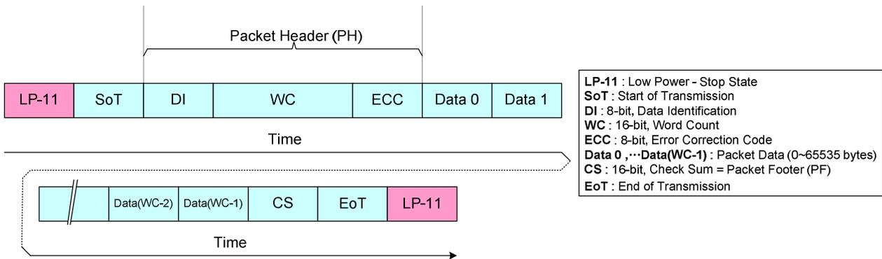
**Figure 56: Long Packet (LPa) Structure**
