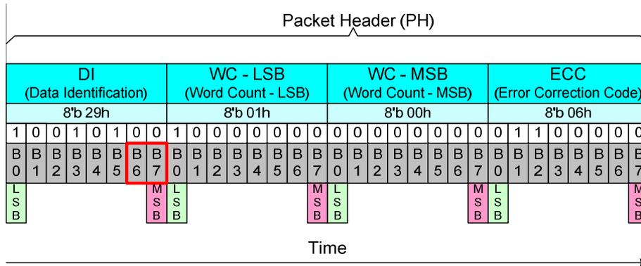
**Figure 63: Virtual Channel (VC) on the Packet Header (PH)**
