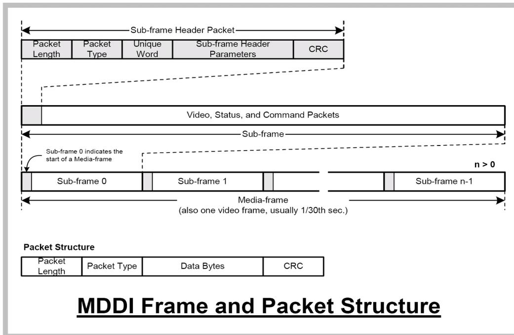
**Figure 118: Forward Link Structure**
