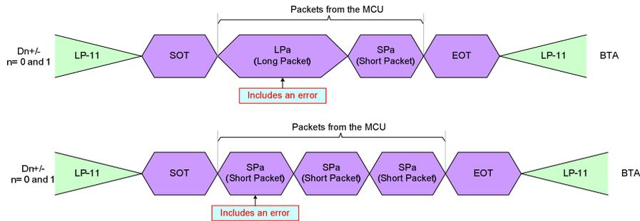
**Figure 95: Errors Packets**
