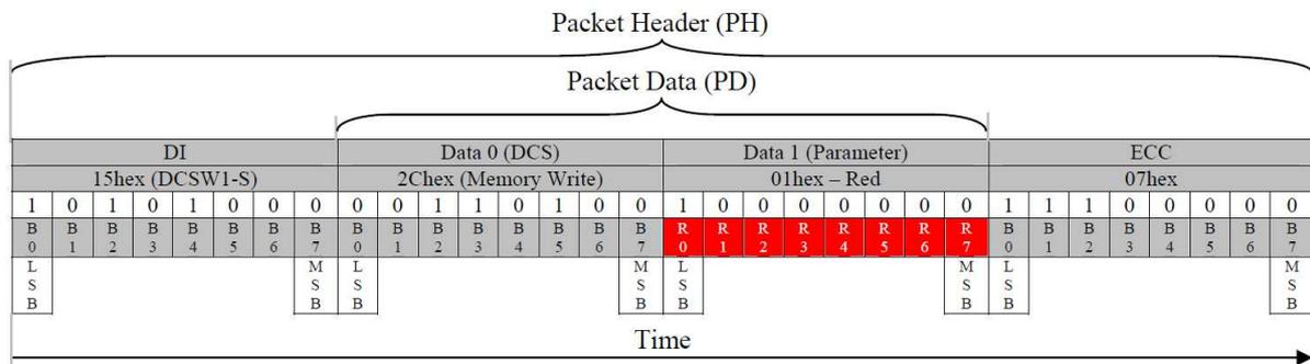
**Figure 108: Red Subpixel Write (DCSW1-S) – Example 4**
