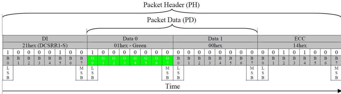
**Figure 112: Green Subpixel Response (DCSRR1-S) – Example 3**
