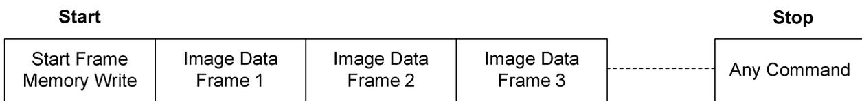
**Figure 20: Data Transfer Mode - Method 1**
