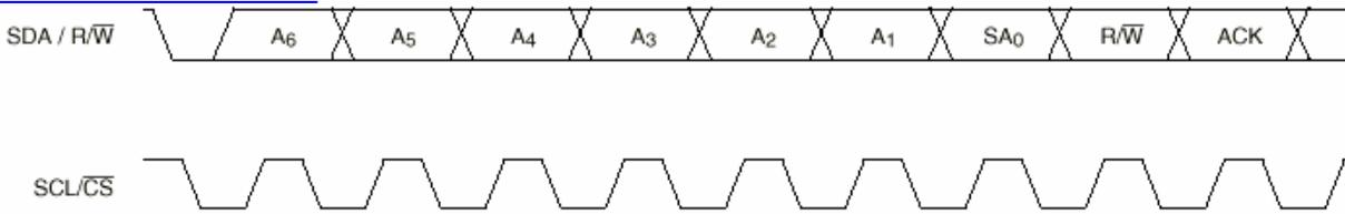
Figure 18. 7-bit Slave Address with Read/Write Bit
