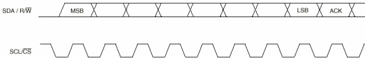
Figure 17. Serial Interface – Typical Byte Transfer
