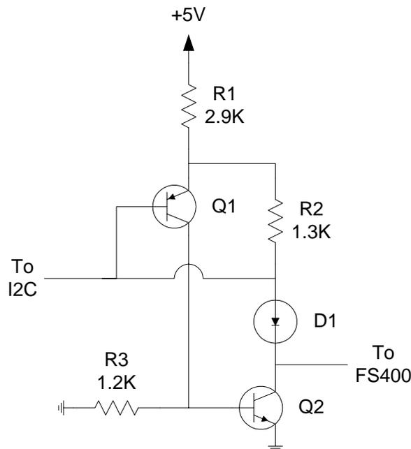
**Figure 26. SIO Translation Using Current Mirrors**
