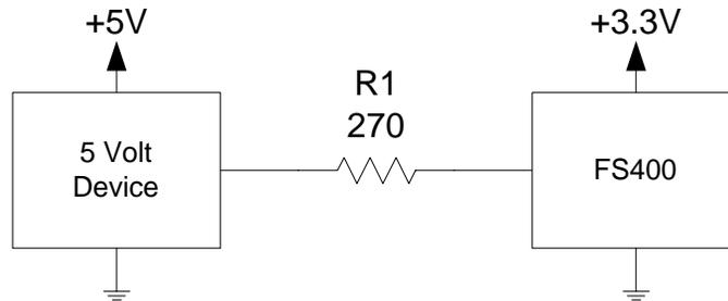
Figure 23. 5 to 3.3 Volt Translation using a Resistor
