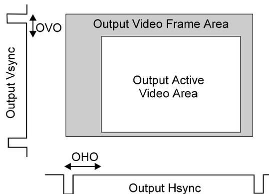
**Figure 13. Output Horizontal and Vertical Offset Definitions**
