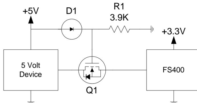
Figure 24. 5 to 3.3 Volt Translation using a MOSFET
