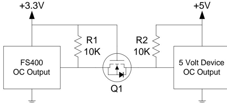
**Figure 27. SIO (Open Collector) Translation using a MOSFET**
