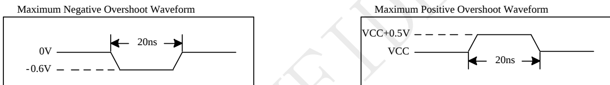
Figure 5-2 Input Test Waveforms and Measurement Level
