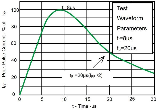
Fig 1. Pulse Waveform
