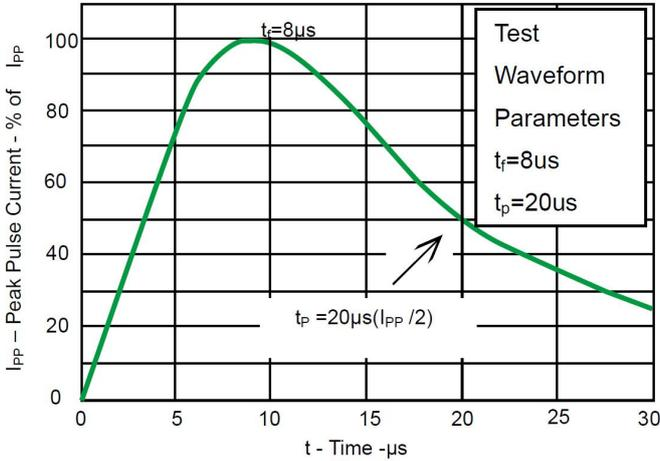
Fig 1. Pulse Waveform
