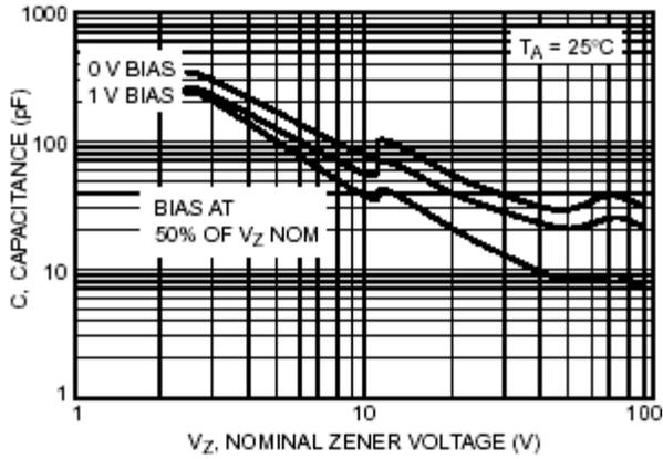
Figure 7. Typical Capacitance
