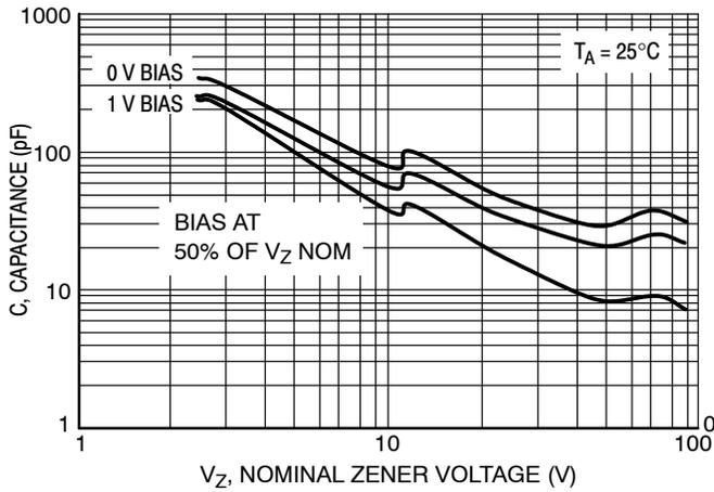
Figure 5. Typical Capacitance
