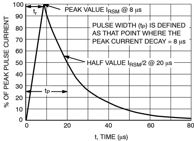
Figure 9.  $8 \times 20 \mu\text{s}$  Pulse Waveform
