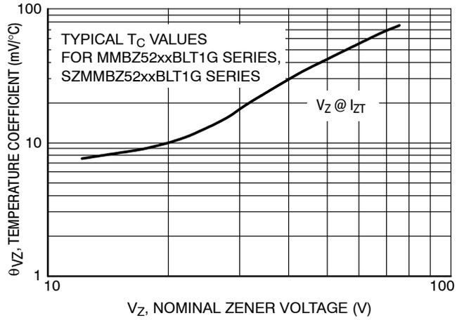
**Figure 2. Temperature Coefficients**
