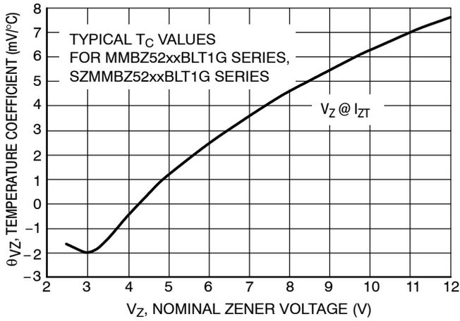
**Figure 1. Temperature Coefficients**
