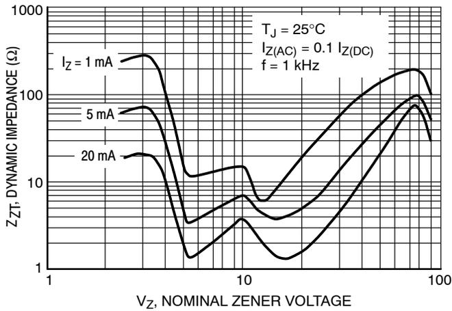
**Figure 3. Effect of Zener Voltage on Zener Impedance**
