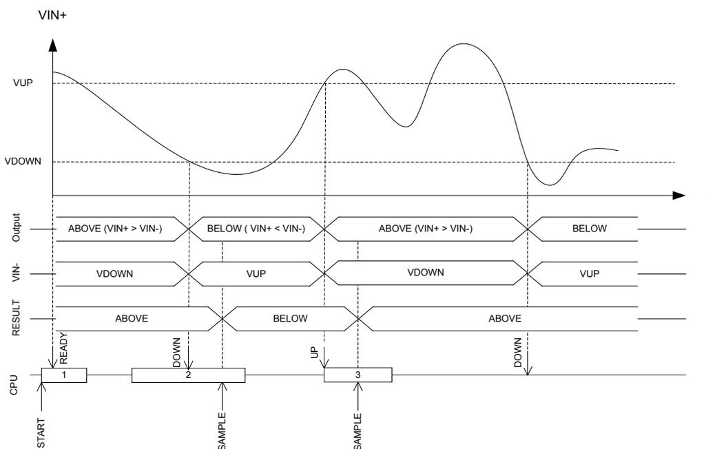
Figure 38: Hysteresis example where  $VIN+$  starts above  $VUP$
