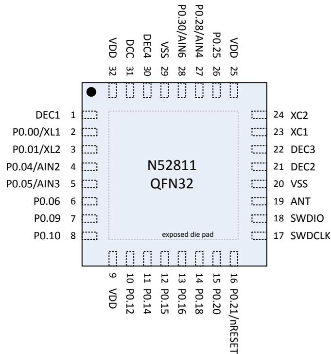
Figure 152: QFN32 pin assignments, top view
