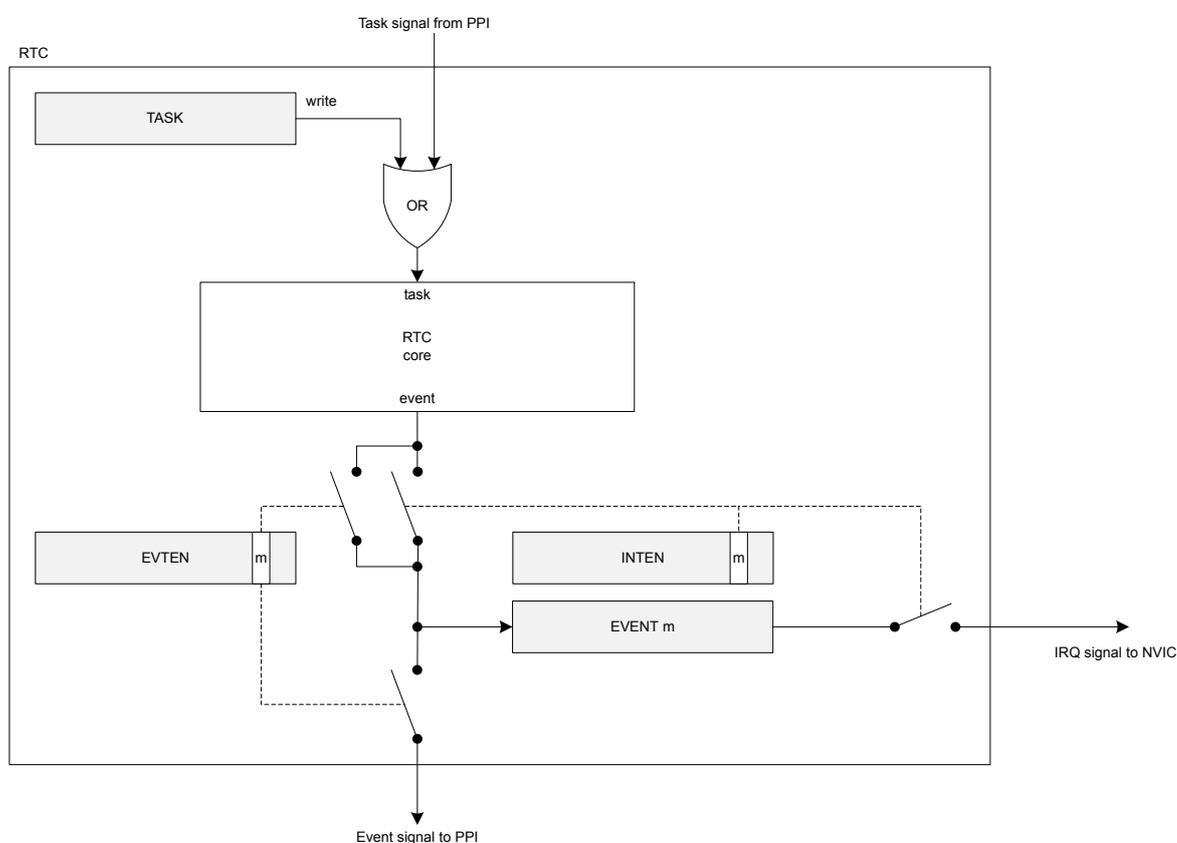
Figure 92: Tasks, events and interrupts in the RTC
