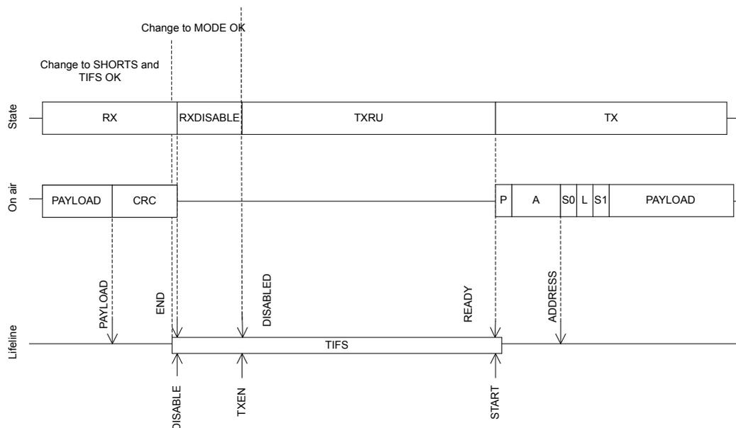
Figure 69: IFS timing detail
