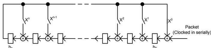
Figure 61: CRC generation of an  $n$  bit CRC
