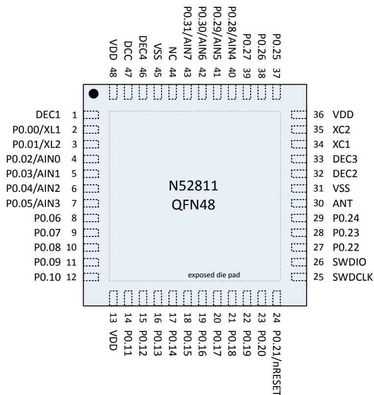
Figure 151: QFN48 pin assignments, top view
