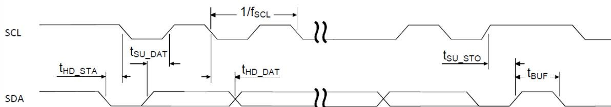
Figure 135: TWIM timing diagram, 1 byte transaction
