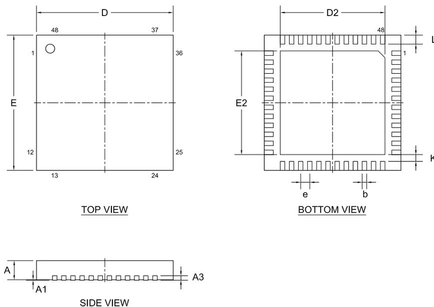
Figure 154: QFN48 6 x 6 mm package
