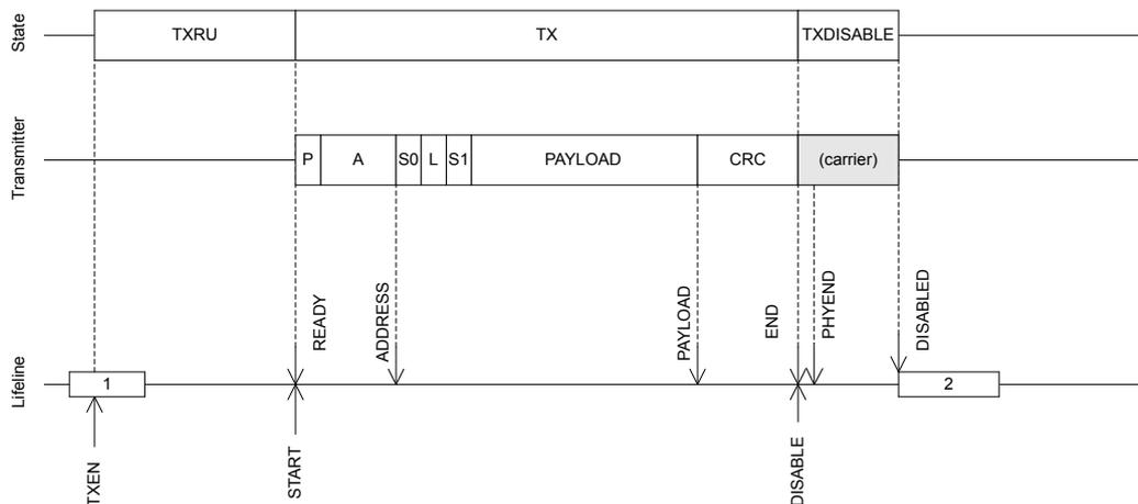
Figure 64: Transmit sequence using shortcuts to avoid delays
