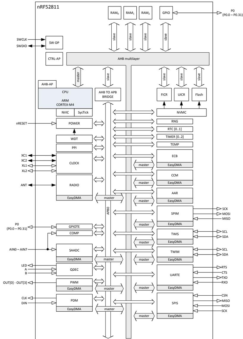
Figure 1: Block diagram
