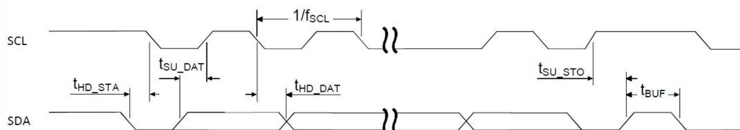
Figure 143: TWIS timing diagram, 1 byte transaction
