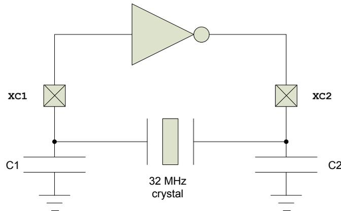
Figure 18: Circuit diagram of the 64 MHz crystal oscillator
