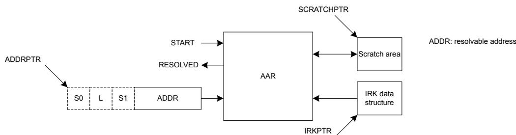
Figure 23: Address resolution with packet preloaded into RAM
