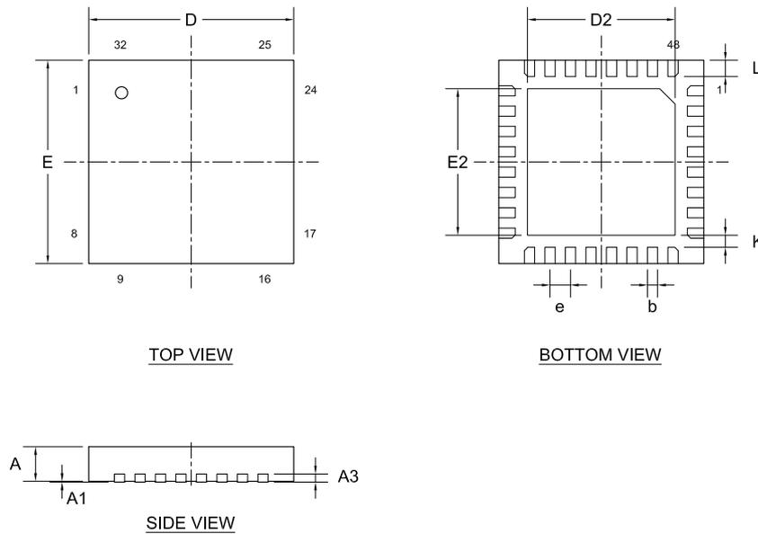
Figure 155: QFN32 5 x 5 mm package
