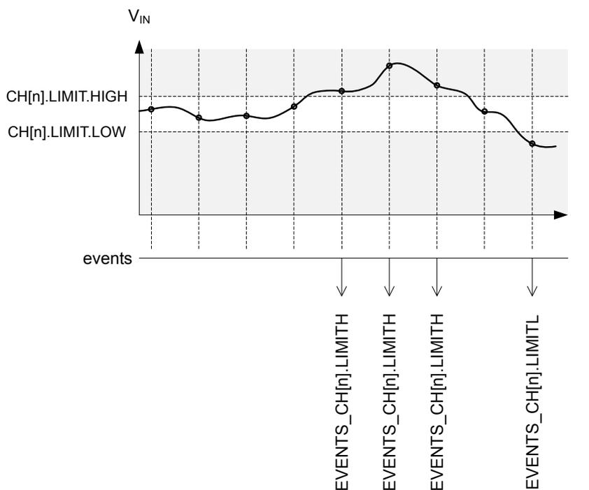
Figure 110: Example of limits monitoring on channel 'n'
