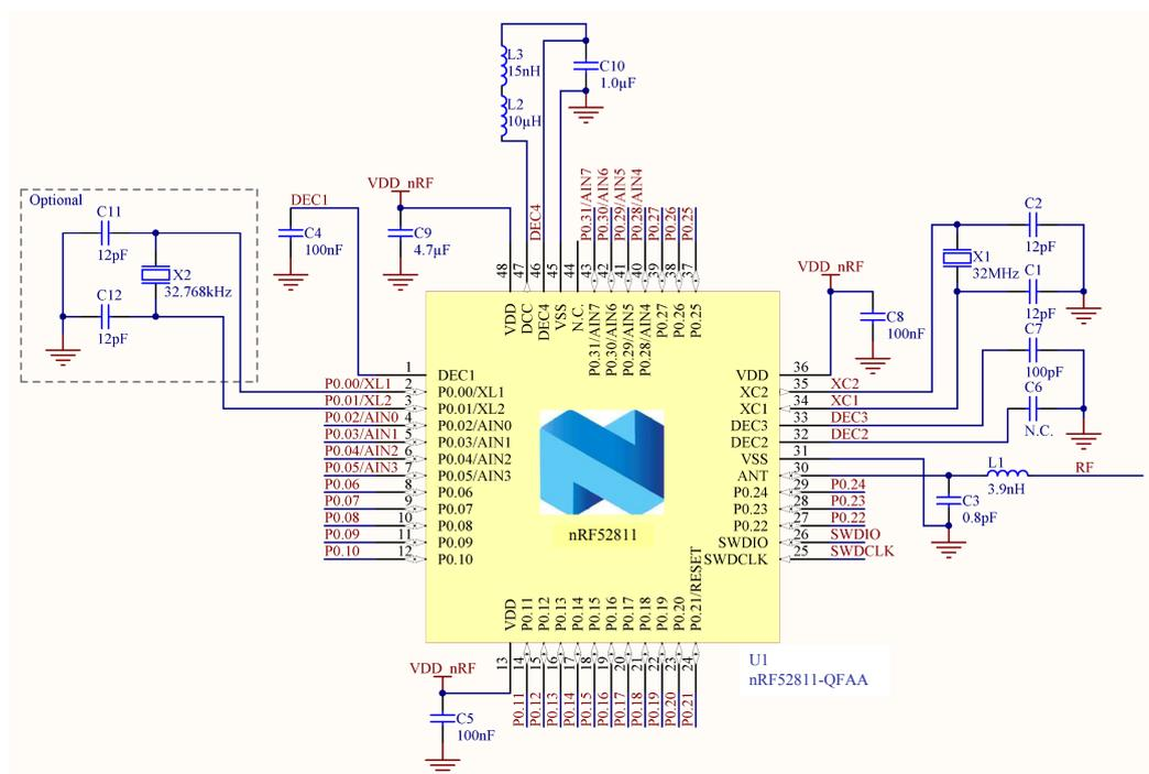
Figure 158: QFAA QFN48 with DC/DC regulator setup
