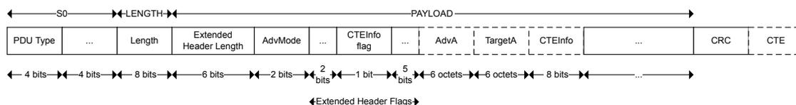
Figure 73: Advertising channel PDU header
