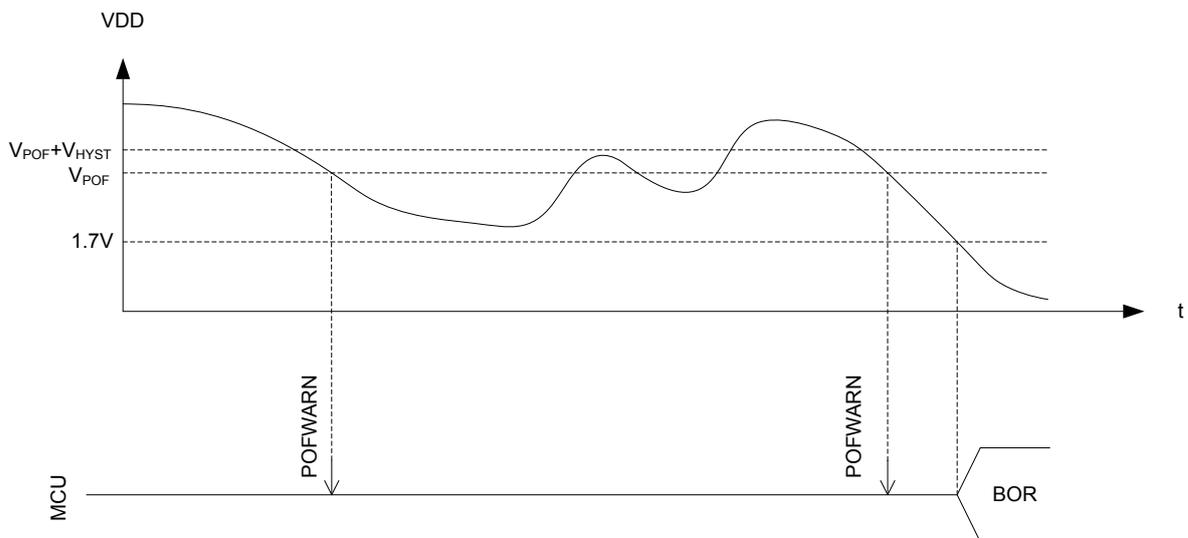
Figure 16: Power-fail comparator (BOR = Brownout reset)
