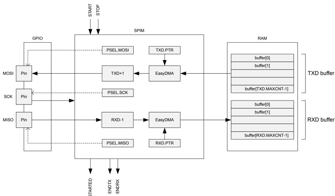
Figure 115: SPIM — SPI master with EasyDMA
