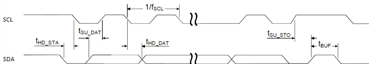
Figure 127: TWI timing diagram, 1 byte transaction
