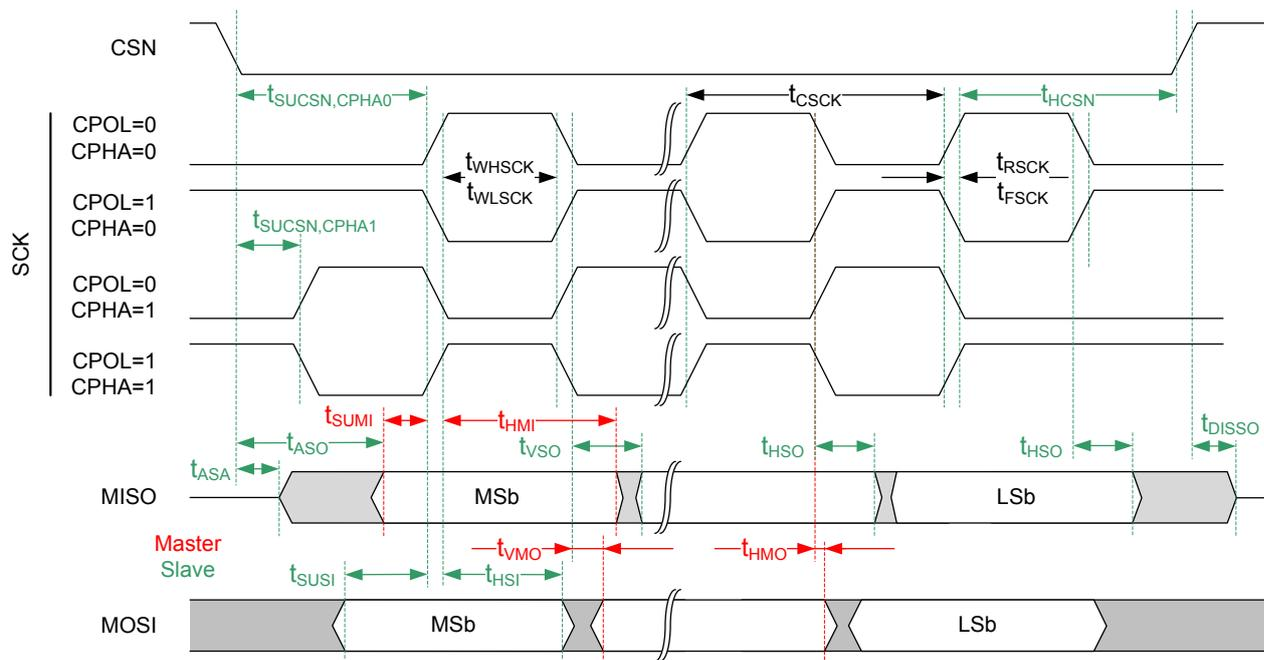
Figure 121: Common SPIM and SPIS timing diagram
