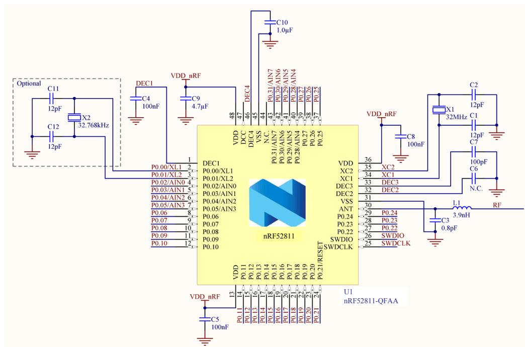
Figure 157: QFAA QFN48 with internal LDO regulator setup
