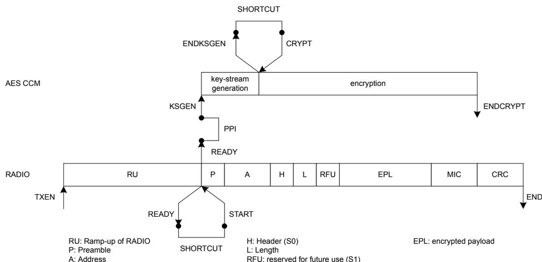
Figure 30: On-the-fly encryption of short packets (MODE.LENGTH = Default) using a PPI connection
