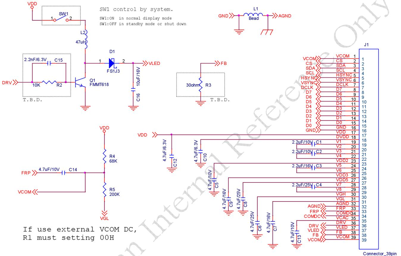
Note1: Use internal LED driver must set R5[1](SHDB1)= "1".
