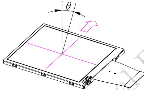
Note 8. Measured at the center area of the panel when all the input terminals of LCD panel are electrically opened with LED driving current = 25mA.
