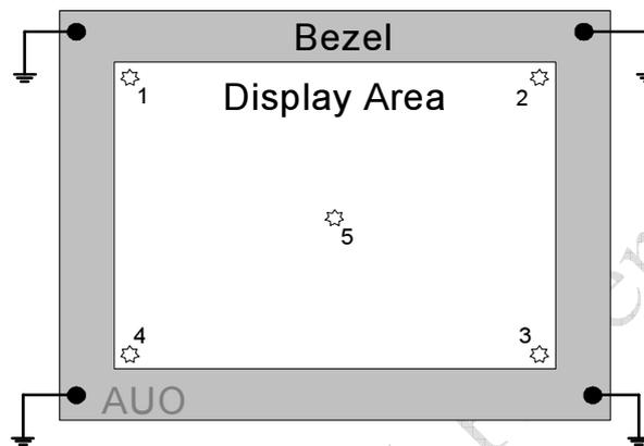
7. The metal casing is connected to ground (0V) at four corners.
