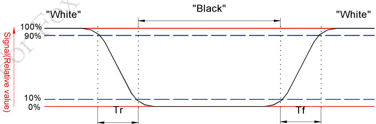
The response time is defined as the time interval between the 10% and 90% of amplitudes. Refer to figure as below.
