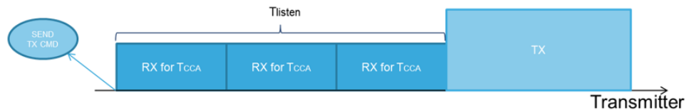
Figure 23. CSMA if channel is free (timeline)
