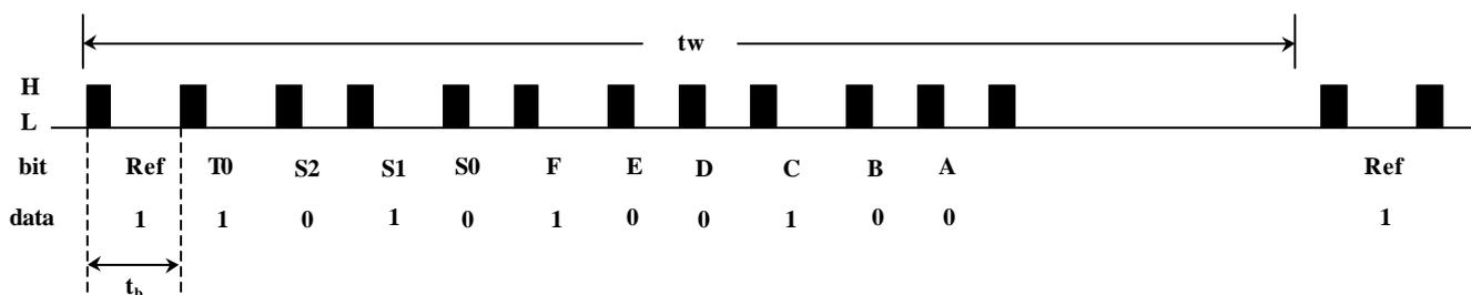
Modulated pulse 【  $t_{pw} = (5 \times t_M) + t_{MH}$  】
