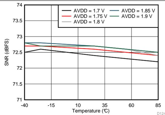
Figure 123. Signal-to-Noise Ratio vs AVDD Supply and Temperature (170 MHz)
