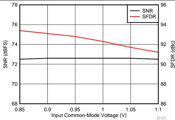
Figure 120. Performance vs Input Common-Mode Voltage (30 MHz)
