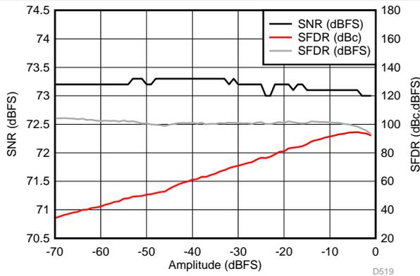
Figure 52. Performance vs Input Amplitude (30 MHz)
