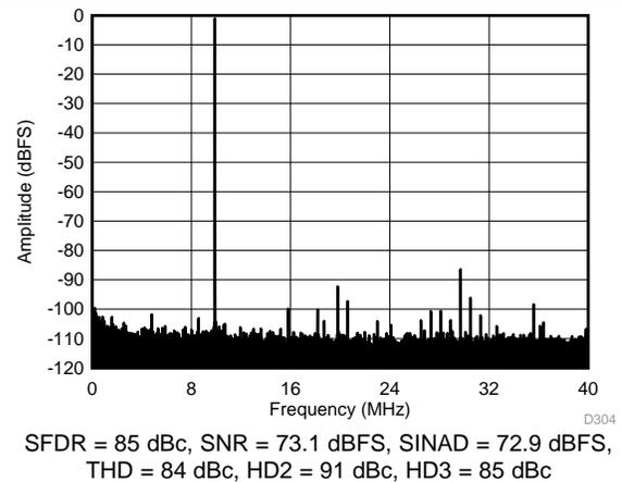
**Figure 70. FFT for 70-MHz Input Signal (Dither Off)**
