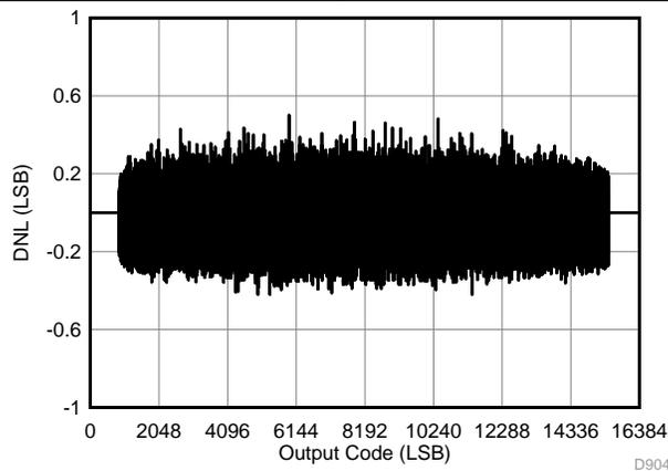
Figure 66. Differential Nonlinearity for 20-MHz Input
