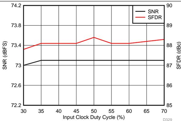
Figure 95. Performance vs Clock Duty cycle (30 MHz)
