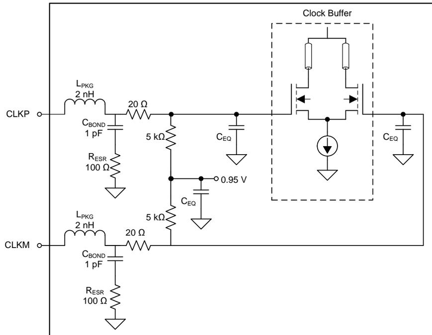
NOTE:  $C_{EQ}$  is 1 pF to 3 pF and is the equivalent input capacitance of the clock buffer.
