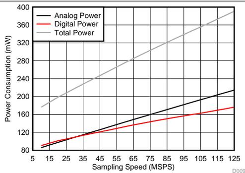
Figure 137. Power vs Sampling Frequency (Two-Wire Mode)
