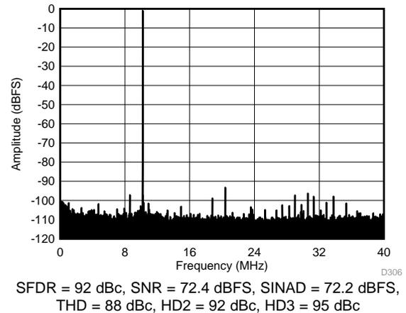
**Figure 72. FFT for 170-MHz Input Signal (Dither Off)**
