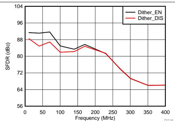
Figure 18. Spurious-Free Dynamic Range vs Input Frequency
