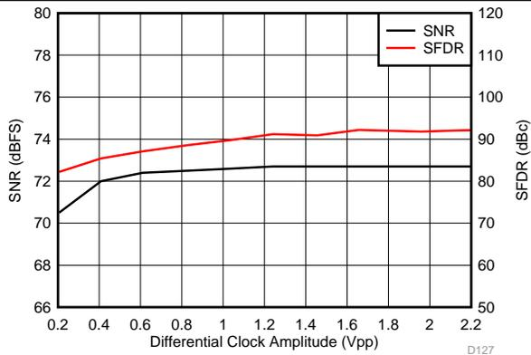
Figure 126. Performance vs Clock Amplitude (40 MHz)
