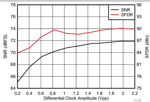
Figure 94. Performance vs Clock Amplitude (150 MHz)
