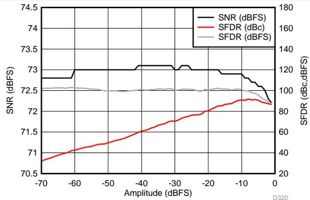
Figure 86. Performance vs Input Amplitude (170 MHz)
