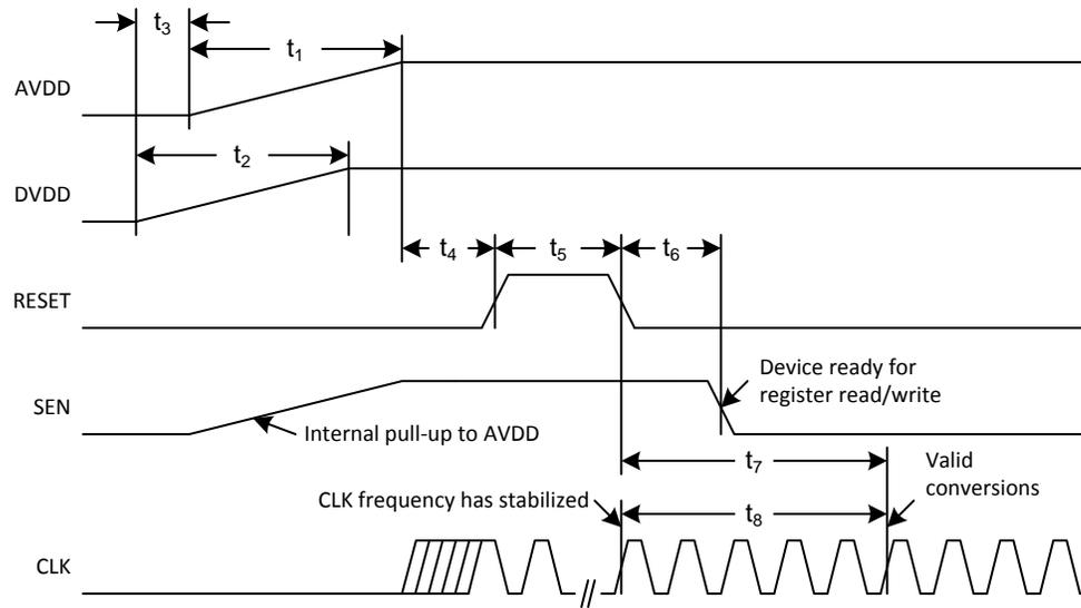
**Figure 160. Power-Up Timing**
