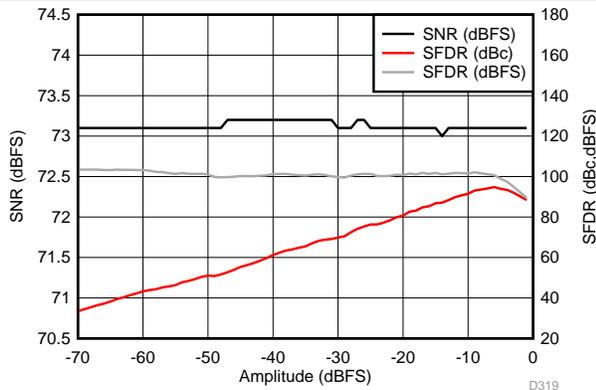
Figure 85. Performance vs Input Amplitude (30 MHz)
