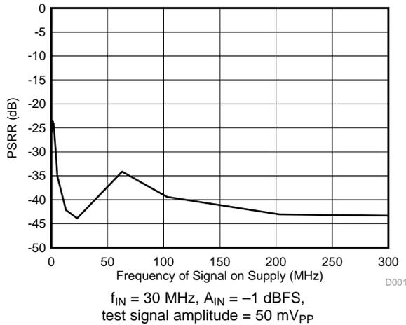
Figure 133. Power-Supply Rejection Ratio vs Test Signal Frequency
