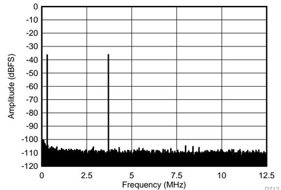
$f_{IN1} = 46.3 \text{ MHz}$ ,  $f_{IN2} = 50.3 \text{ MHz}$ , IMD3 = 105 dBFS,
