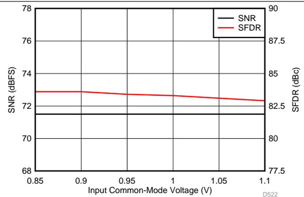
Figure 55. Performance vs Input Common-Mode Voltage (170 MHz)
