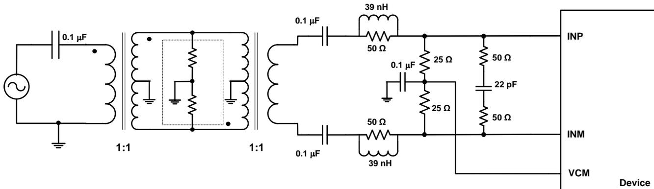
Figure 197. Driving Circuit for Low Input Frequencies
