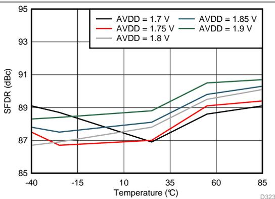
Figure 89. Spurious-Free Dynamic Range vs AVDD Supply and Temperature (170 MHz)
