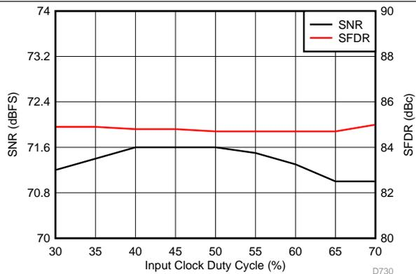
Figure 30. Performance vs Clock Duty Cycle (150 MHz)
