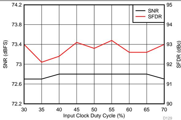
Figure 128. Performance vs Clock Duty Cycle (30 MHz)
