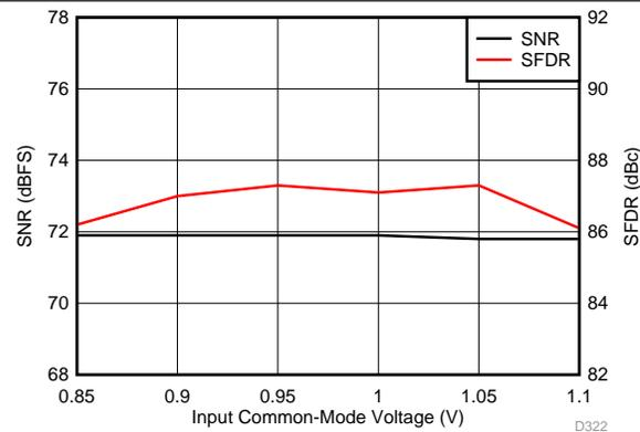
Figure 88. Performance vs Input Common-Mode Voltage (170 MHz)
