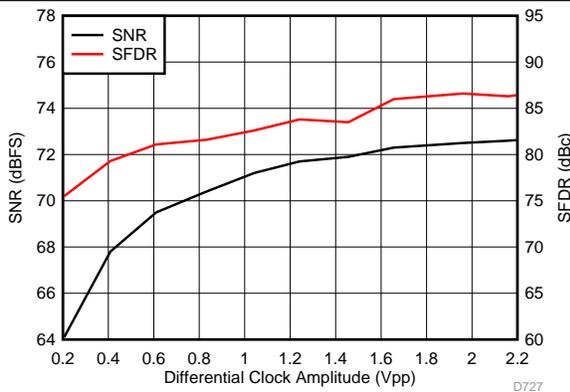
Figure 27. Performance vs Clock Amplitude (40 MHz)
