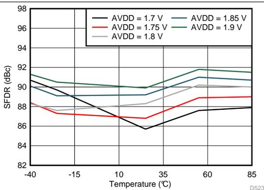
Figure 56. Spurious-Free Dynamic Range vs AVDD Supply and Temperature (30 MHz)
