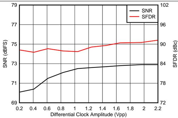
Figure 60. Performance vs Clock Amplitude (40 MHz)
