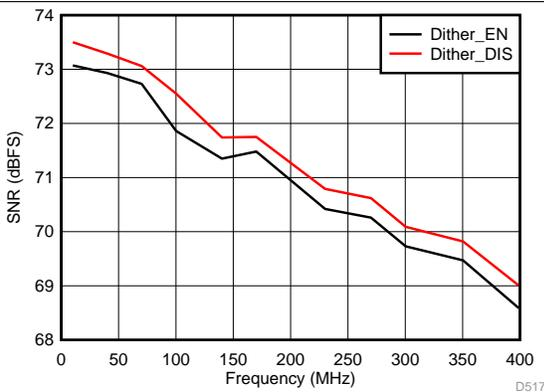
Figure 50. Signal-to-Noise Ratio vs Input Frequency
