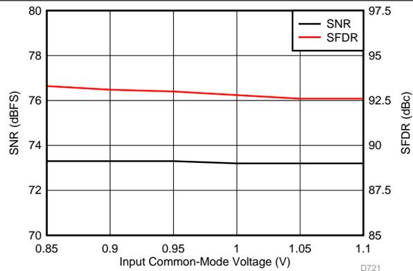
Figure 21. Performance vs Input Common-Mode Voltage (30 MHz)
