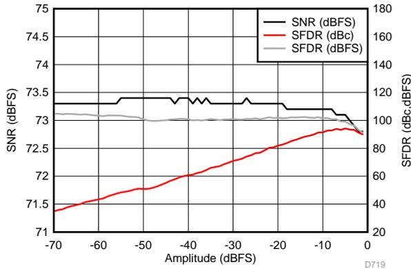
Figure 19. Performance vs Input Amplitude (30 MHz)
