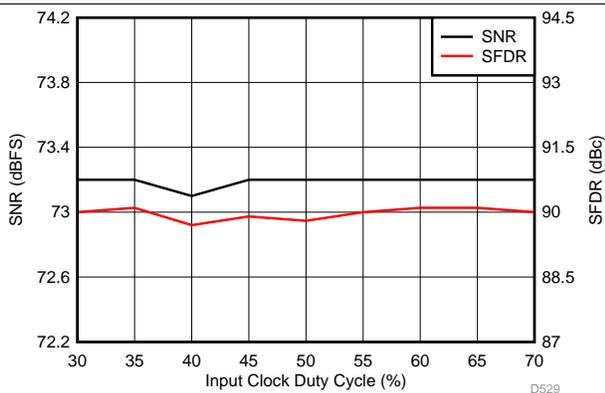
Figure 62. Performance vs Clock Duty Cycle (30 MHz)
