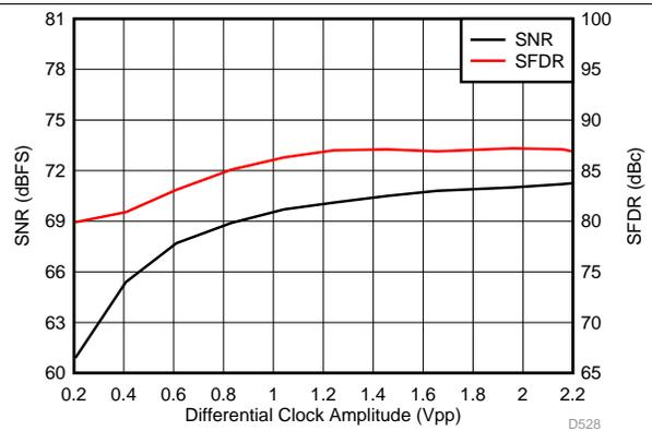
Figure 61. Performance vs Clock Amplitude (150 MHz)
