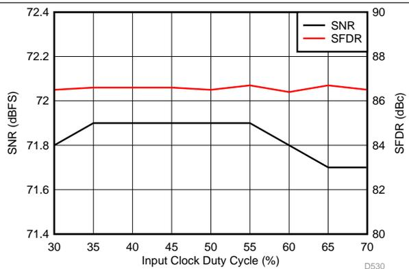
Figure 63. Performance vs Clock Duty Cycle (150 MHz)
