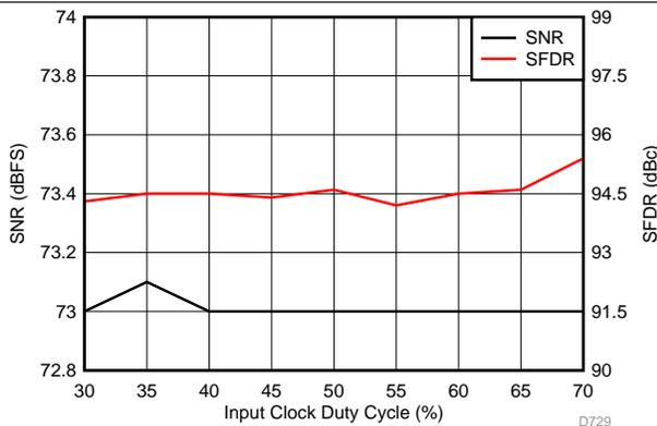
Figure 29. Performance vs Clock Duty Cycle (30 MHz)
