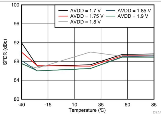
Figure 23. Spurious-Free Dynamic Range vs AVDD Supply and Temperature (30 MHz)
