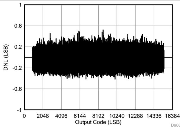
Figure 99. Differential Nonlinearity for 70-MHz Input
