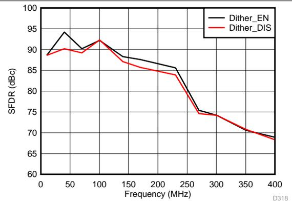
Figure 84. Spurious-Free Dynamic Range vs Input Frequency
