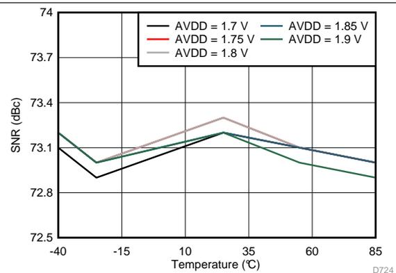
Figure 24. Signal-to-Noise Ratio vs AVDD Supply and Temperature (30 MHz)
