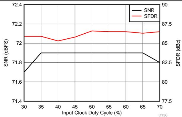
Figure 129. Performance vs Clock Duty Cycle (150 MHz)
