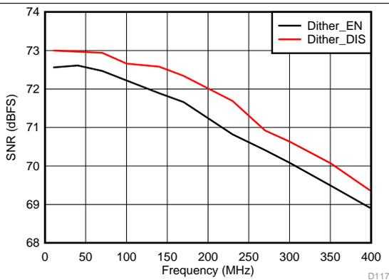
Figure 116. Signal-to-Noise Ratio vs Input Frequency
