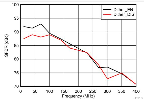
Figure 117. Spurious-Free Dynamic Range vs Input Frequency
