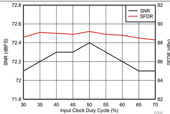
Figure 96. Performance vs Clock Duty Cycle (150 MHz)
