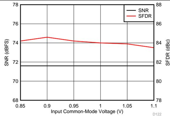
Figure 121. Performance vs Input Common-Mode Voltage (170 MHz)
