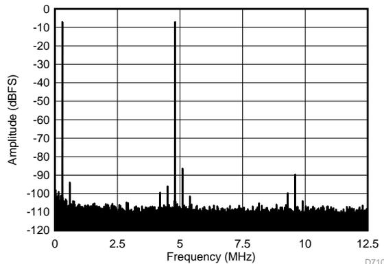
$f_{IN1} = 46.3 \text{ MHz}$ ,  $f_{IN2} = 50.3 \text{ MHz}$ , IMD3 = 86 dBFS,
