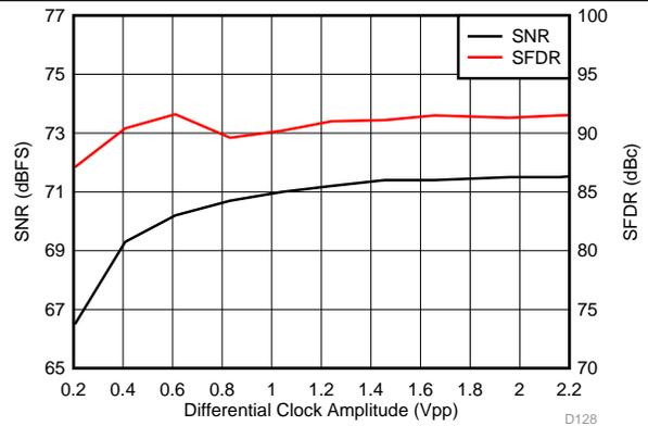
Figure 127. Performance vs Clock Amplitude (150 MHz)
