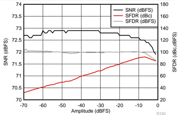
Figure 119. Performance vs Input Amplitude (170 MHz)
