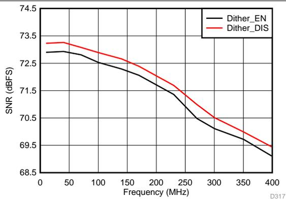
Figure 83. Signal-to-Noise Ratio vs Input Frequency
