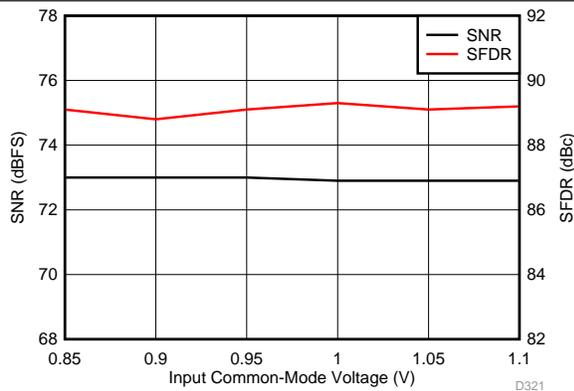
Figure 87. Performance vs Input Common-Mode Voltage (30 MHz)
