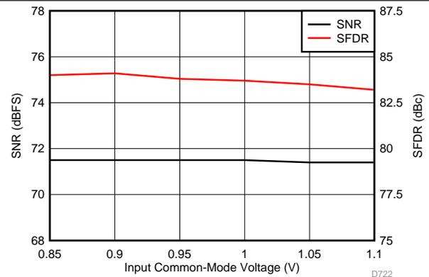
Figure 22. Performance vs Input Common-Mode Voltage (170 MHz)
