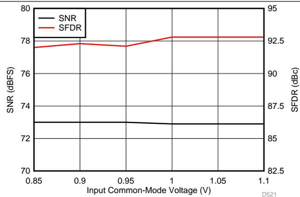
Figure 54. Performance vs Input Common-Mode Voltage (30 MHz)
