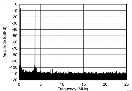
$f_{IN1} = 46.3 \text{ MHz}$ ,  $f_{IN2} = 50.3 \text{ MHz}$ , IMD3 = 102 dBFS,
