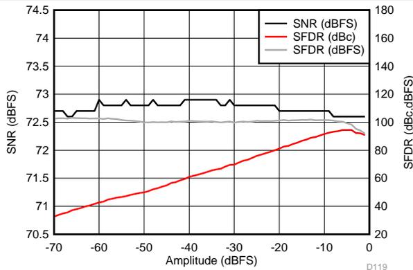
Figure 118. Performance vs Input Amplitude (30 MHz)
