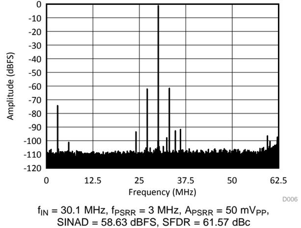
Figure 134. Power-Supply Rejection Ratio Spectrum (Chopper On)
