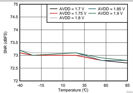
Figure 90. Signal-to-Noise Ratio vs AVDD Supply and Temperature (170 MHz)
