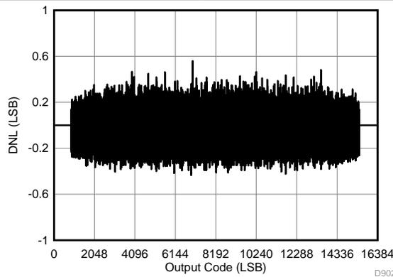
Figure 33. Differential Nonlinearity for 20-MHz Input
