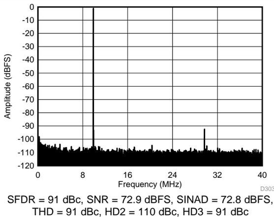
**Figure 69. FFT for 70-MHz Input Signal (Dither On)**
