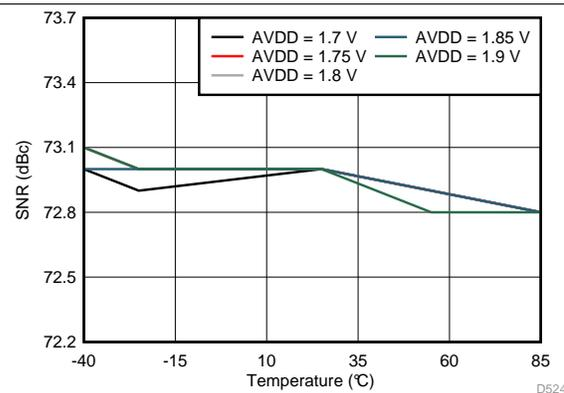
Figure 57. Signal-to-Noise Ratio vs AVDD Supply and Temperature (30 MHz)
