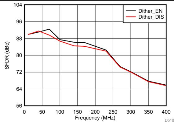
Figure 51. Spurious-Free Dynamic Range vs Input Frequency
