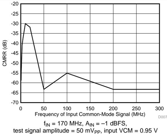
Figure 135. Common-Mode Rejection Ratio vs Test Signal Frequency
