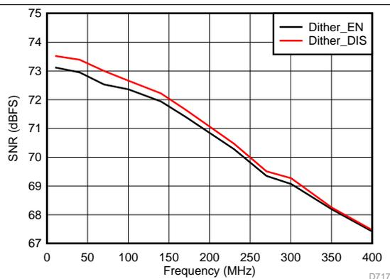
Figure 17. Signal-to-Noise Ratio vs Input Frequency
