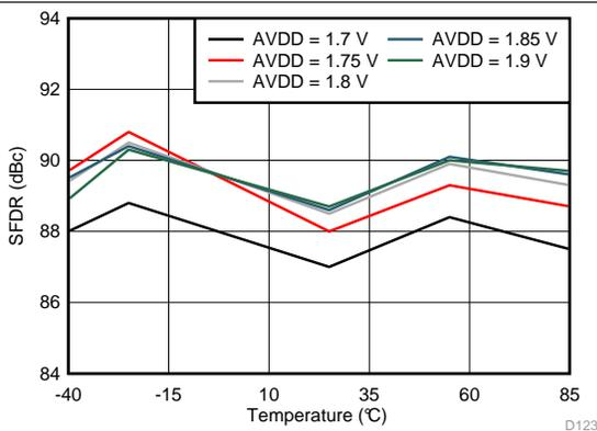
Figure 122. Spurious-Free Dynamic Range vs AVDD Supply and Temperature (170 MHz)
