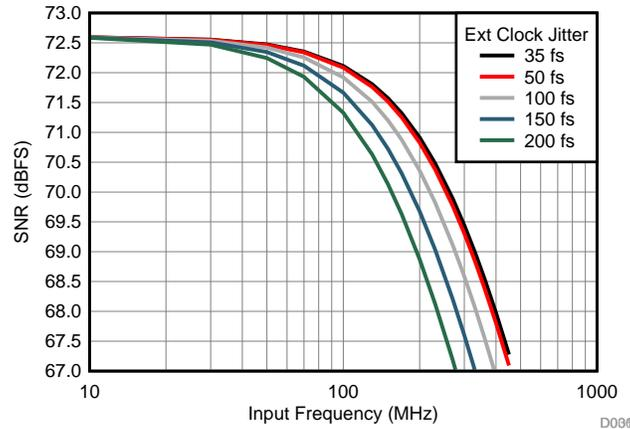
Figure 151. SNR vs Frequency for Different Clock Jitter
