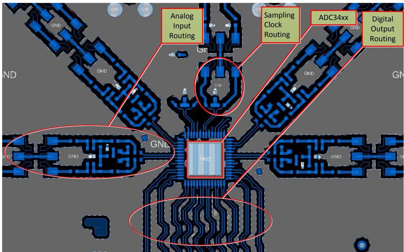
**Figure 203. Typical Layout of the ADC344x Board**
