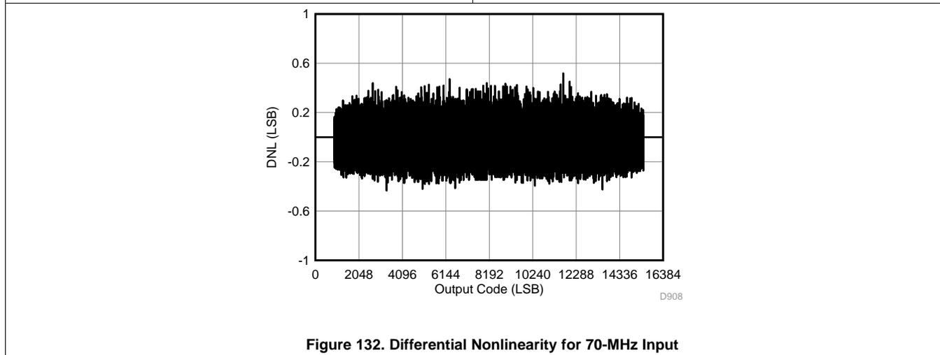
Figure 132. Differential Nonlinearity for 70-MHz Input
