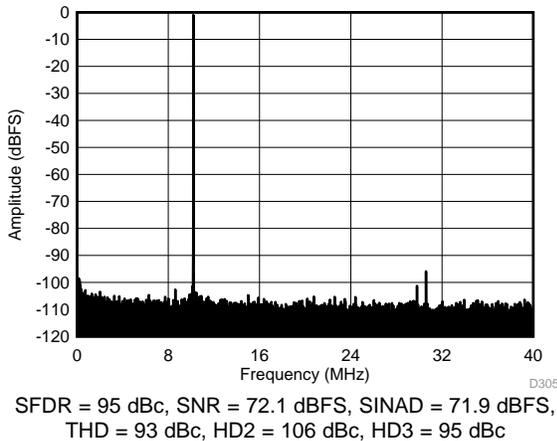
**Figure 71. FFT for 170-MHz Input Signal (Dither On)**
