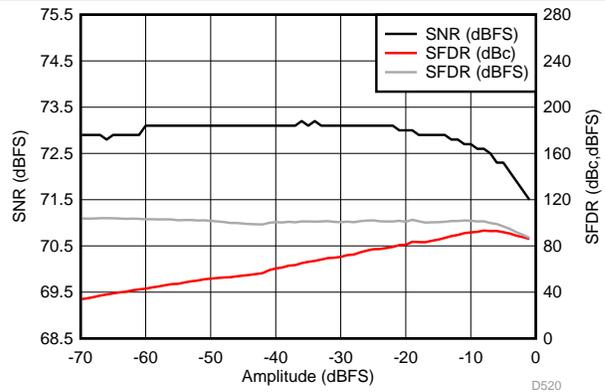
Figure 53. Performance vs Input Amplitude (170 MHz)
