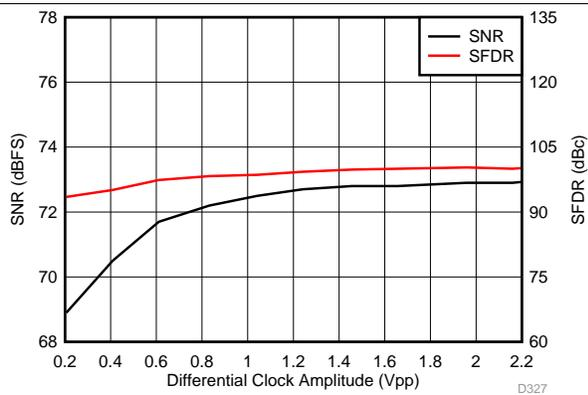
Figure 93. Performance vs Clock Amplitude (40 MHz)
