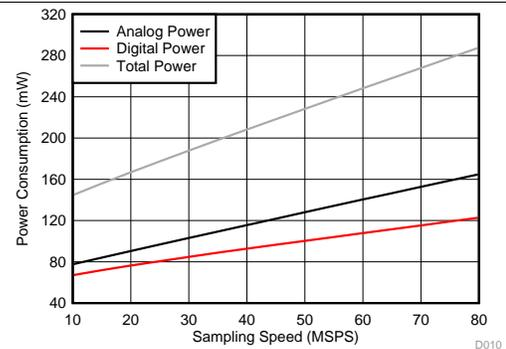
Figure 138. Power vs Sampling Frequency (One-Wire Mode)
