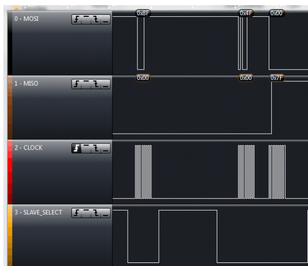
Figure 6-26. Reset FIFO and Read RSSI
