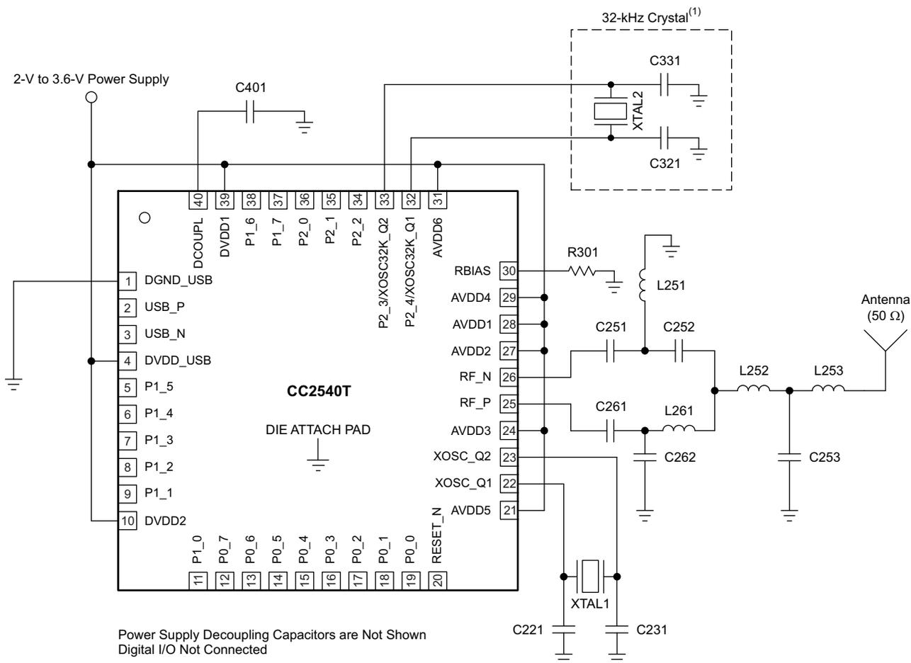
(1) 32-kHz crystal is mandatory when running the chip in low-power modes, except if the link layer is in the standby state (Vol. 6 Part B Section 1.1, see [1]).
