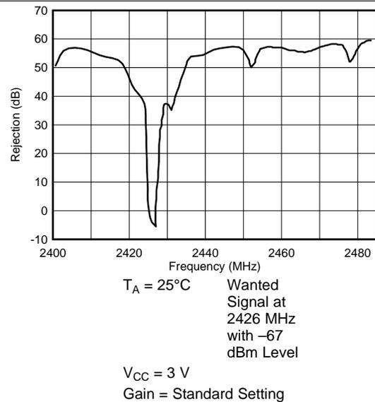
Figure 4-16. RX Interferer Rejection (Selectivity) vs Interferer Frequency
